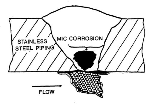
Figure 5-1. Closed Pit, Typical of MIC in Stainless Steel Piping Welds (from [7])
