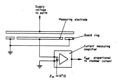
Figure 5. Operating circuit
