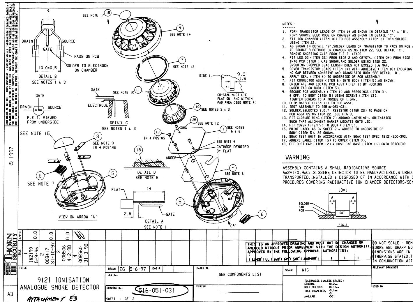
AS SHOWN IN DETAIL 'B', SOLDER LEADS OF TRANSISTOR TO PADS ON PCB AND FIT LED.D3 (ITEM 23) FROM SIDE 2 AND CRYSTAL (ITEM 24) FROM SIDE 1 ENSURING CROPPED LEAD LENGTH DOES NOT EXCEED 1.6 MAX. COVER TRANSISTOR LEADS (ITEM 14) WITH ADHESIVE (ITEM 18) ENSURING NO GAP BETWEEN ADHESIVE AND TRANSISTOR BODY.SEE DETAIL 'D'.
