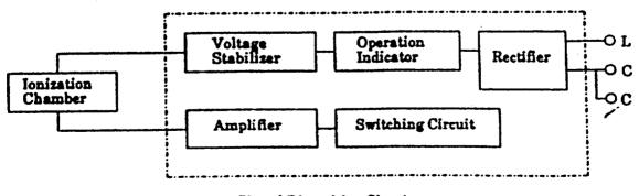
Signal Disposition Circuit
