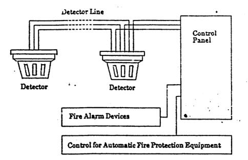
The control panel supplies the power to the detectors. The lines are also used as signal lines. Removal of any the detector head and the interruption of lines are supervised by the end-of-line device.
