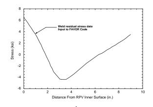
Figure 4-7 Through-thickness weld residual stress profile assumed by FAVOR [56]
