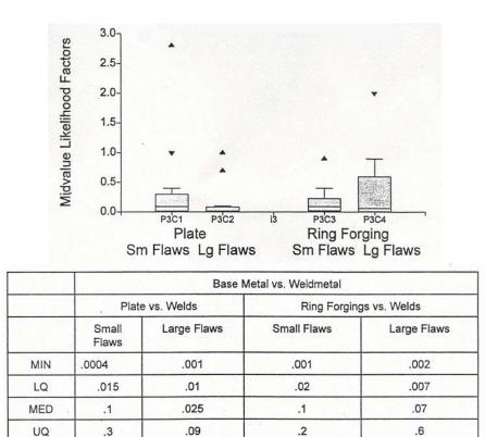
Figure 3 Relative Flaw Densities of Base Metal Compared to Weld Metal as Estimated by Expert Judgment Process (from Jackson and Abramson 2000)
