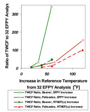
Figure 5-1 Effect of different methods to artificially increase embrittlement on the predicted TWCF values
