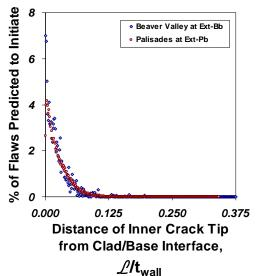
Figure 4-3 Distribution through-wall position of cracks that initiate
