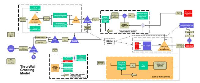
Figure 4-10 Model of through-wall cracking adopted by FAVOR
