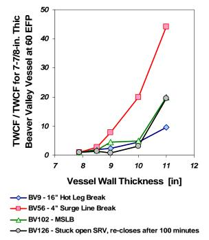
Figure 5-4 Effect of vessel wall thickness on the TWCF of various transients in Beaver Valley (all analyses at 60 EFPYs)
