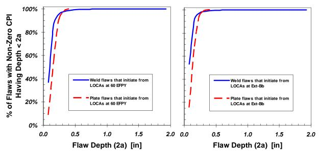
Figure 4-4 Flaw depths that contribute to crack initiation probability in Beaver Valley Unit 1 when subjected to medium- and large-diameter pipe break transients at two different embrittlement levels
