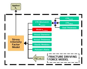
Figure 4-11 Crack driving force model for through-wall cracking
