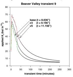
Figure 5-2 Effect of vessel wall thickness on the variation of applied-K<sub>i</sub> vs. time for a 16in. diameter hot-leg break in Beaver Valley. The flaw has the following dimensions: L=0.35 in., 2a=0.50 in, 2c=1.5 in.
