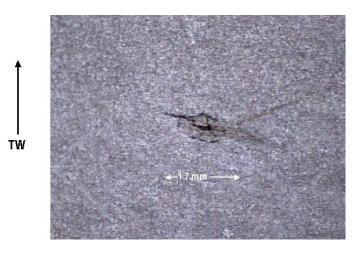
Figure 1 Small Flaw in Plate Material
