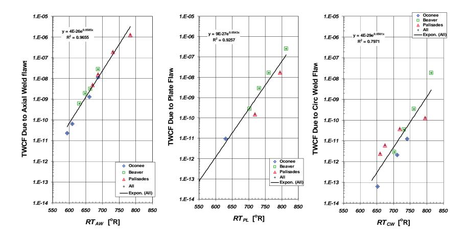
Figure 2-1 Correlation of through-wall cracking frequencies with reference temperature metrics for the three study plants (°R = °F + 459.69) reported in NUREG-1806 [20]
