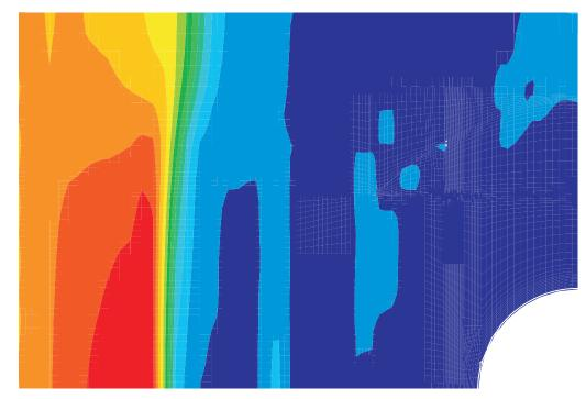
Figure 7-34. Liner Hoop Strains, Posttest Analysis Case D, at 3.5 Pd and 3.6 Pd
