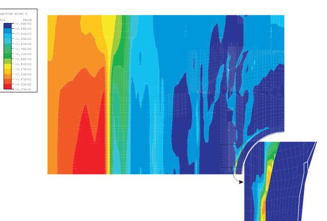
Figure 7-29. Liner Hoop Strains, Posttest Analysis Case C, at 3.5 Pd and 3.6 Pd
