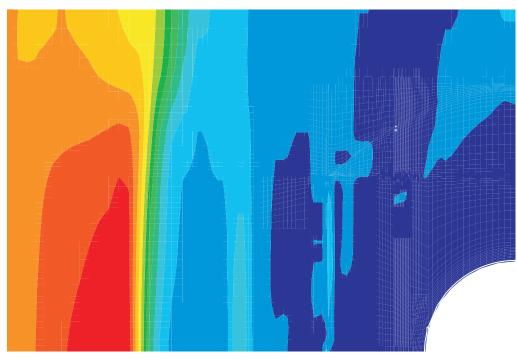
Figure 7-39. Liner Hoop Strains, Posttest Analysis Case E, at 3.5 Pd and 3.6 Pd
