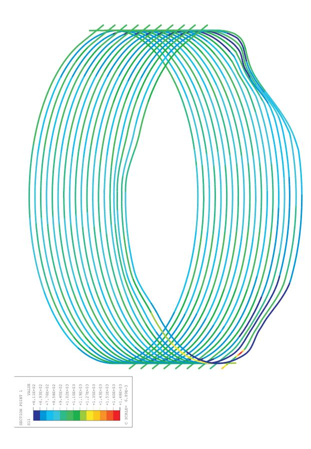
Figure 6-43. 3DCM Posttest Tendon Stress Contours at P = 1.5 Pd, Run 9
