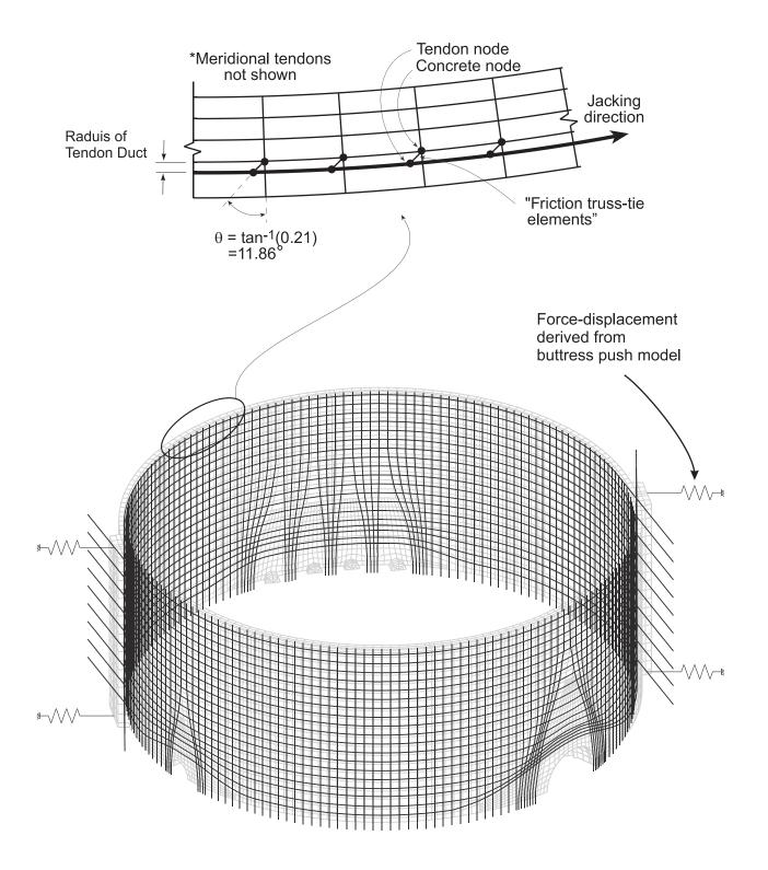
Figure 6-2. Isometric View of 3DCM Tendon Modeling and Added Buttress Springs
