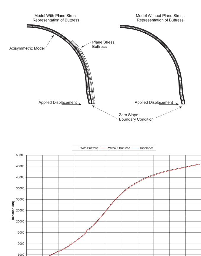
Figure 6-7. Definition of Upper 3DCM Buttress Radial Spring Properties by Axisymmetric Analysis
