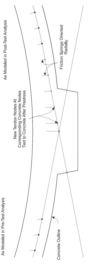
Figure 6-9. Addition of Tendon Ties in Straight Run of Tendons Between Tangent Points and Anchorages
