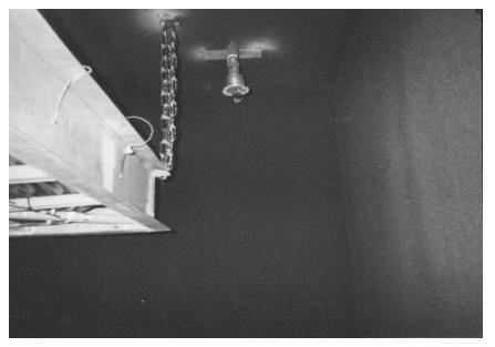
Figure 4-7. Water sprinkler head inside fire test cell.
