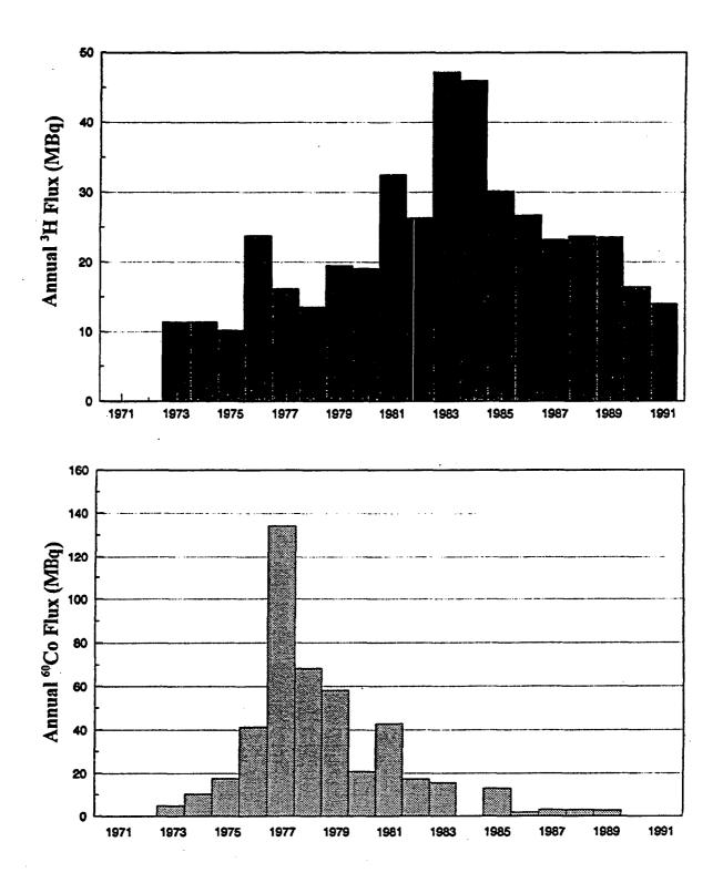
Figure 1.11 Annual flux of <sup>3</sup>H and <sup>60</sup>Co through the Duke Stream weir
