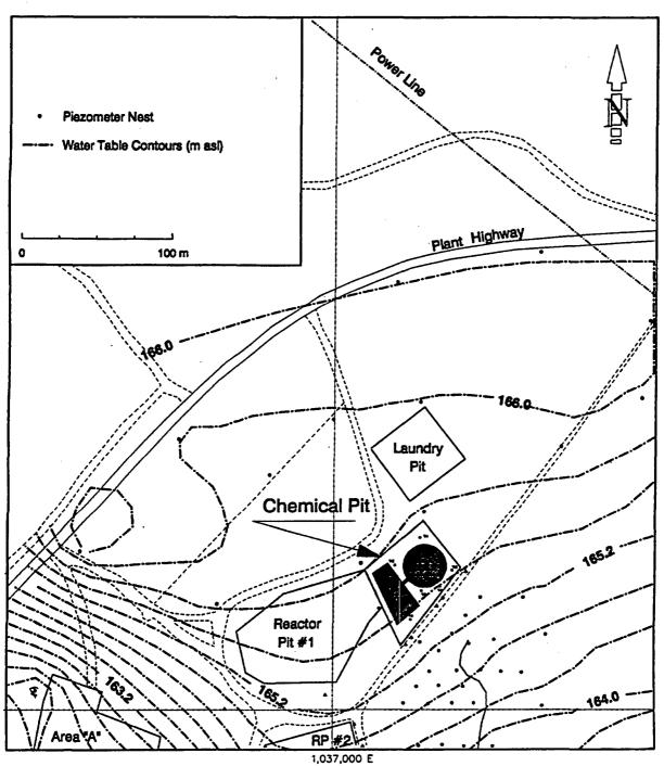
Figure 1.5 Water table contours in the vicinity of the Chemical Pit
