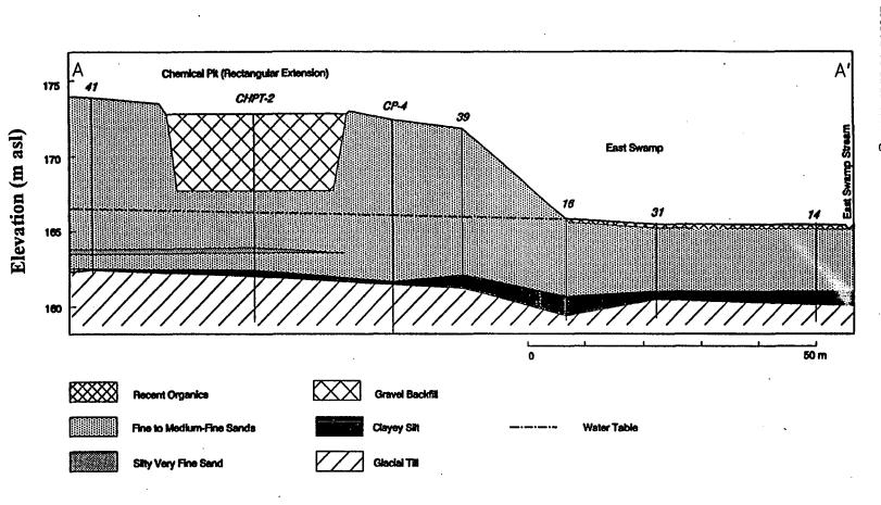
Figure 1.4 Stratigraphic section through the Chemical Pit and East Swamp. Vertical exaggeration 2.5X. Refer to A-A' in Figure 1.3.
