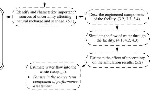
Figure 2.1 Flowchart for the Hydrologic Evaluation Methodology. Chapter 2 discusses the processes and factors affecting recharge and seepage as well as methods for estimating recharge. Numbers indicate sections in this document in which the items are discussed.
