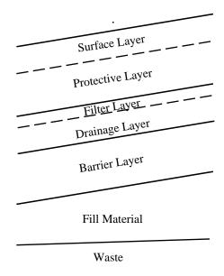
Figure 3.4 Illustration of cover system components
