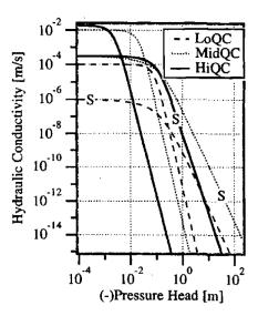
Figure 6.8 Water retention and hydraulic conductivity curves for Hi-, Mid-, and LoQC sand and gravel materials. Curves labeled with an "S" are sand, and the others are gravel (MidQC and LoQC water retention curves for sand coincide).
