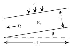
Figure 3.5 Parameters used in evaluating drainage
