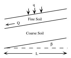
Figure 3.7 Illustration of a capillary barrier
