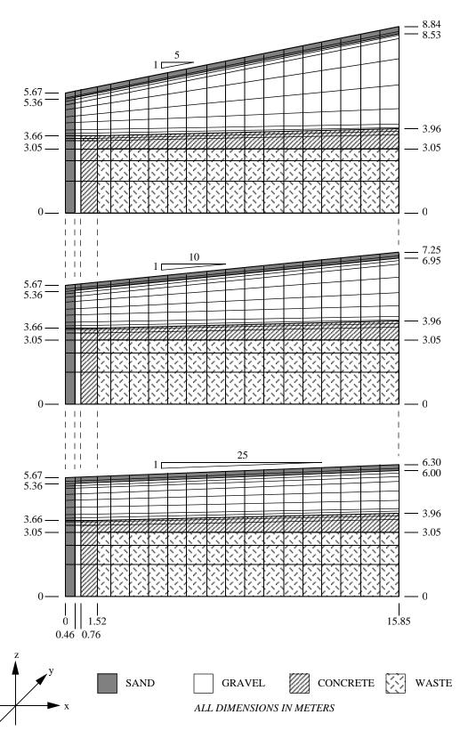
Figure 6.7 Elevation (XY) perspectives of the three-dimensional model for three capillary barrier slopes.
