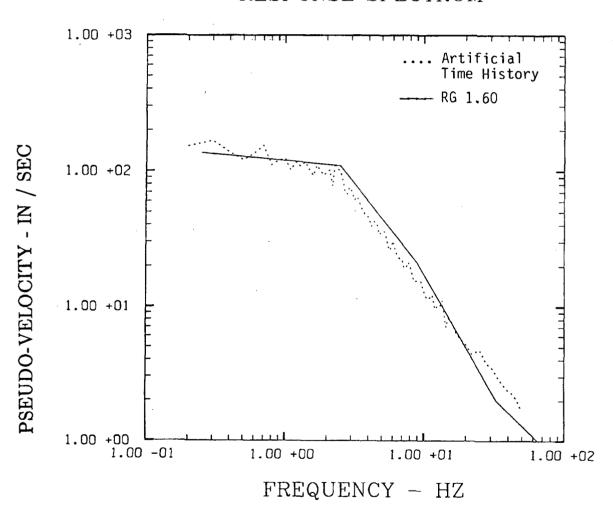
Figure 4. 2% DAMPED PSEUDO RELATIVE VELOCITY RESPONSE SPECTRUM ASSOCIATED WITH PSD2 AND ENVELOPE FUNCTION A COMPARED TO RG 1.60
