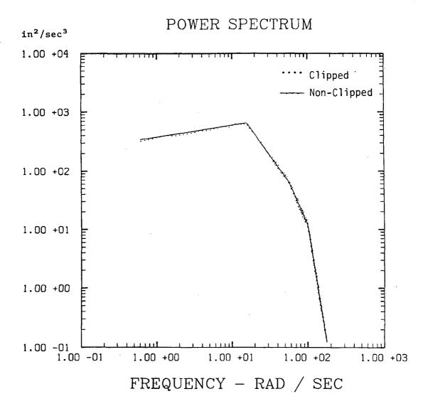
Figure 12. PSD OBTAINED FROM CLIPPED VERSUS NON-CLIPPED TIME HISTORIES
