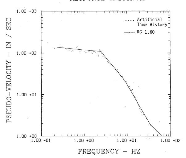
Figure 13. 2% DAMPED PSEUDO RELATIVE VELOCITY RESPONSE SPECTRUM OBTAINED FROM PSD3 AND ENVELOPE FUNCTION A WITH TIME HISTORY CLIPPED AT 1.0g
