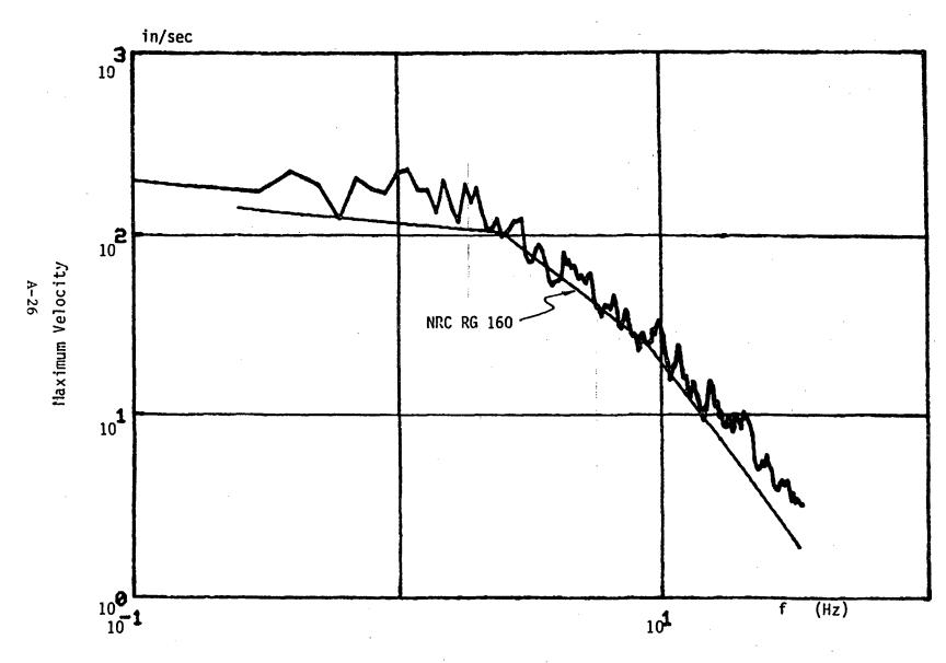
Fig. 2 Velocity Spectrum; Parameter Set No. 2 (From Reference 3)
