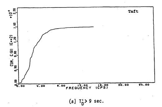
FIGURE 3. CUMULATIVE SPECTRAL DENSITY FUNCTIONS OF EFFECTIVE ACCELEROGRAM SEGMENT DEFINED BY  $T_D^1 = T_m - T_{.05}$  (Reproduced from Ref.  $\underline{4}$ )
