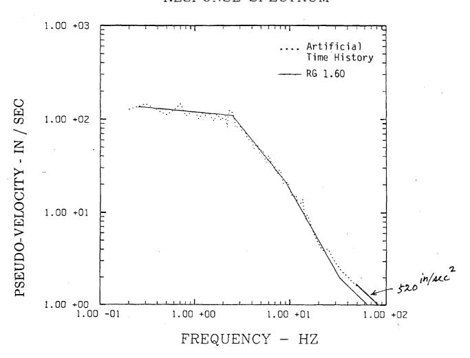
Figure 8. 2% DAMPED PSEUDO RELATIVE VELOCITY RESPONSE SPECTRUM ASSOCIATED WITH PSD3 AND ENVELOPE FUNCTION A COMPARED TO RG 1.60
