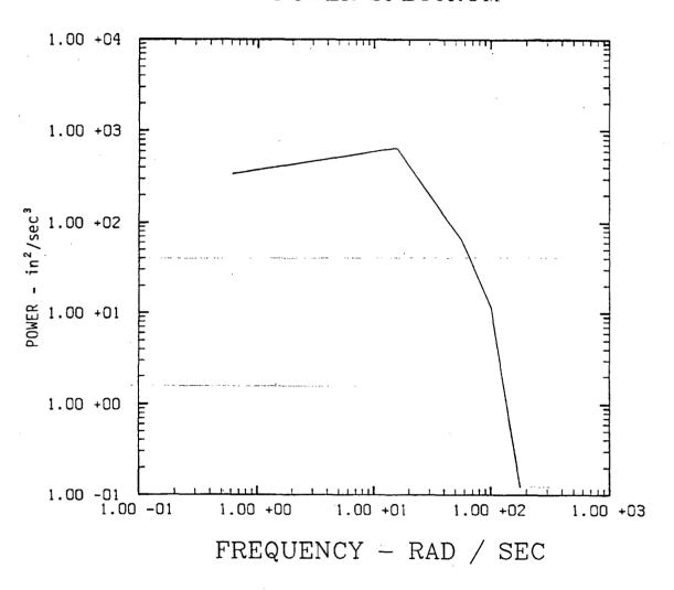
Figure 5. RECOMMENDED MINIMUM POWER SPECTRAL DENSITY REQUIREMENT  $(\underline{PSD3})$
