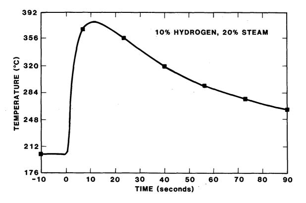
Figure 15. Typical Temperature Response for Flat-Plate Calorimeter
