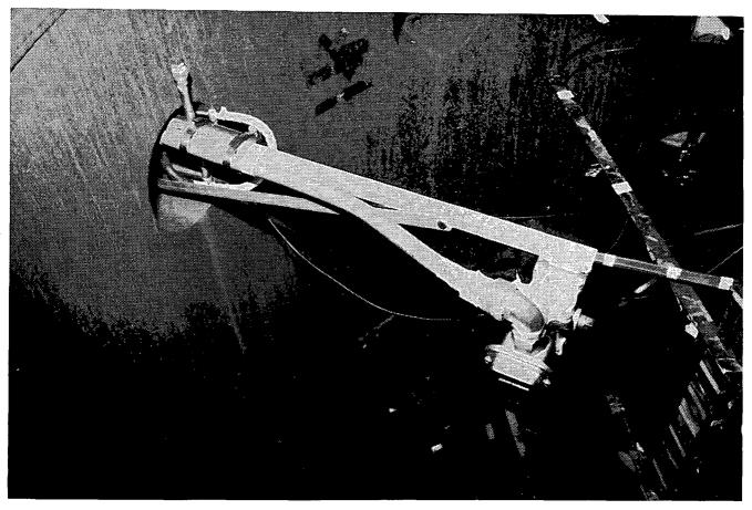
Figure 9. Solenoid Valve Mounted in FITS Test Vessel
