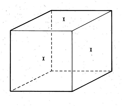
Figure 7. Location of Thermocouples on Solid and Hollow Cube Calorimeters
