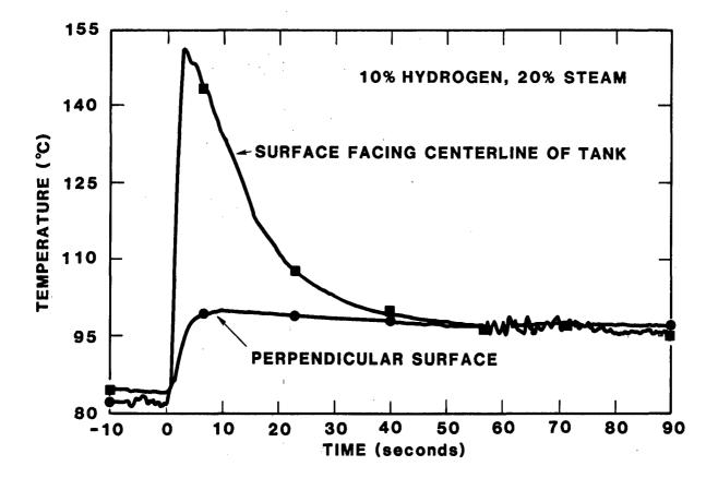
Figure 20. Surface Temperature Response of Mixing Fan
