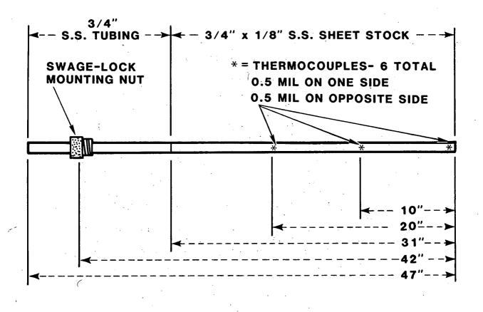
Figure 3. Schematic Drawing of Thermocouple Probe
