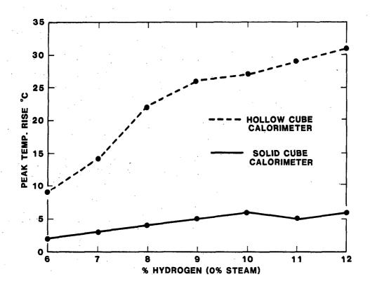
Cube Calorimeters: Effect of Hydrogen Concentra-tion on Peak Temperature Rise Figure 18.
