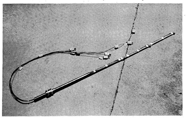
Figure 4. Photograph of Thermocouple Probe
