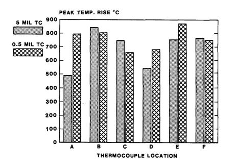
Figure 13. Thermocouple Response Comparison
