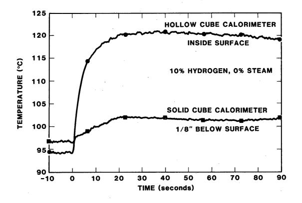
Figure 17. Typical Temperature Responses of Hollow and Solid Cube Calorimeters
