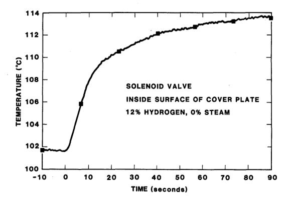
Figure 19. Typical Temperature Response of Solenoid Valve
