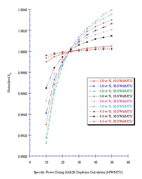
Figure A-5: Reactivity effect of specific power during depletion on k<sub>inf</sub> in an array of fuel pins (actinides only).<sup>10</sup>
