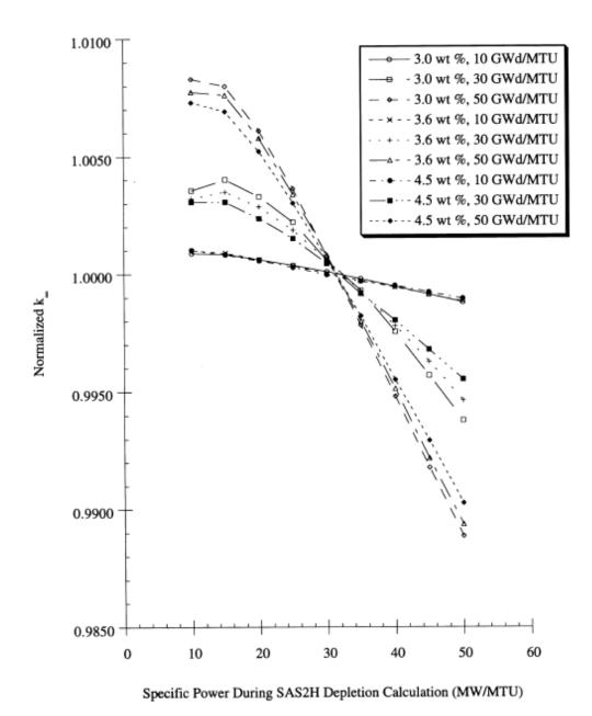
Figure A-6: Reactivity effect of specific power during depletion on k<sub>inf</sub> in an array of fuel pins (actinides and fission products).<sup>10</sup>
