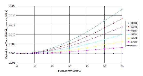
Figure A-3: Reactivity effect of moderator temperature during depletion on  $k_{inf}$  in an array of poisoned storage cells. Results correspond to fuel with 5.0 weight percent initial <sup>235</sup>U enrichment.<sup>9</sup>
