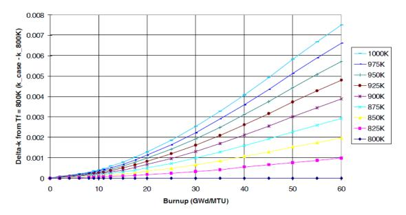
Figure A-2: Reactivity effect of fuel temperature during depletion on  $k_{inf}$  in an array of poisoned storage cells. Results correspond to fuel with 5.0 weight percent initial <sup>235</sup>U enrichment.<sup>9</sup>
