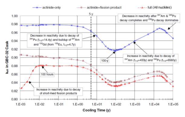
Figure A-1: Reactivity behavior in the GBC-32 cask as a function of cooling time for fuel with 4.0 weight percent <sup>235</sup>U initial enrichment and 40 GWd/MTU burnup<sup>7</sup>
