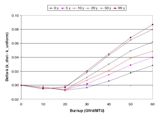
Figure A-7: Effect of axial burnup distribution on  $k_{eff}$  in the GBC-32 cask for actinide-only burnup credit and various cooling times for fuel with 4.0 weight percent initial enrichment.<sup>9</sup>
