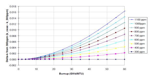
Figure A-4: Reactivity effect of soluble boron concentration during depletion on  $k_{inf}$  in an array of poisoned storage cells. Results correspond to fuel with 5.0 weight percent initial <sup>235</sup>U enrichment.<sup>9</sup>
