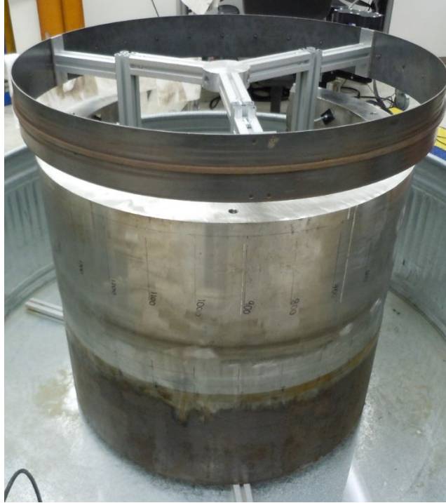
Figure 4-5 Specimen 14C-146 – 914 mm (36 in) Diameter, 84 mm (3.3 in.) Wall Thickness, PWR Primary Loop Hot Leg Specimen
