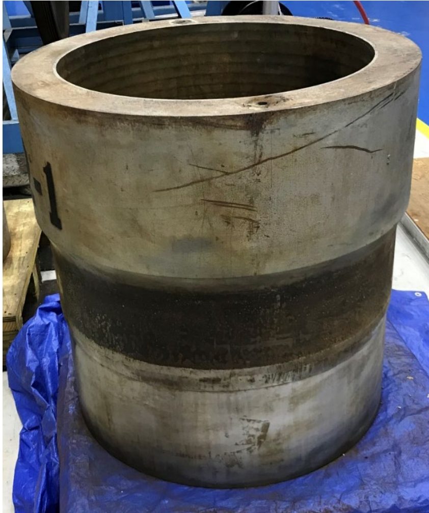
Figure 4-7 Specimen 602—Primary Loop Cold Leg Nozzle to Safe-End Weld with an 864 mm (34 in.) Diameter and an Average Wall Thickness of 74 mm (2.9 in.)
