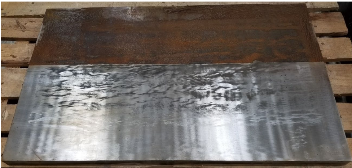
Figure 4-10 Specimen 21C-303-3 1.25 in. Wall Thickness Dissimilar Metal Weld Flat Plate
