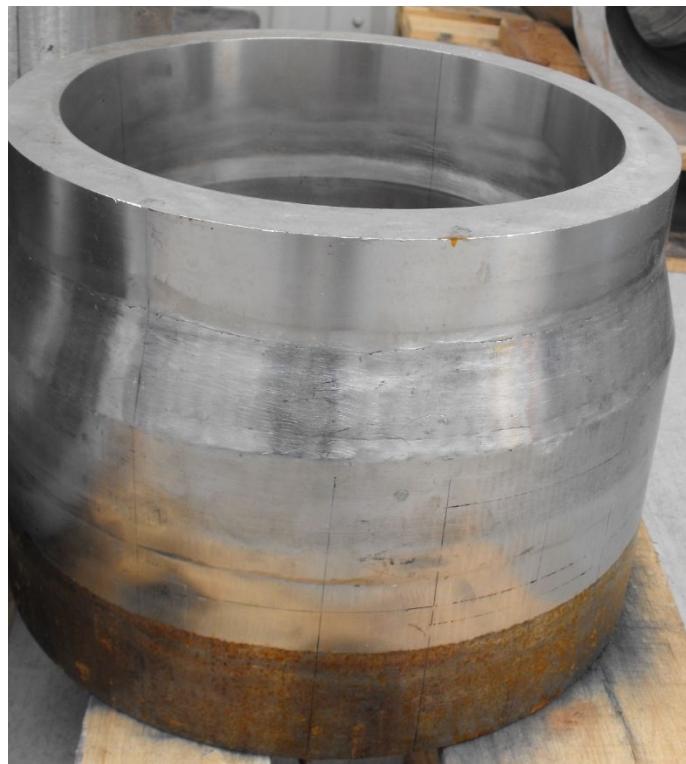
Figure 4-1 Specimen 8C-032 – 318 mm Diameter (12.75 in.) Dissimilar Metal Carbon Steel Nozzle to 316 Stainless Steel Safe-End with an Average Wall Thickness of 32 mm (1.5 in.)
