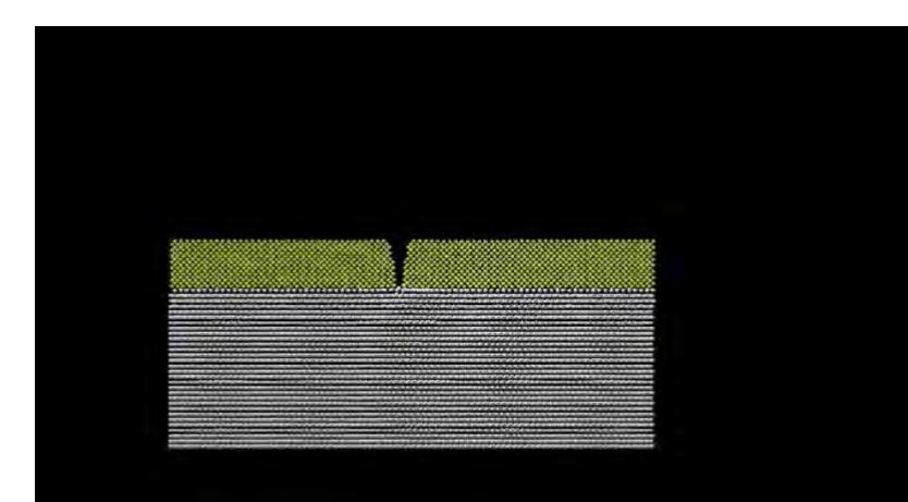
Under lateral strain, a pre-existing crack in the Cr coating causes pitting of the exposed Zr substrate.
