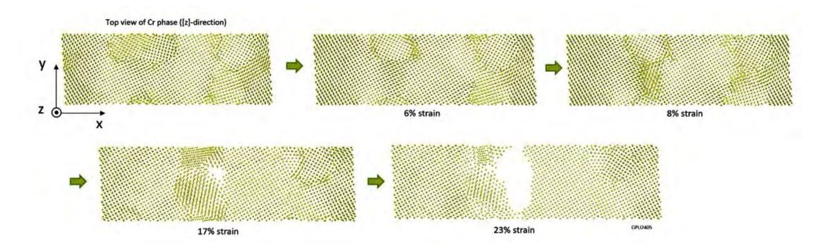
Subject to tensile strain, a model with columnar grains (shown above) expose the underlying Zr at a strain of 17%, which is similar to that of a monocrystalline Cr coating.
