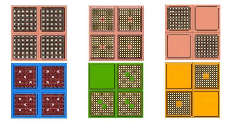
Flux-trap and non-flux-trap SFP rack designs, 1-out-of-4 to 4-out-of-4 configurations
