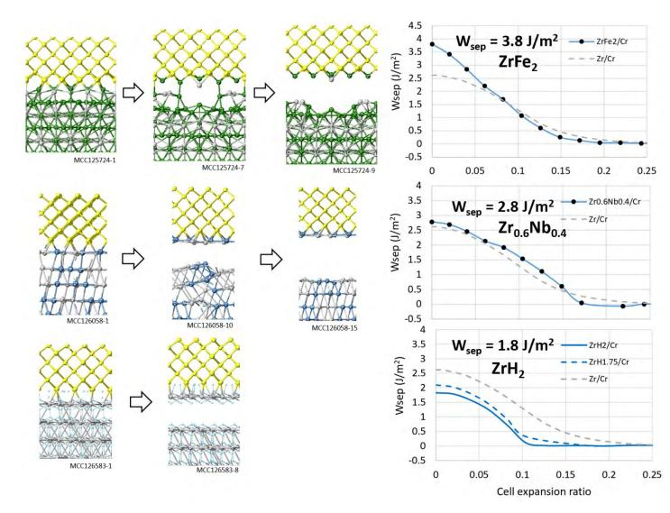
Precipitation of ZrFe<sub>2</sub> strengthens the interface, but potentially introduces brittleness
