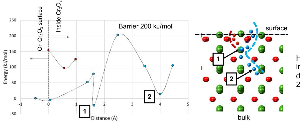
H atoms can be trapped in  $Cr_2O_3$  and have high diffusion barriers (about 200 kJ/mol).
