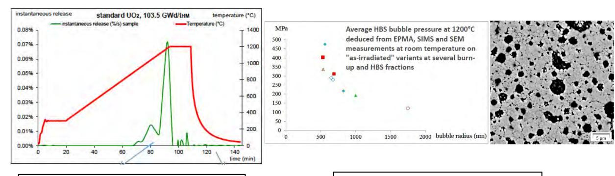
Measuring gas release upon heating
