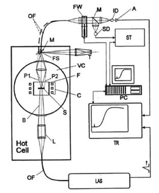
• Induction + multiple laser pulse heating
