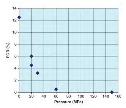
High hydrostatic restraint pressures prevented fission gas release and thus fragmentation
