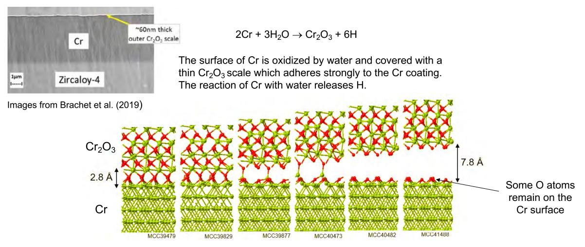
Work of separating  $Cr_2O_3$  from Cr surface: **3.1 J/m<sup>2</sup>**
