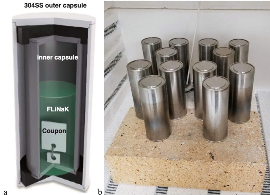
Figure 3-1. (a) schematic of standard inner and outer molten salt capsule and (b) capsules loaded in box furnace for isothermal testing. The wire and nipple used to secure the specimen in (a) were the same material as the capsule
