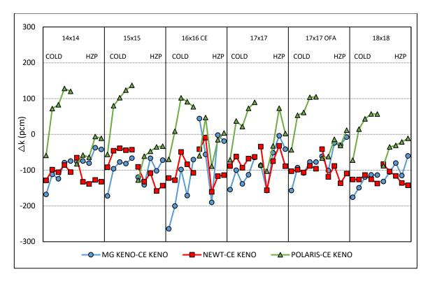
Figure B-15 Test Suite 1: Effect of Boron Concentration on k<sub>inf</sub> Differences for Uncontrolled Cases
