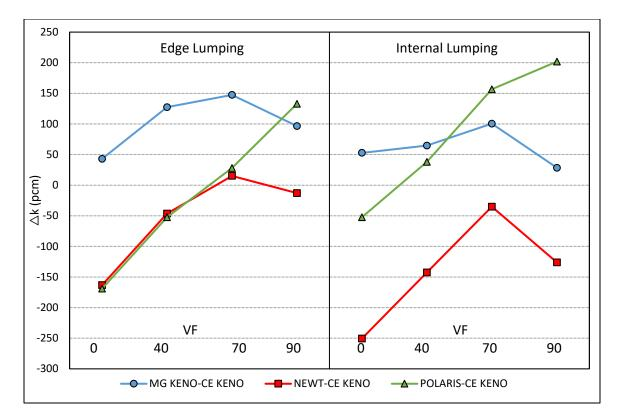
Figure B-60 Test Suite 10: k<sub>inf</sub> Differences for BWR Uncontrolled Cases
