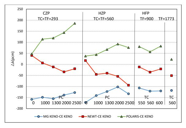
Figure B-34 Test Suite 3: 15 × 15 MOX PWR Lattice k<sub>inf</sub> Differences for ncontrolled Cases
