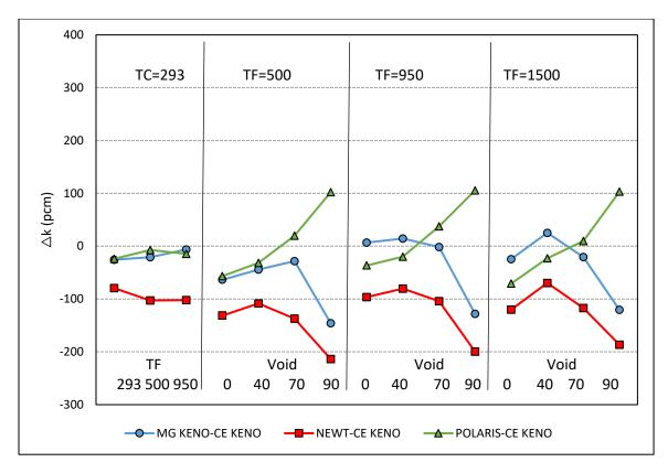
Figure B-28 Test Suite 3: MOX BWR k<sub>inf</sub> Differences for Controlled Cases
