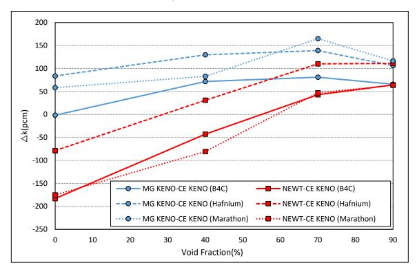
Figure B-23 Test Suite 2: MG KENO and NEWT k<sub>inf</sub> Void Fraction Trends for Different Control Blade Types
