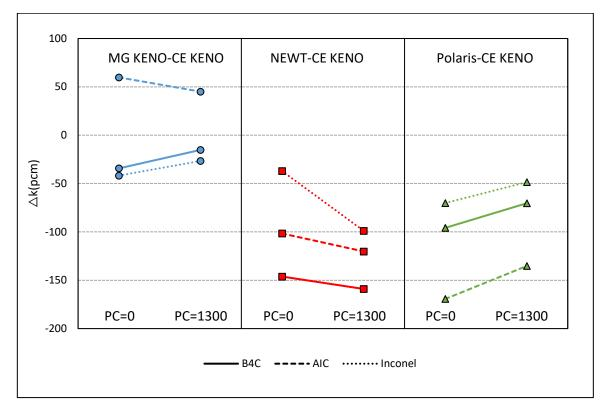
Figure B-25 Test Suite 2: k<sub>inf</sub> Boron Trends for Different Control Rod Types
