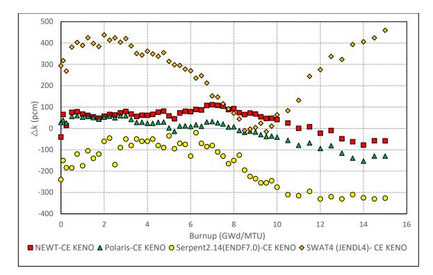
Figure B-72 Test Suite 13: BWR k<sub>inf</sub> Differences with Depletion for 40% Void Fraction
