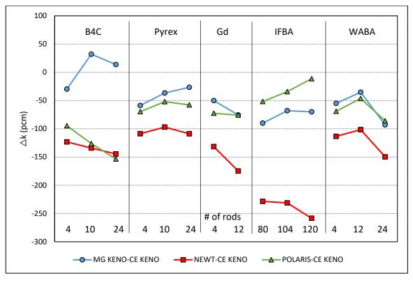
Figure B-66 Test Suite 10: PWR k<sub>inf</sub> Differences
