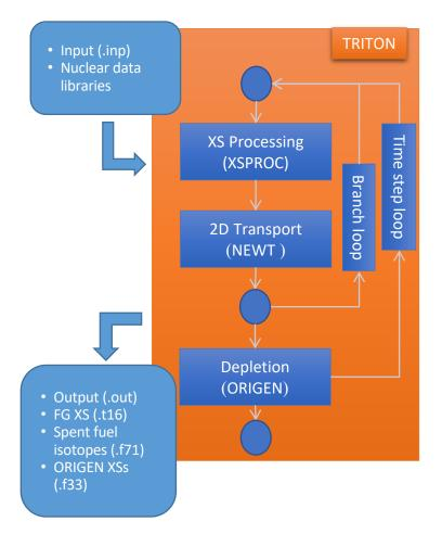
Figure 3-1 TRITON/NEWT Lattice Physics Calculation Flow
