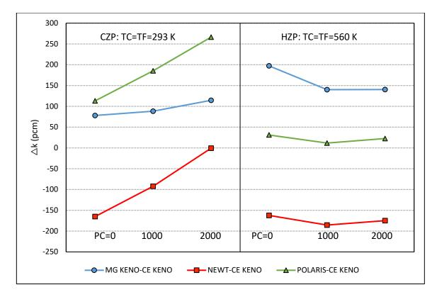
Figure B-43 Test Suite 6: BWR Lattice k<sub>inf</sub> Differences for Boron Variations
