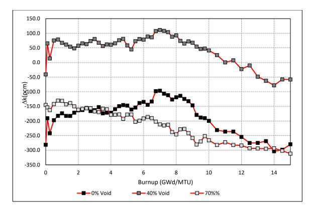
Figure B-40 Test Suite 5: 8 × 8 BWR Lattice NEWT k<sub>inf</sub> Differences
