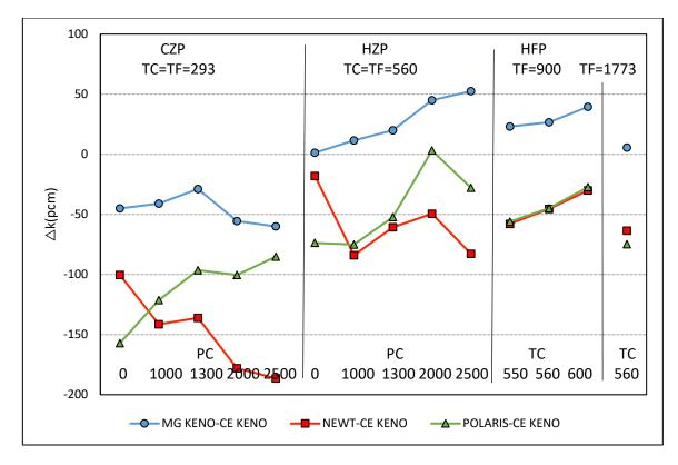
Figure B-33 Test suite 3 17 × 17 MOX PWR Lattice k<sub>inf</sub> Differences for Controlled Cases
