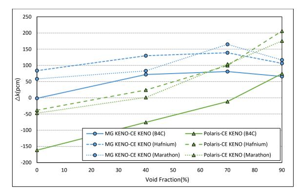
Figure B-24 Test Suite 2: k<sub>inf</sub> MG KENO and Polaris Void Fraction Trends for Different Control Blade Types
