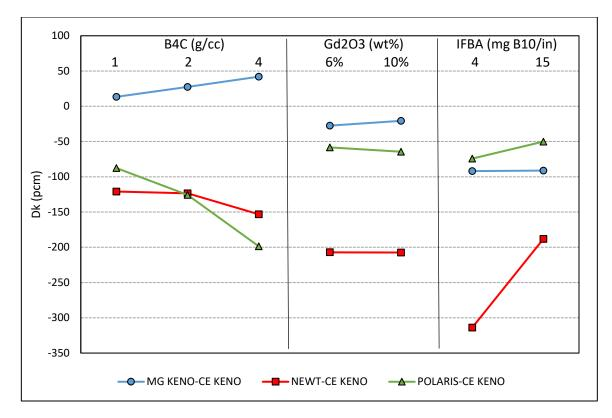
Figure B-57 Test Suite 9: k<sub>inf</sub> Differences for Uncontrolled PWR Cases
