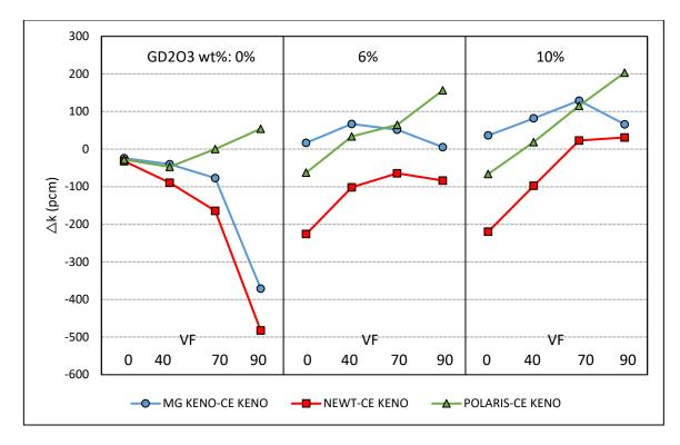
Figure B-55 Test suite 9: k<sub>inf</sub> Differences for Uncontrolled BWR Cases
