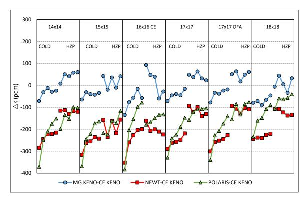
Figure B-16 Test Suite 1: Effect of Boron Concentration on k<sub>inf</sub> Differences for Controlled Cases
