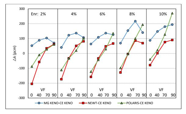
Figure B-49 Test Suite 7: k<sub>inf</sub> Differences for Controlled BWR Cases
