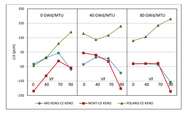
Figure B-38 Test Suite 4: 10 × 10 BWR Lattice k<sub>inf</sub> Differences
