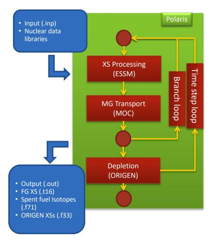
Figure 3-2 Polaris Lattice Physics Calculation Flow
