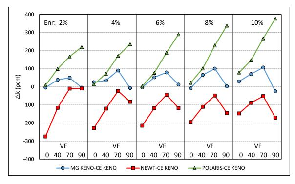
Figure B-48 Test Suite 7: k<sub>inf</sub> Differences for Uncontrolled BWR Cases
