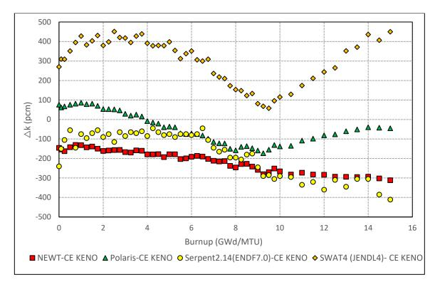
Figure B-73 Test Suite 13: BWR k<sub>inf</sub> Differences with Depletion for 70% Void Fraction
