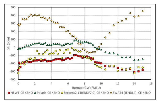
Figure B-71 Test Suite 13: BWR k<sub>inf</sub> Differences with Depletion for 0% Void Fraction
