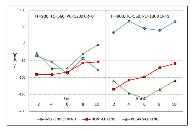
Figure B-51 Test Suite 7: k<sub>inf</sub> Differences for Uncontrolled and Controlled PWR Cases
