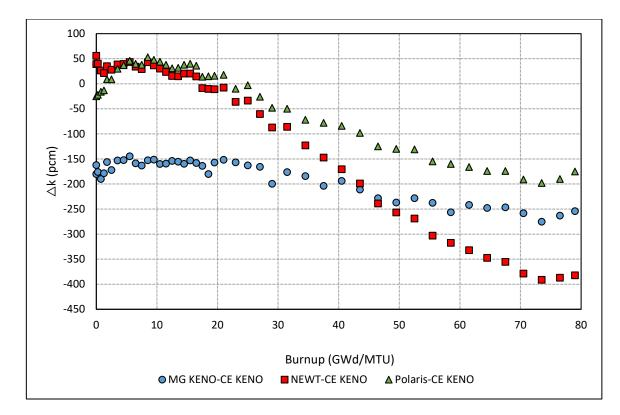
Figure B-42 Test Suite 5: 17 × 17 PWR Lattice k<sub>inf</sub> Differences
