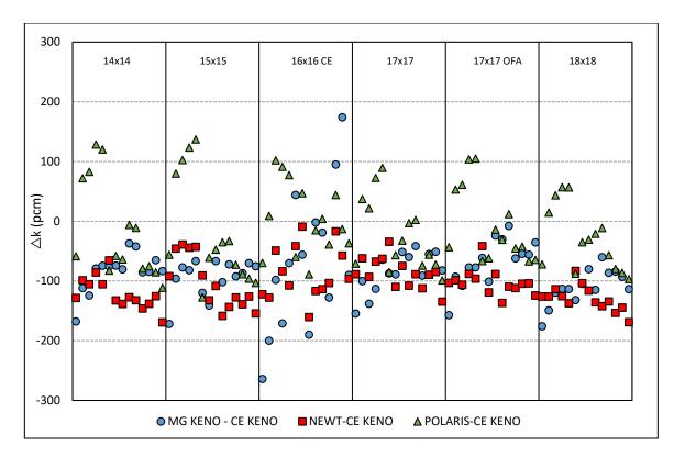
Figure B-13 Test Suite 1: PWR k<sub>inf</sub> Comparisons for Uncontrolled Cases
