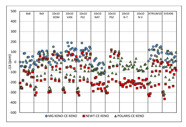
Figure B-2 Test Suite 1: BWR k<sub>inf</sub> Comparisons for Controlled Cases
