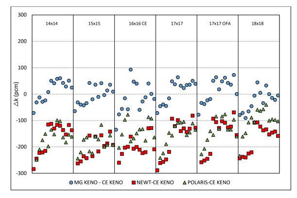
Figure B-14 Test Suite 1: PWR k<sub>inf</sub> Comparisons for Controlled Cases
