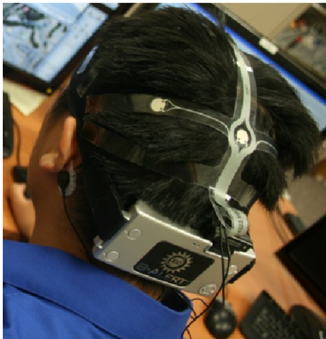
Figure 2-4 ABM's X 10 EEG/ECG system
