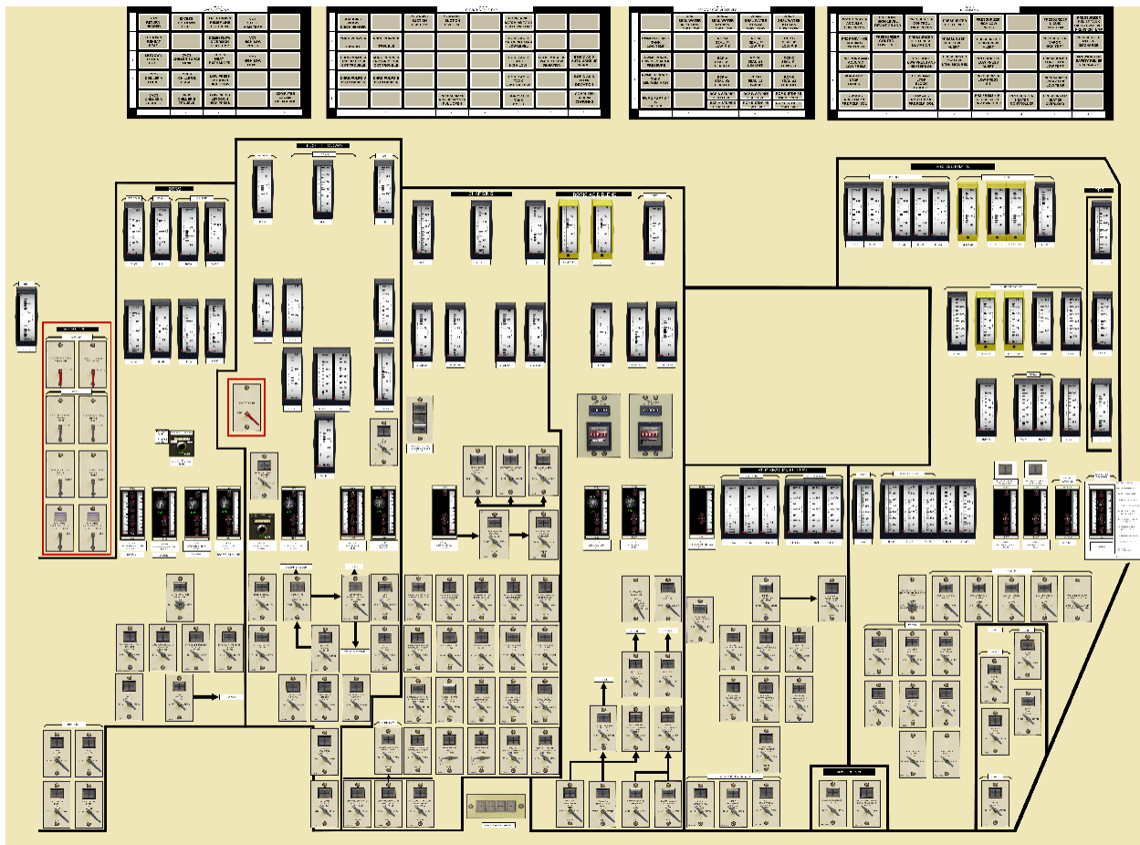
Figure 2-2 An Example of a Digitally Represented Analog NPP MCR Control Panel
