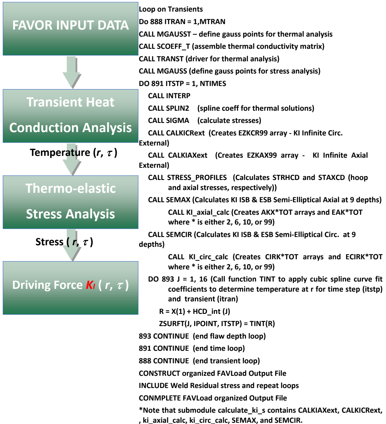
Figure 5: FAVLoad Calculational Flow and Subroutines Called to Generate FAVLoad Output file for use by FAVPFM
