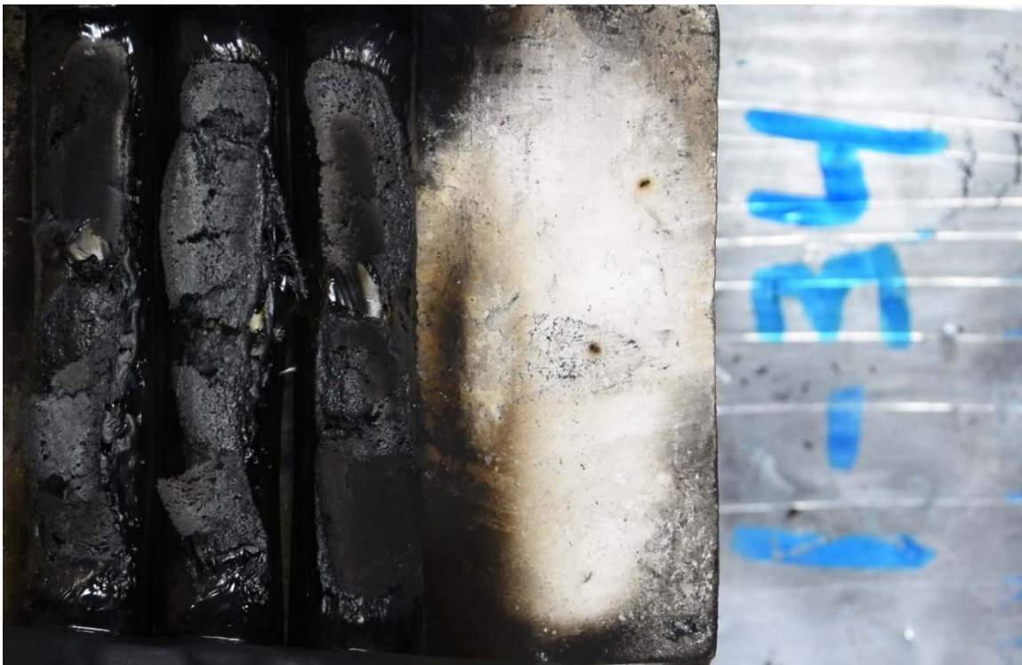
Figure B-4 Photo of SNL Test 1-34 ( 25 \text{ MJ/m}^2 ), sample classified as “insulation exposure”
