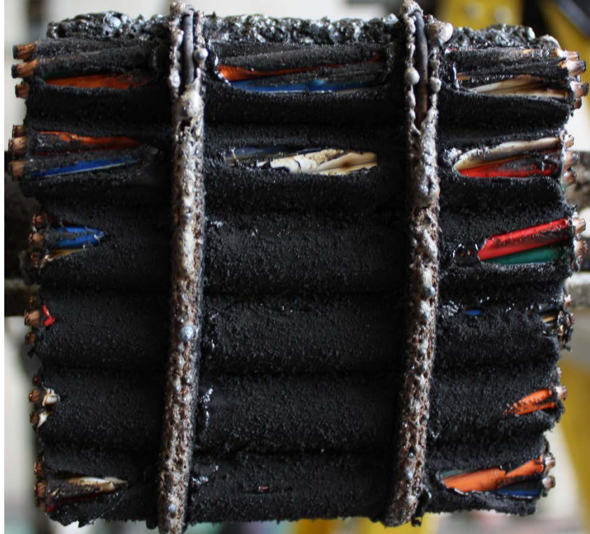
Figure B-3 Photo of NRC Test 2-21 Rack 2 sample 1-23 ( 7.8 \text{ MJ/m}^2 ), sample classified as “insulation exposure”
