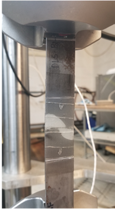
Figure D-3 Double-lap shear test setup at Emc 2 laboratory
