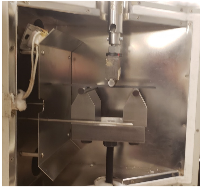
Figure C-1 Flexural test setup at Emc 2 laboratory showing flexural specimen in three-point bending
