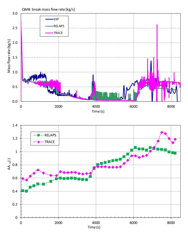
Figure 5-8 Break Mass Flow Rate (QMB): a) Visual Observation (Top), b) Accuracy Measure AA<sub>m</sub> (Bottom)
