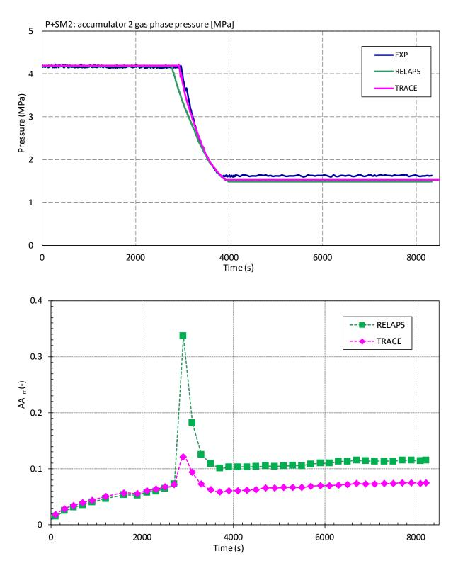
Figure 5-3 Accumulator 2 Gas Phase Pressure (P+SM2): a) Visual Observation (Top), b) Accuracy Measure AA<sub>m</sub> (Bottom)
