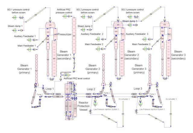
Figure 3-1 RELAP5 Hydraulic Components View of BETHSY Facility
