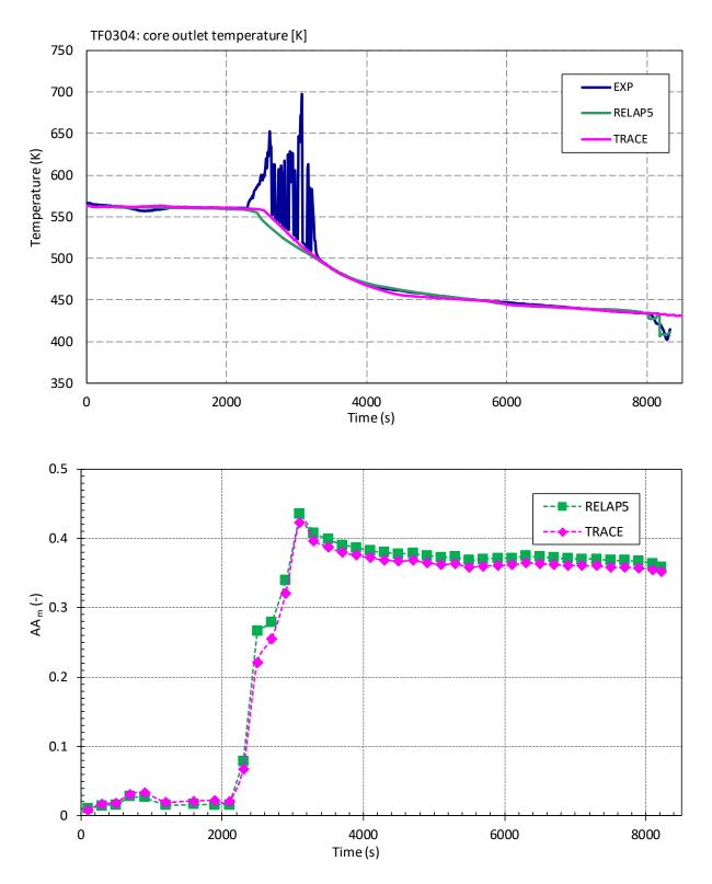
Figure 5-5 Core Outlet Temperature (TF0304): a) Visual Observation (top), b) Accuracy Measure AA<sub>m</sub> (Bottom)
