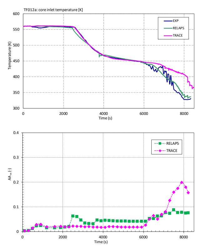
Figure 5-4 Core Inlet Temperature (TF012A): a) Visual Observation (top), b) Accuracy Measure AA<sub>m</sub> (Bottom)
