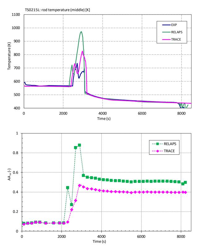
Figure 5-11 Rod Temperature (Middle) (TS0215L): a) Visual Observation (Top), b) Accuracy Measure AA<sub>m</sub> (Bottom)
