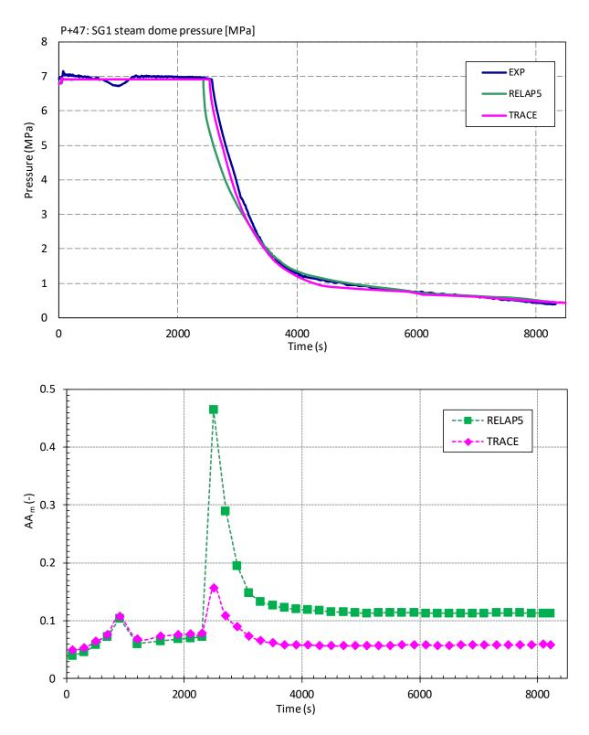
Figure 5-2 SG1 Steam Dome Pressure (P+47): a) Visual Observation (Top), b) Accuracy Measure AA<sub>m</sub> (Bottom)
