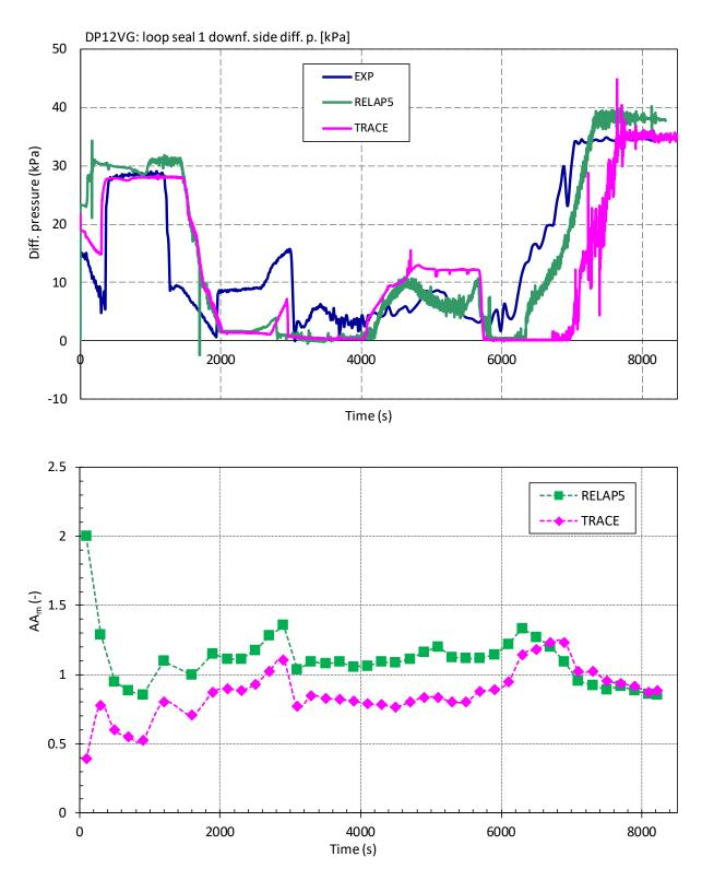
Figure 5-17 Loop Seal 1 Downflow Side Differential Pressure (DP12VG): a) Visual Observation (Top), b) Accuracy Measure AA<sub>m</sub> (Bottom)
