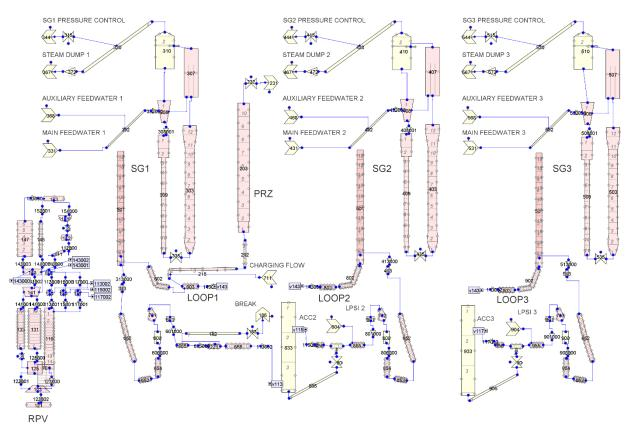
Figure 3-3 TRACE Hydraulic Components View of BETHSY Facility
