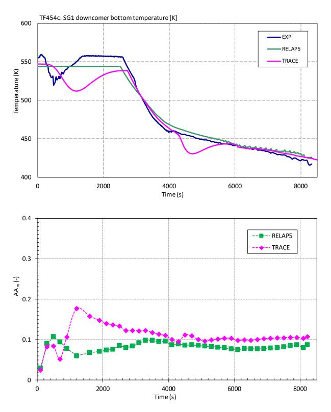
Figure 5-7 SG1 Downcomer Bottom Temperature (TF454C): a) Visual Observation (Top), b) Accuracy Measure AA<sub>m</sub> (Bottom)
