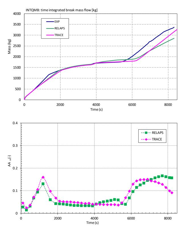
Figure 5-9 Time Integrated Break Mass Flow (INTQMB): a) Visual Observation (Top), b) Accuracy Measure AA<sub>m</sub> (Bottom)
