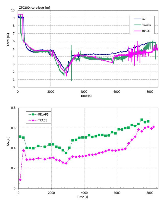
Figure 5-13 Core Collapsed Level (ZT0200): a) Visual Observation (Top), b) Accuracy Measure AA<sub>m</sub> (Bottom)
