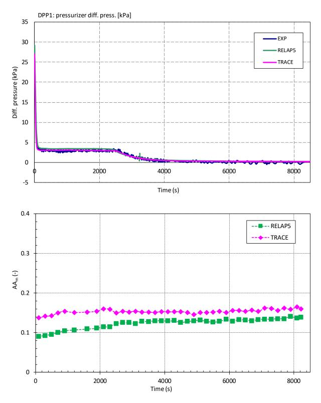
Figure 5-19 Pressurizer Differential Pressure (DPP1): a) Visual Observation (Top), b) Accuracy Measure AA<sub>m</sub> (Bottom)
