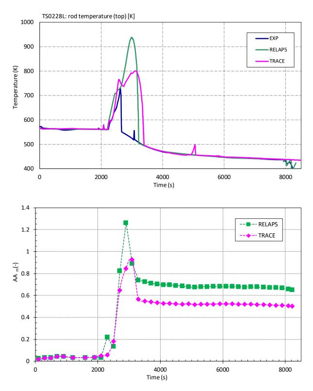
Figure 5-12 Rod Temperature (Top) (TS0228L): a) Visual Observation (Top), b) Accuracy Measure AA<sub>m</sub> (Bottom)
