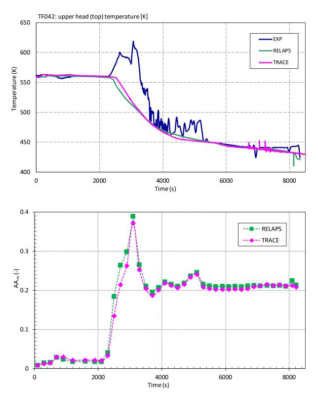
Figure 5-6 Upper Head (Top) Temperature (TF042): a) Visual Observation (Top), b) Accuracy Measure AA<sub>m</sub> (Bottom)
