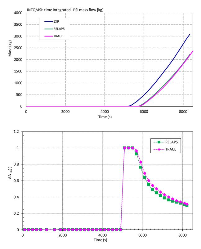
Figure 5-10 Time Integrated LPSI Mass Flow (INTQMSI): a) Visual Observation (Top), b) Accuracy Measure AA<sub>m</sub> (Bottom)
