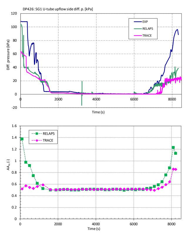
Figure 5-14 SG1 U-Tube Upflow Side Differential Pressure (DP426): a) Visual Observation (Top), b) Accuracy Measure AA<sub>m</sub> (Bottom)
