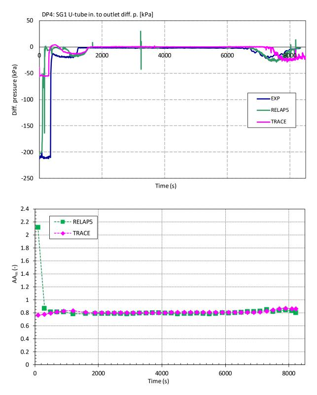
Figure 5-15 SG1 U-tube Inlet to Outlet Differential Pressure (DP4): a) Visual Observation (Top), b) Accuracy Measure AA<sub>m</sub> (Bottom)
