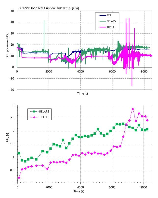
Figure 5-18 Loop Seal 1 Upflow Side Differential Pressure (DP12VP): a) Visual Observation (Top), b) Accuracy Measure AA<sub>m</sub> (Bottom)
