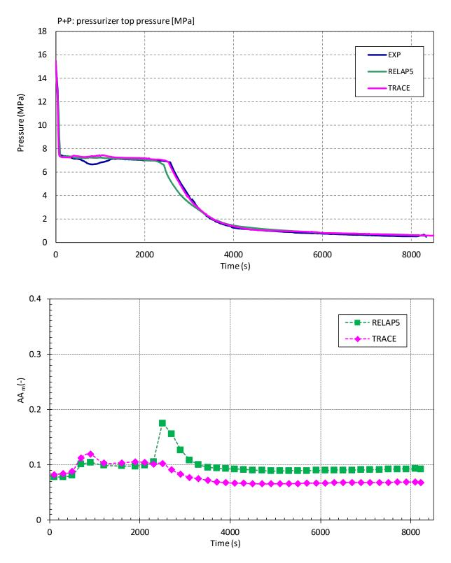
Figure 5-1 Pressurizer Top Pressure (P+P): a) Visual Observation (Top), b) Accuracy Measure AA<sub>m</sub> (Bottom)
