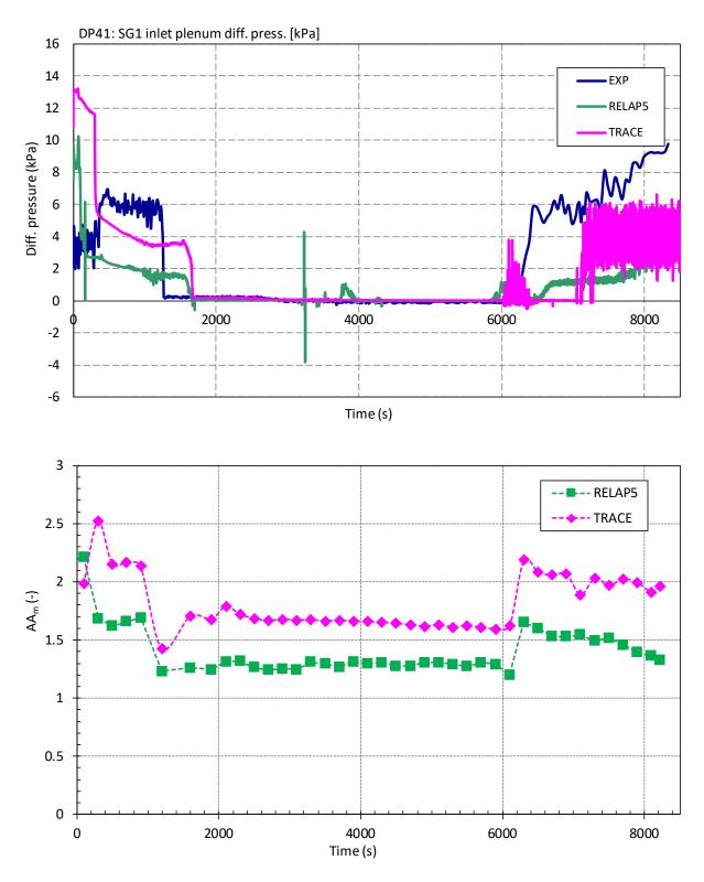
Figure 5-20 SG1 Inlet Plenum Differential Pressure (DP41): a) Visual Observation (Top), b) Accuracy Measure AA<sub>m</sub> (Bottom)
