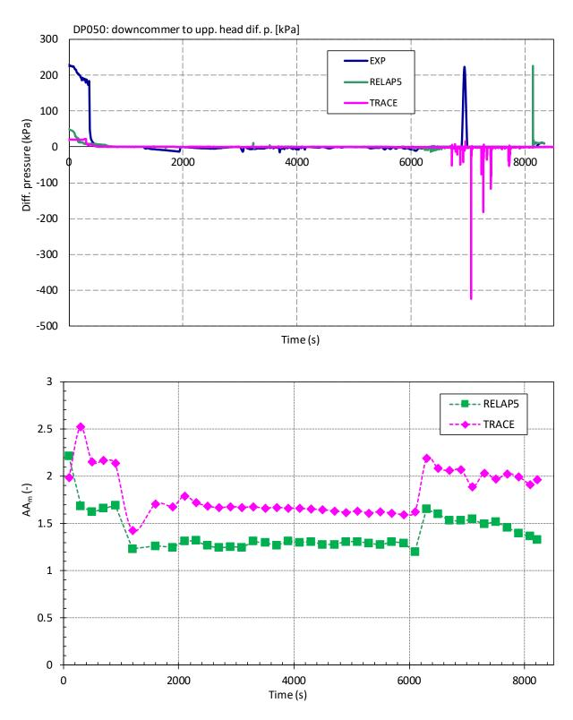
Figure 5-21 Downcommer to Upper Head Differential Pressure (DP050): a) Visual Observation (Top), b) Accuracy Measure AA<sub>m</sub> (Bottom)
