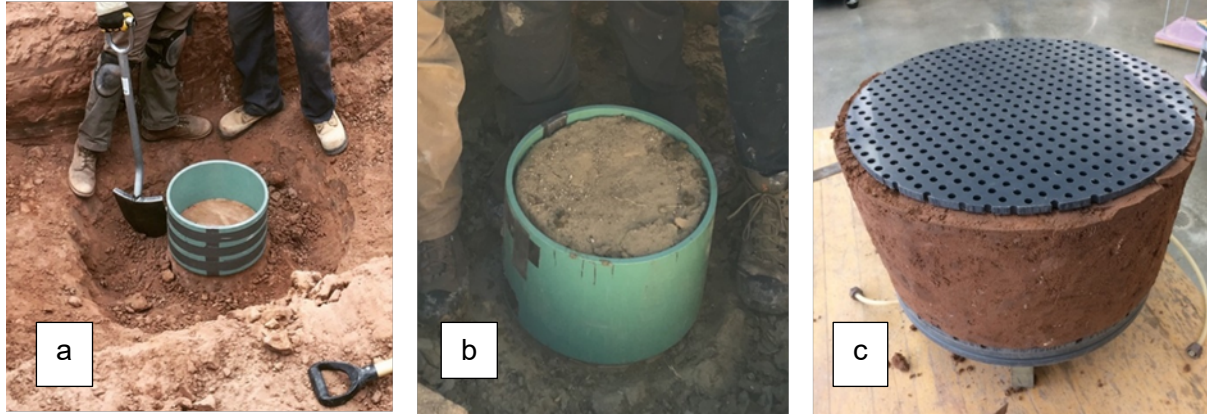
Figure 3-3 Block Samples from Radon Barriers to Characterize Hydraulic Properties: (a) trimming block sample into containment ring, (b) block sample within PVC containment ring, and (c) block sample trimmed to 305 mm diameter in the laboratory for hydraulic properties testing.
