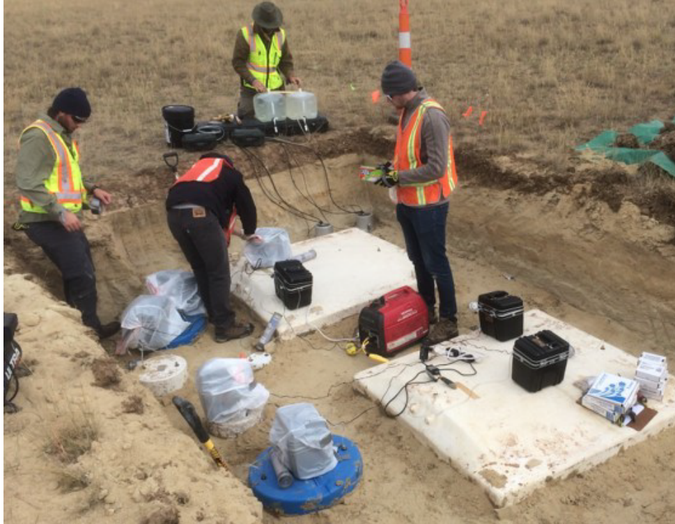
Figure 4-1 Field Installation of Eight Flux Chambers of Four Sizes on the Top of the Radon Barrier at Shirley Basin South
