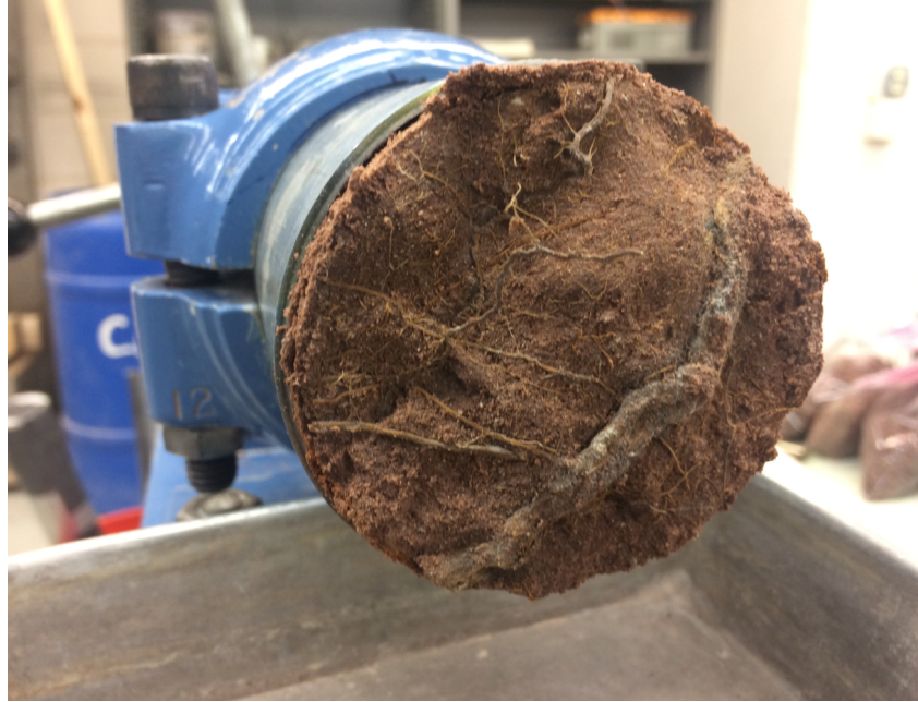
Figure 4-18 Large Root in the Radon Barrier in a Shelby Tube Sample from Bluewater Test Pit 5 here Fluxes were High and Exhibited a Wide Range
