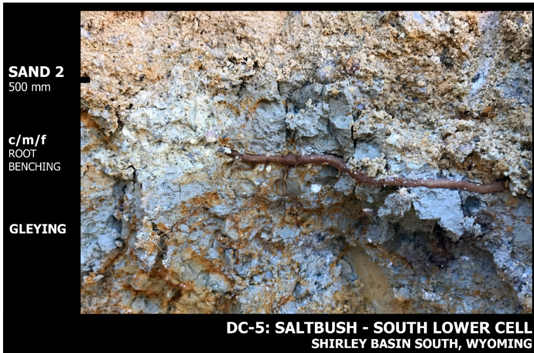
Figure 6-34 Gleying in a Clay Lens Located Above the Radon Barrier at Shirley Basin South, Wyoming
