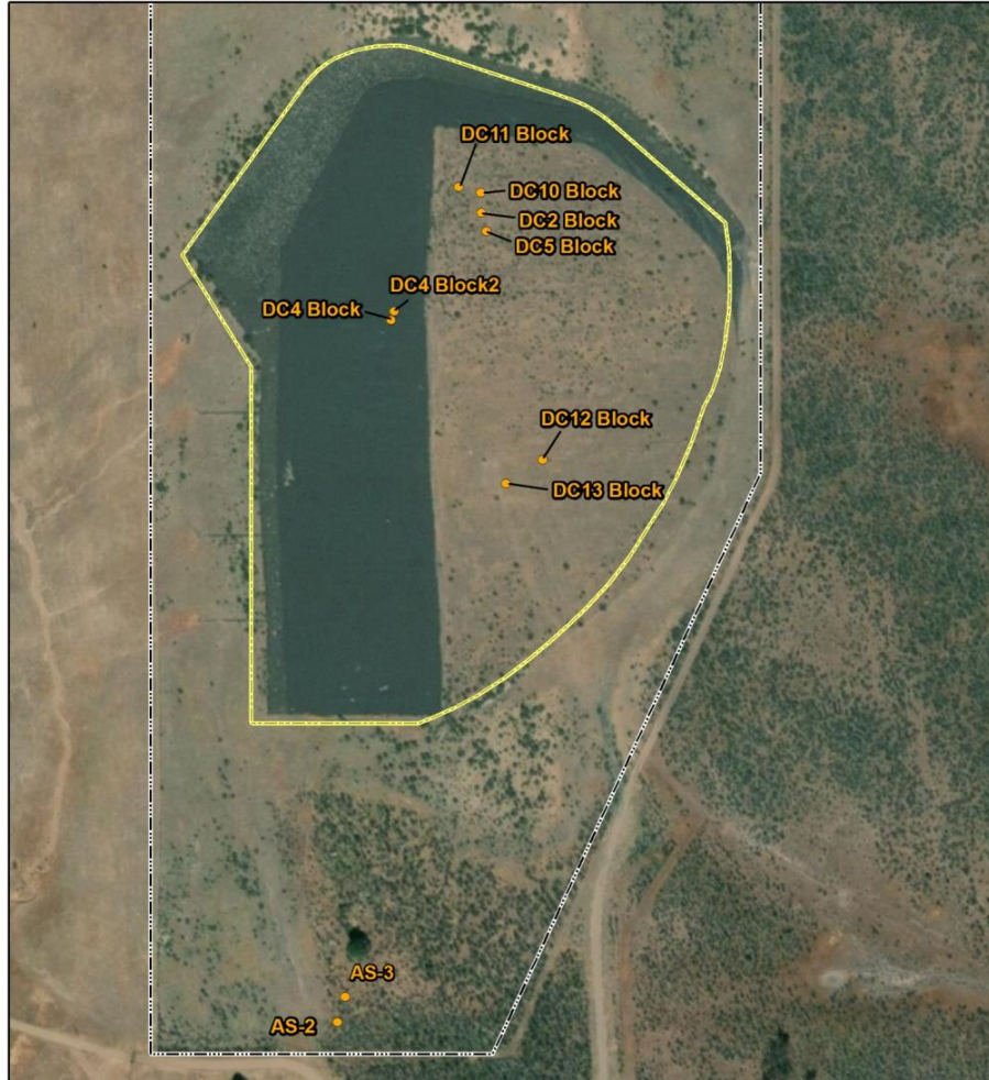
Figure 2-7 Test Pit Locations on the Disposal Cell Top-Deck, Side Slope, and at Analogue Sites (AS) for Lakeview, Oregon
