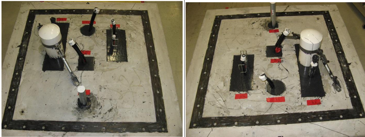
Figure 4-16 Photos of Test Deck 3 After Seal Assembly Installation
