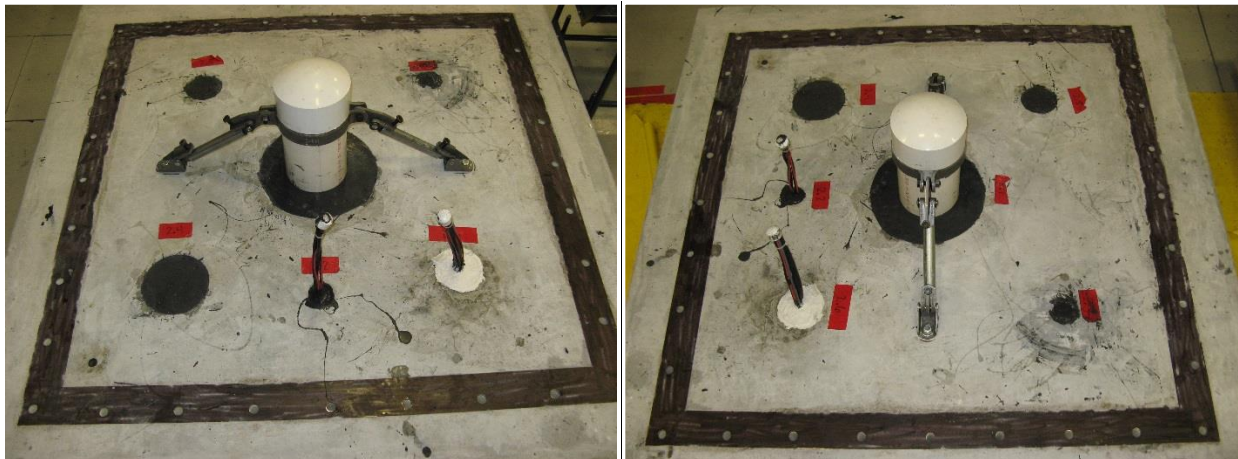
Figure 4-13 Photos of Test Deck 2 After Seal Assembly Installation
