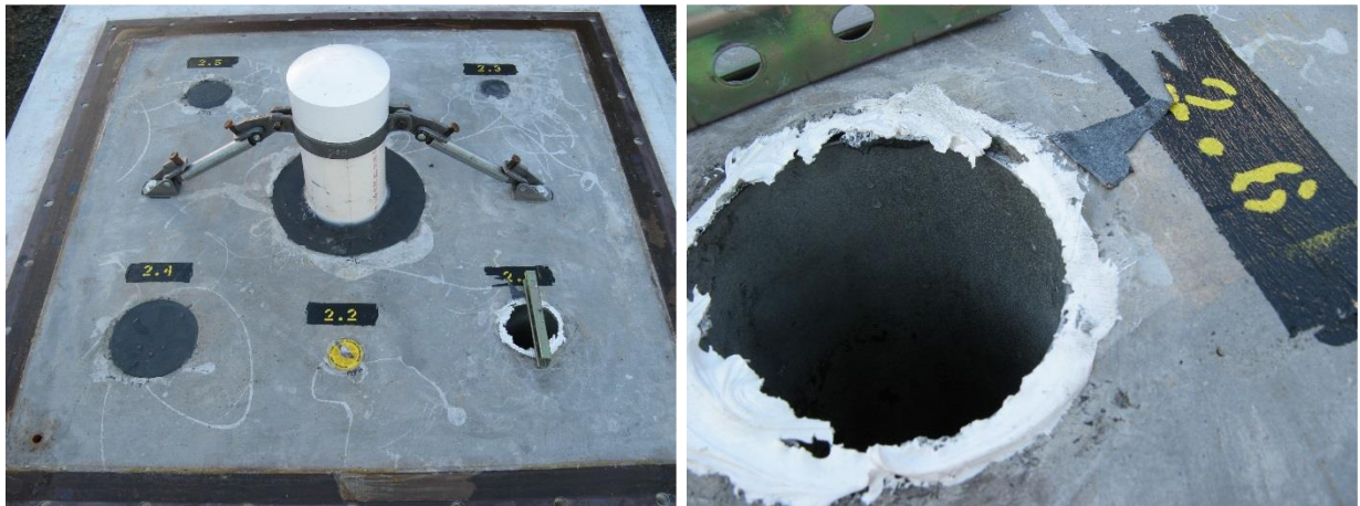
Figure 5-12 Test Deck 2 Post-Test (Left Photo) and Empty Sleeve (Right Photo) for Ejected Penetration 2.6
