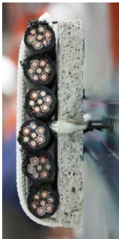
Fig. 18. Cable coupon constructed of seven conductor PE / PVC control cable (Cable 900). Side view.
