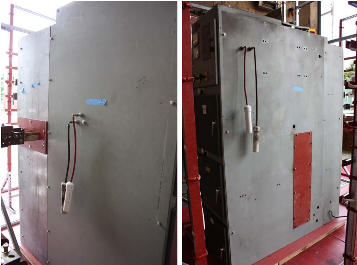
Fig. 15. Photos of pressure measurement locations (PT3 and PT4 (left); PT1 and PT2 (right)).
