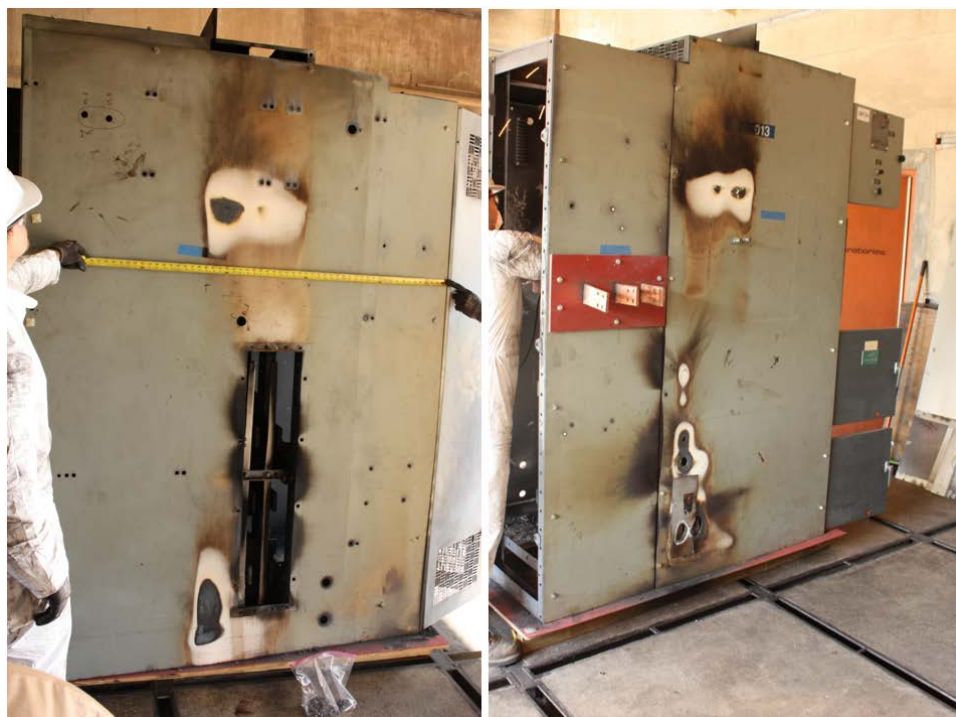
Fig. 75. Post-experiment image of enclosure. (load side (left), supply side (right)).
