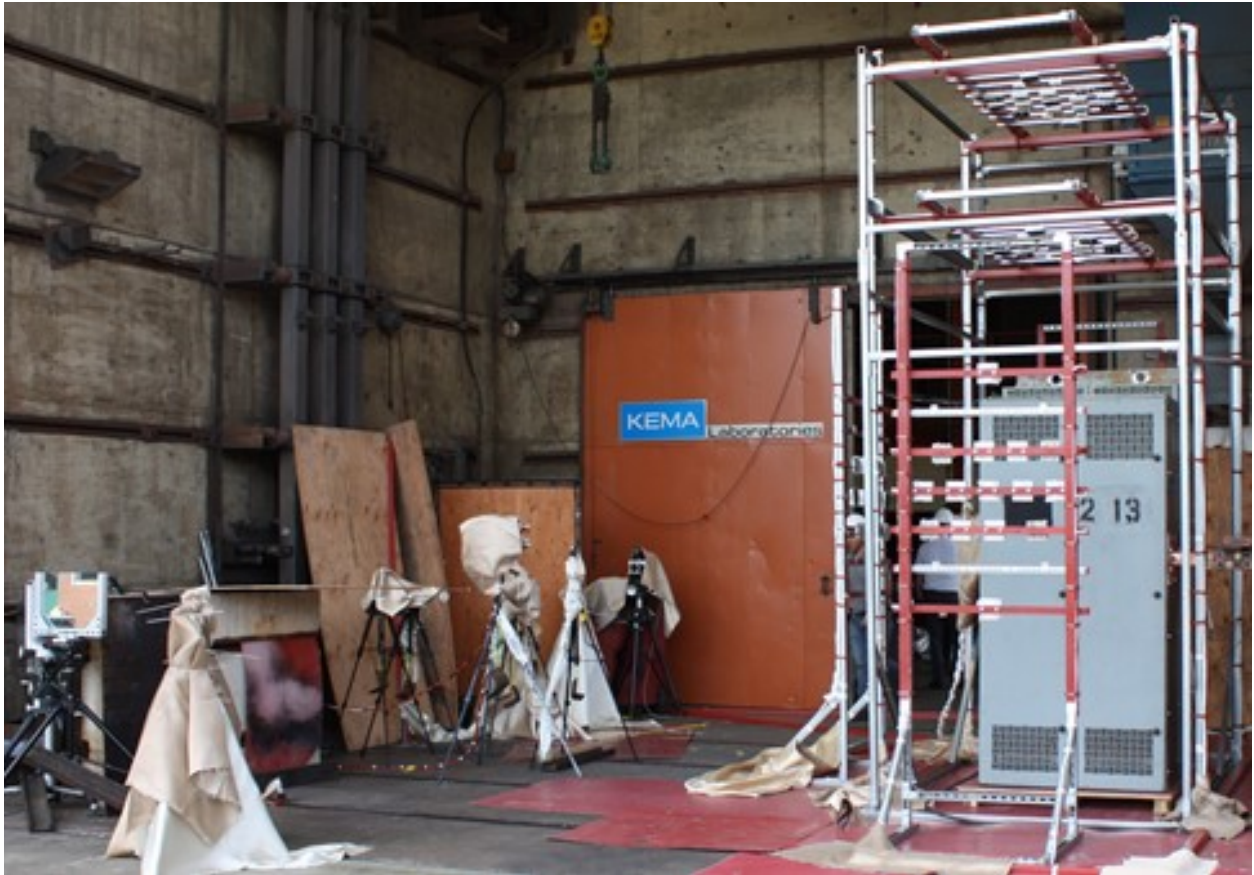
Fig. 7. Photograph of instrumentation cluster (from Left-to-right, air breakdown, radiometer, d-dot, air conductivity, high speed IR and visible videography)
