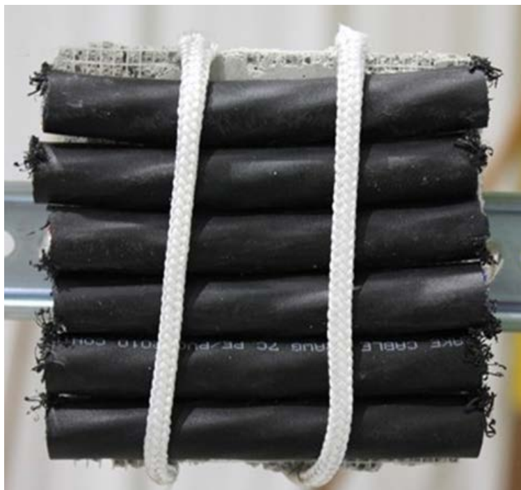
Fig. 17. Cable coupon constructed of seven conductor PE / PVC control cable (Cable 900). Front view.
