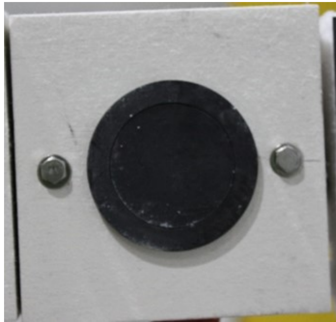
Fig. 12. Cross-section of ASTM Slug (top) nominal dimensions in millimeters, photo of device being prepared in the field (bottom). Note that the two bolts on each side of the device are used for mounting to the DIN rail of the instrumentation rack.
