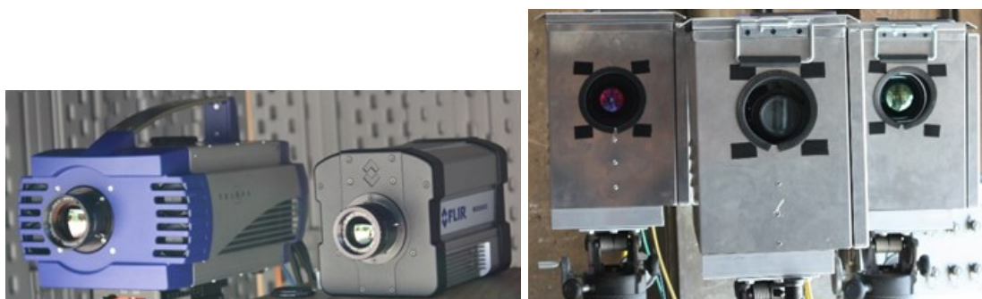
Fig. 8. Thermal imagers (NIST thermal imaging cameras located approximately 26.5 m from test device (let), SNL imaging cameras located approximately 27 m from test device (right), from left to right (thermal, high speed visible, thermal))
