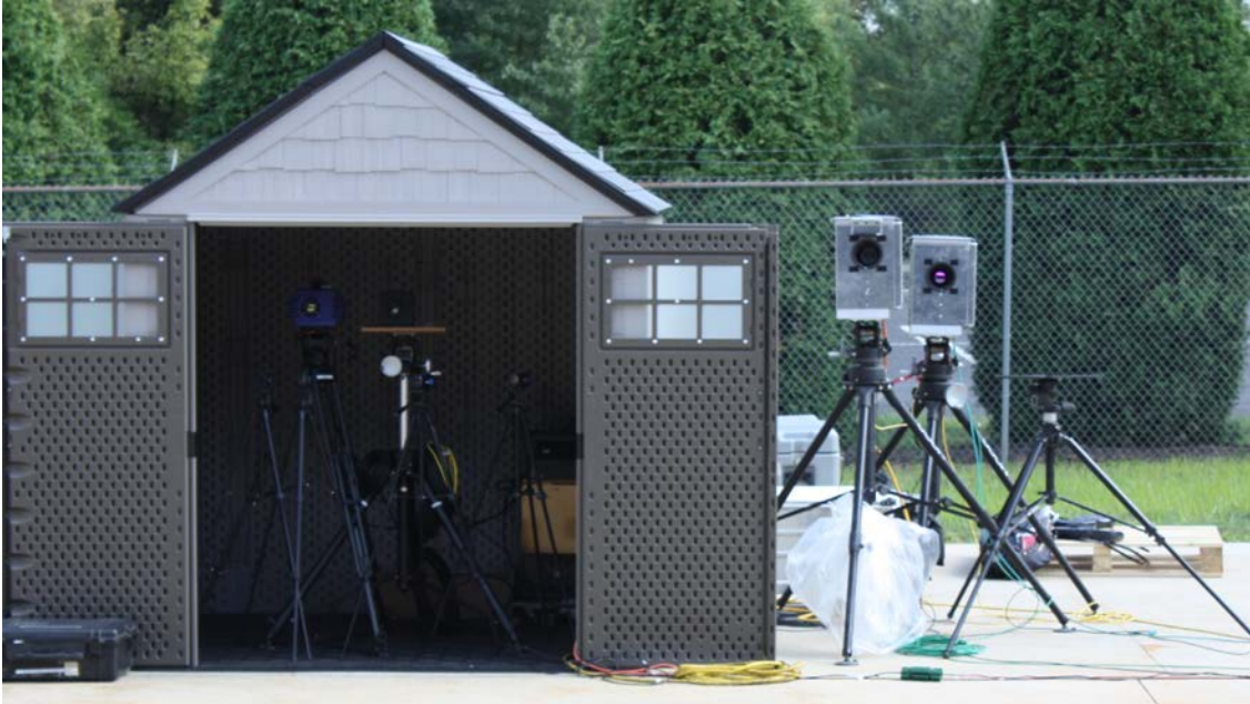
Fig. 9. Thermal imagers and high speed imagers are located in the courtyard. Four NIST cameras are in structure, approximately 26.5 m from the test device. Two SNL cameras are located outside the structure, approximately 27.0 m from the test device.
