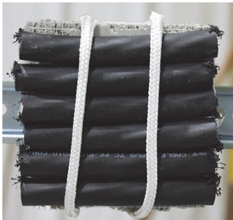
Fig. 22. Cable coupon constructed of seven conductor PE / PVC control cable (Cable 900). Front view.
