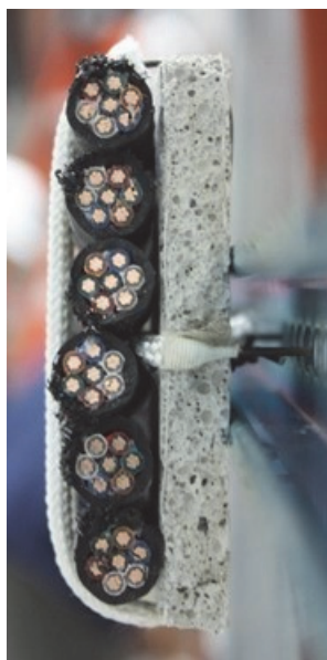
Fig. 109. Cable coupon constructed of seven conductor PE / PVC control cable (Cable 900). Side view.
