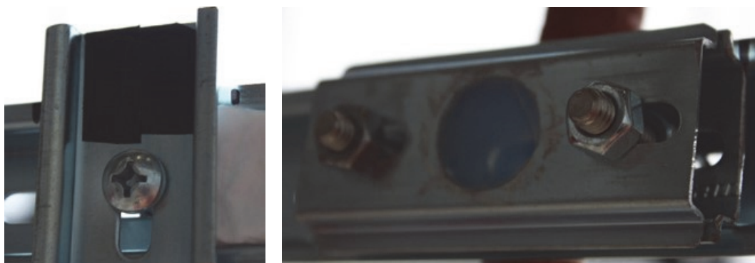
Fig. 19. Photo of carbon tape (left), and aerogel (right) particle collection apparatus
