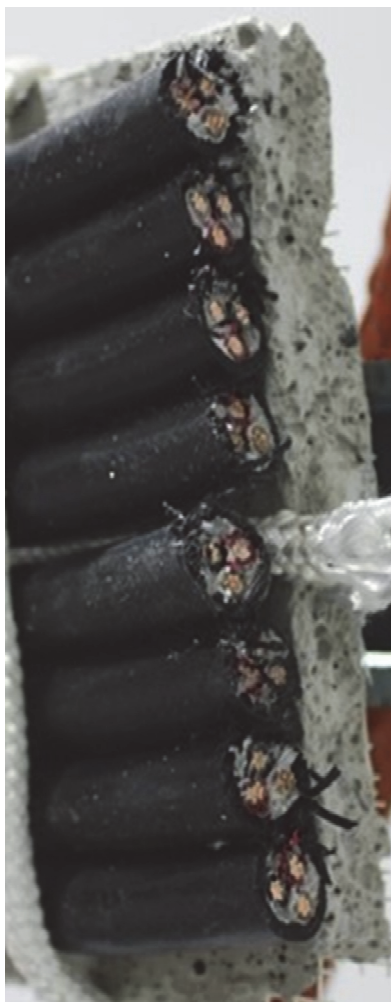
Fig. 111. Cable coupon constructed of three conductor PE / PVC control cable (Cable 902). Side view.
