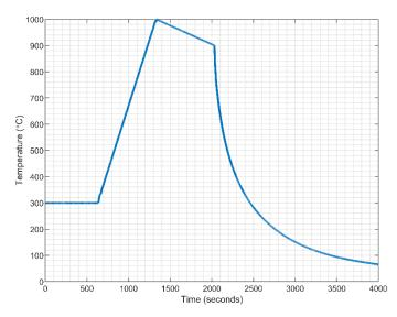
Figure 6. Example time and temperature transient for a tFGR test performed at Studsvik.
