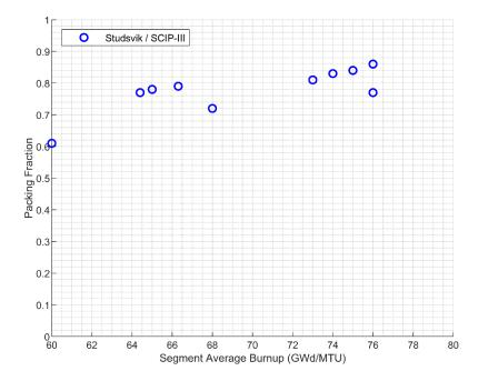
Figure 12. Average packing fraction in the lower portion of the balloon in the SCIP III tests (Magnusson, et al., 2020).
