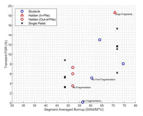
Figure 7. Measured tFGR as a function of burnup. Circle symbols represent out-of-pile LOCA tests (Magnusson, et al., 2020; Magnusson, et al., 2016; Tejland and Sheng, 2019a; Tejland and Sheng, 2019b; Bianco, et al., 2015). The triangle represents an in-pile LOCA test (Tradotti, 2014), and crosses represent single pellet-clad nonwelded samples (Pontillon, et al., 2004).
