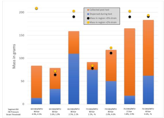
Figure A-10. Comparison of mass below 2-percent and 3-percent strain compared to mass dispersed and mobile.
