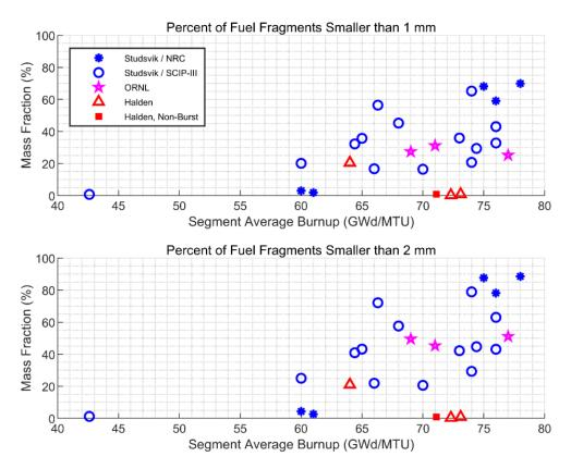
Figure 3. Measurements of percent of fuel fragments smaller than 1 mm.<sup>5</sup> and 2 mm as a function of burnup (Wiesenack, 2013; Wiesenack, 2015; NRC, 2013; Capps, et al., 2020; Magnusson, 2017; Magnusson and Sheng, 2017; Magnusson, 2018; Magnusson, et al., 2020; Mileshina and Magnusson, 2019a, b, c, d, e; Mileshina et al., 2019; König, 2021a, b, c).<sup>6</sup>.
