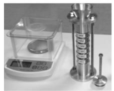
Figure 1. A sieve stack apparatus is used to examine fuel fragment size distribution in the programs referenced in this RIL. The image is of Halden's sieving apparatus used in the IFA-650 experiments (Wiesenack, 2015).
