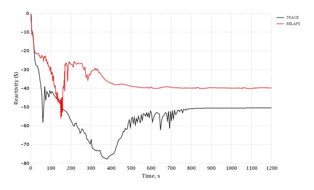
Figure 3-159 PRZ Surge Line Break. Core Reactivity
