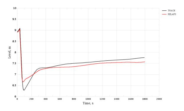
Figure 3-112 Uncontrolled Withdrawal of CR Group. Pressurizer Level
