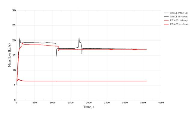
Figure 3-16 MSH Break. Make-Up and Let-Down Mass Flow Rate
