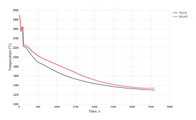
Figure 3-11 MSH Break. Coolant Temperature in Cold Leg, Loop 4
