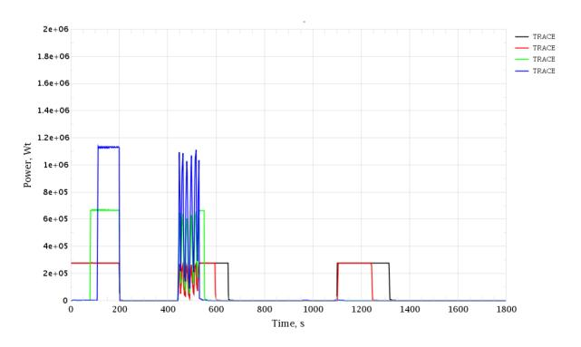
Figure 3-191 Inadvertent Opening of SG SRV in Hot Shutdown. PRZ Heaters Power
