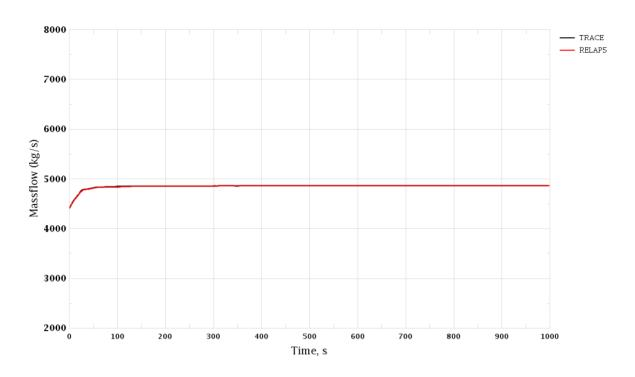
Figure 3-86 Trip of One RCP. RCS Loop 2 Mass Flow Rate
