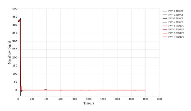
Figure 3-136 Uncontrolled Withdrawal of CR Group. Mass Flow through MSIV
