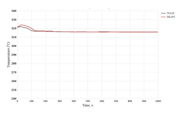
Figure 3-79 Trip of One RCP. Coolant Temperature in Hot Leg, Loop 3
