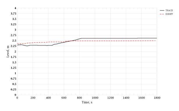
Figure 3-199 Inadvertent Opening of SG SRV in Hot Shutdown. SG-4 Level (Wide Range)
