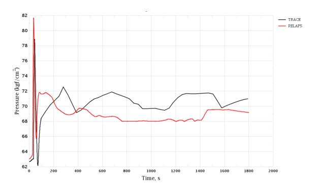
Figure 3-128 Uncontrolled Withdrawal of CR Group. SG-1 Pressure
