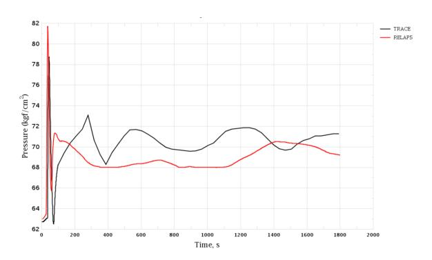
Figure 3-129 Uncontrolled Withdrawal of CR Group. SG-2 Pressure
