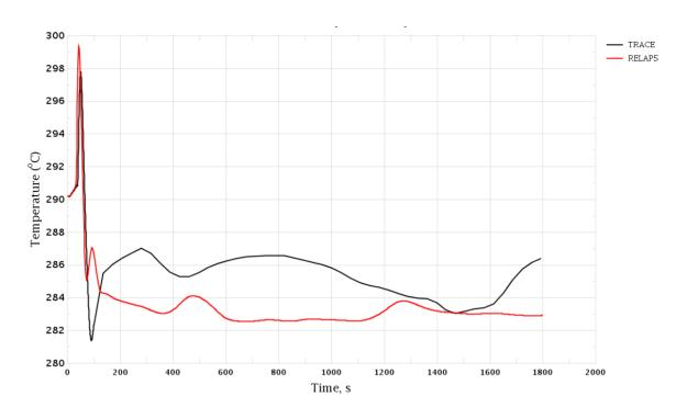
Figure 3-120 Uncontrolled Withdrawal of CR Group. Coolant Temperature in Cold Leg, Loop 4
