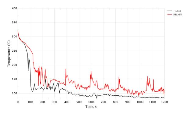
Figure 3-147 PRZ Surge Line Break. Coolant Temperature in Hot Leg, Loop 3
