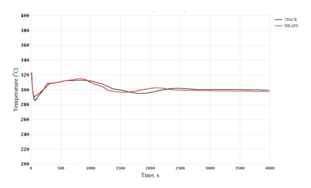
Figure 3-44 Loss of Turbine Condenser Vacuum. Coolant Temperature in Hot Leg, Loop 4
