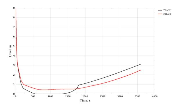
Figure 3-3 MSH Break. Pressurizer Level
