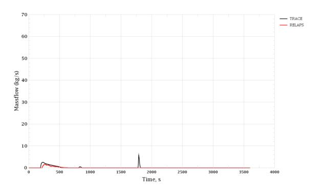
Figure 3-32 MSH Break. HPIS-1 Mass Flow Rate
