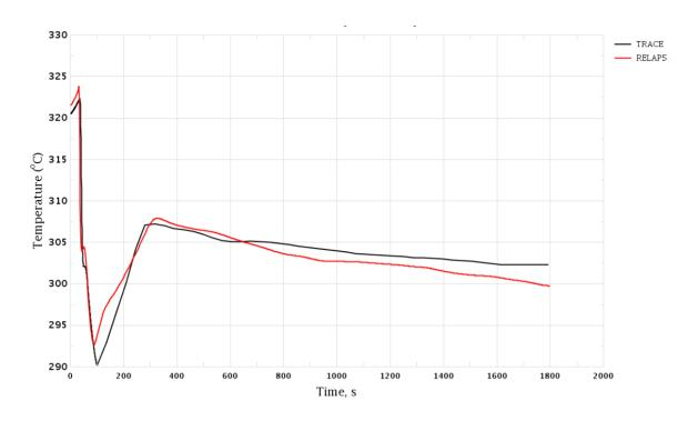
Figure 3-114 Uncontrolled Withdrawal of CR Group. Coolant Temperature in Hot Leg, Loop 2
