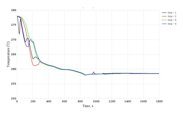
Figure 3-188 Inadvertent Opening of SG SRV in Hot Shutdown. Coolant Temperature in Cold Legs
