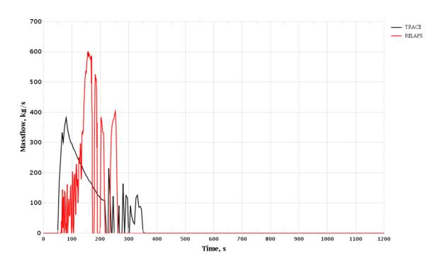
Figure 3-180 PRZ Surge Line Break. HA-4 Mass Flow Rate
