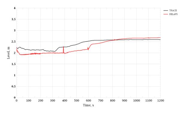
Figure 3-167 PRZ Surge Line Break. SG-4 Level (Wide Range)
