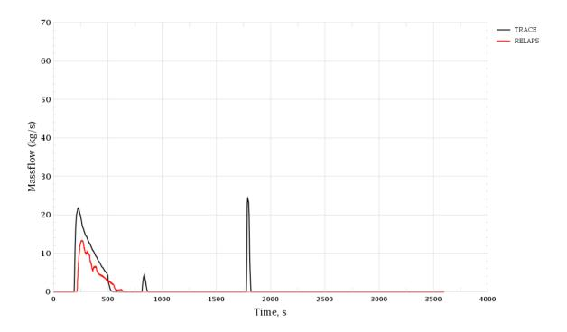
Figure 3-34 MSH Break. HPIS-3 Mass Flow Rate
