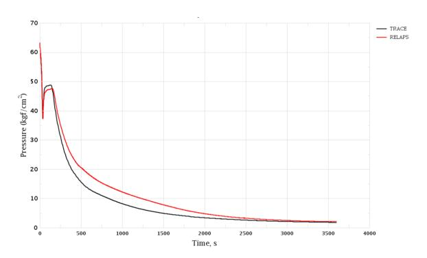
Figure 3-22 MSH Break. SG-4 Pressure
