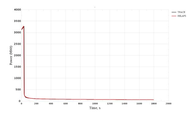
Figure 3-110 Uncontrolled Withdrawal of CR Group. Core Thermal Power
