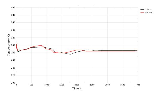
Figure 3-48 Loss of Turbine Condenser Vacuum. Coolant Temperature in Cold Leg, Loop 4
