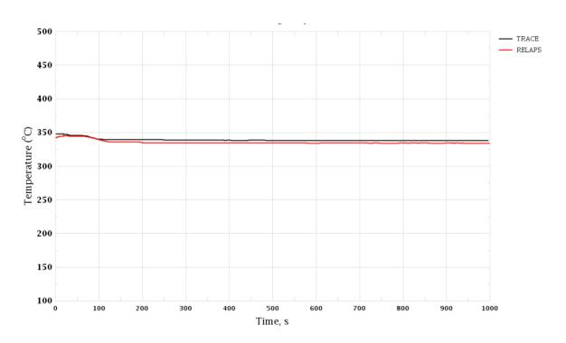
Figure 3-109 Trip of One RCP. Maximal Cladding Temperature
