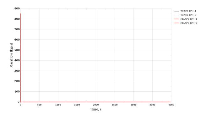
Figure 3-70 Loss of Turbine Condenser Vacuum. MFW Mass Flow Rate
