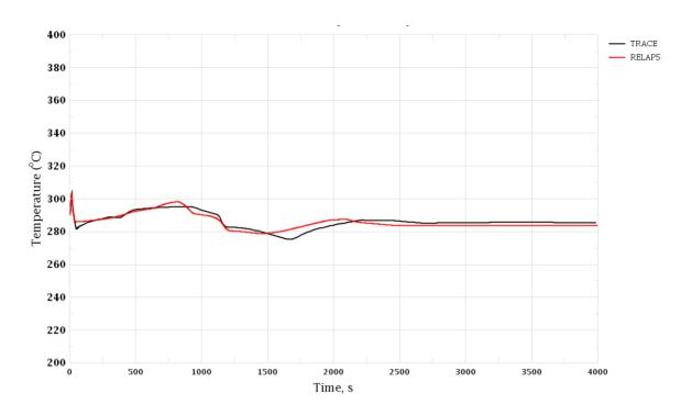
Figure 3-47 Loss of Turbine Condenser Vacuum. Coolant Temperature in Cold Leg, Loop 3
