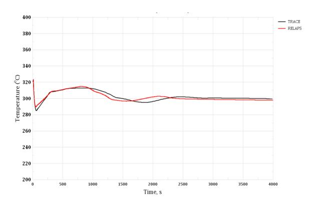
Figure 3-43 Loss of Turbine Condenser Vacuum. Coolant Temperature in Hot Leg, Loop 3
