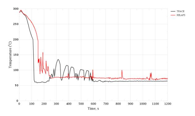
Figure 3-150 PRZ Surge Line Break. Coolant Temperature in Cold Leg, Loop 2
