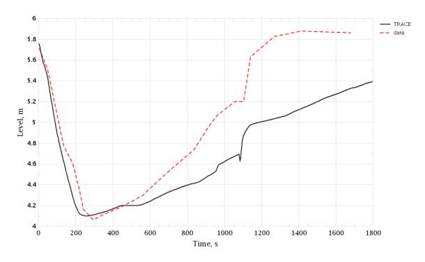
Figure 3-186 Inadvertent Opening of SG SRV in Hot Shutdown. Pressurizer Level
