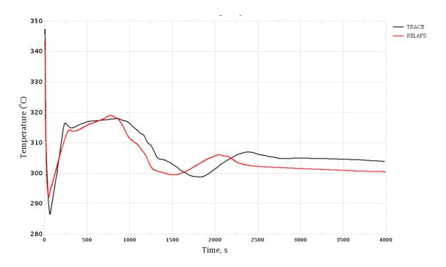
Figure 3-73 Loss of Turbine Condenser Vacuum. Maximal Cladding Temperature
