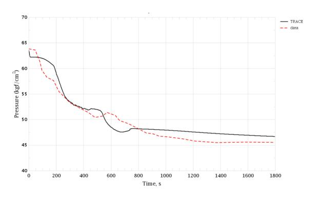
Figure 3-193 Inadvertent Opening of SG SRV in Hot Shutdown. SG-2 Pressure
