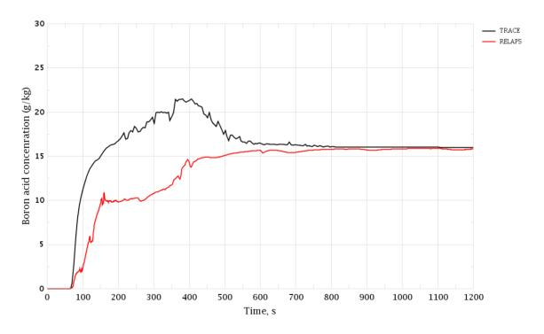
Figure 3-183 PRZ Surge Line Break. Boric Acid Concentration in the Core
