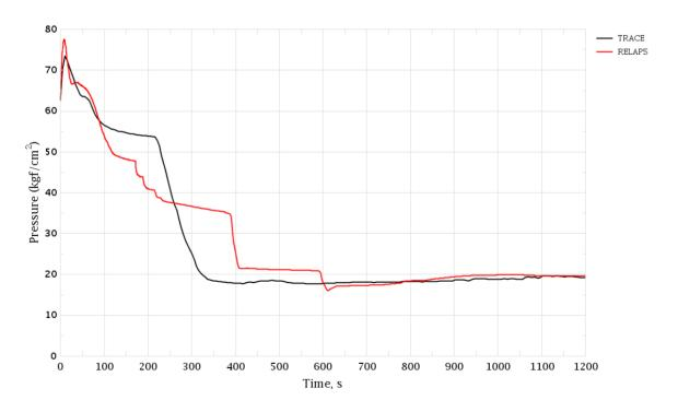
Figure 3-163 PRZ Surge Line Break. SG-4 Pressure
