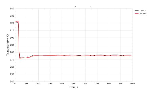
Figure 3-77 Trip of One RCP. Coolant Temperature in Hot Leg, Loop 1
