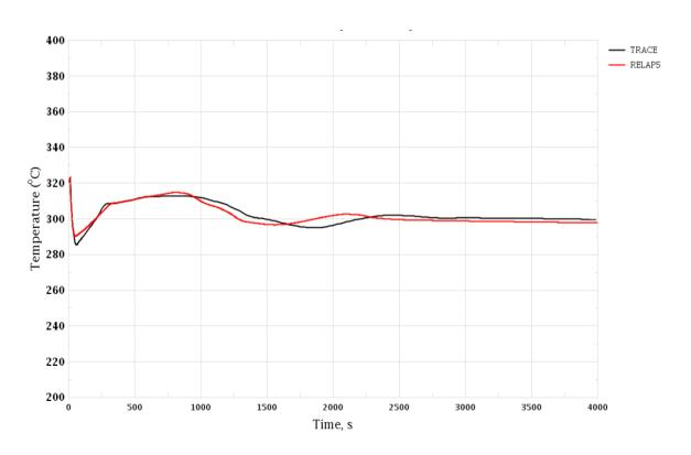
Figure 3-41 Loss of Turbine Condenser Vacuum. Coolant Temperature in Hot Leg, Loop 1
