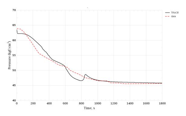
Figure 3-194 Inadvertent Opening of SG SRV in Hot Shutdown. SG-3 Pressure
