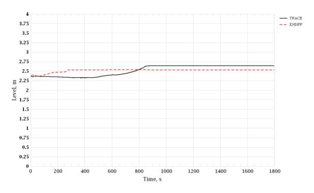
Figure 3-198 Inadvertent Opening of SG SRV in Hot Shutdown. SG-3 Level (Wide Range)
