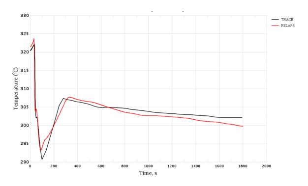
Figure 3-116 Uncontrolled Withdrawal of CR Group. Coolant Temperature in Hot Leg, Loop 4
