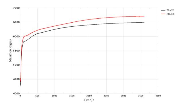
Figure 3-12 MSH Break. RCS Loop 1 Mass Flow Rate
