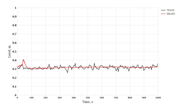
Figure 3-104 Trip of One RCP. SG-4 Level (Narrow Range)
