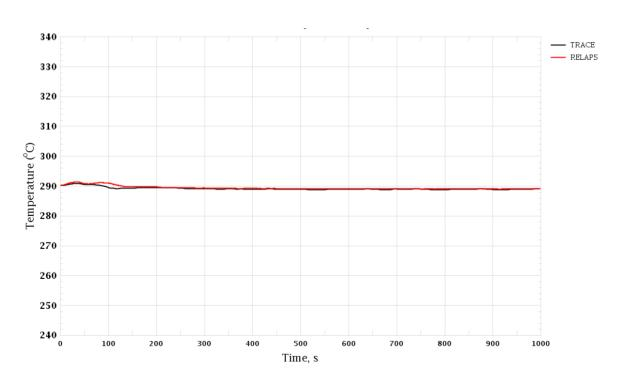
Figure 3-83 Trip of One RCP. Coolant Temperature in Cold Leg, Loop 3
