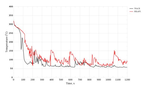
Figure 3-145 PRZ Surge Line Break. Coolant Temperature in Hot Leg, Loop 1
