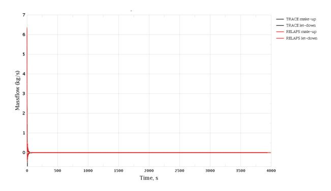
Figure 3-53 Loss of Turbine Condenser Vacuum. Make-Up and Let-Down Mass Flow
