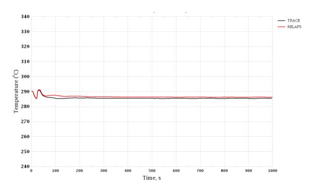
Figure 3-81 Trip of One RCP. Coolant Temperature in Cold Leg, Loop 1
