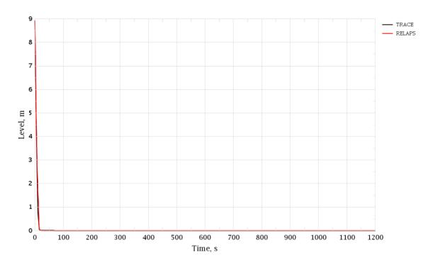
Figure 3-144 PRZ Surge Line Break. Pressurizer Level
