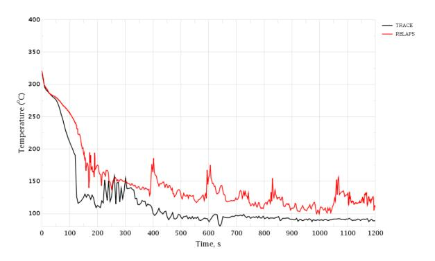
Figure 3-146 PRZ Surge Line Break. Coolant Temperature in Hot Leg, Loop 2
