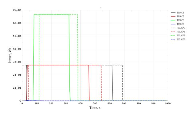
Figure 3-90 Trip of One RCP. PRZ Heaters Power
