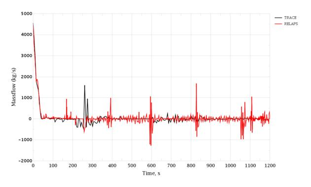
Figure 3-155 PRZ Surge Line Break. RCS Loop 3 Mass Flow Rate
