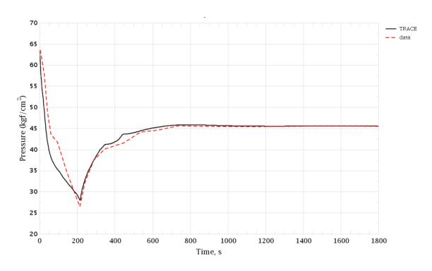
Figure 3-192 Inadvertent Opening of SG SRV in Hot Shutdown. SG-1 Pressure
