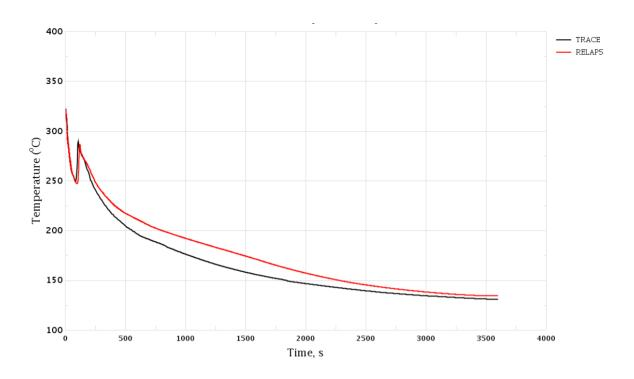
Figure 3-7 MSH Break. Coolant Temperature in Hot Leg, Loop 4
