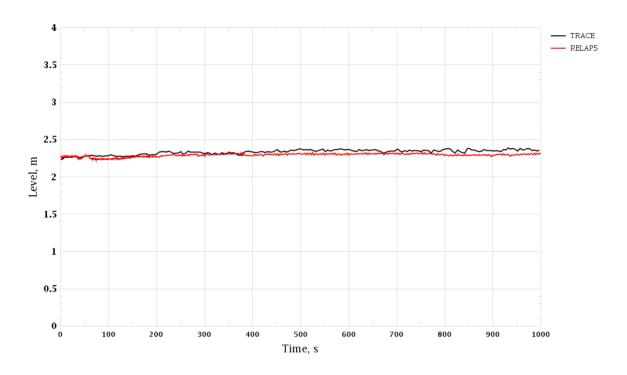
Figure 3-100 Trip of One RCP. SG-4 Level (Wide Range)
