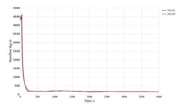
Figure 3-52 Loss of Turbine Condenser Vacuum. RCS Loop 4 Mass Flow Rate
