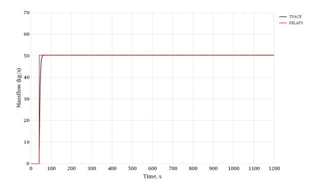
Figure 3-171 PRZ Surge Line Break. HPIS-1 Mass Flow Rate
