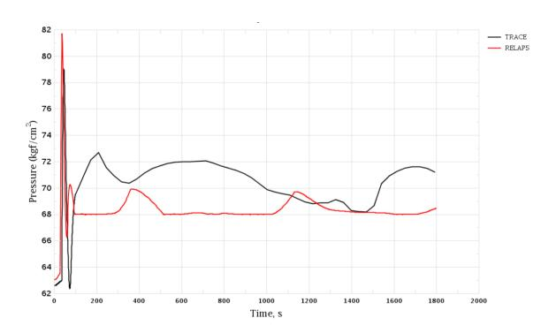
Figure 3-131 Uncontrolled Withdrawal of CR Group. SG-4 Pressure
