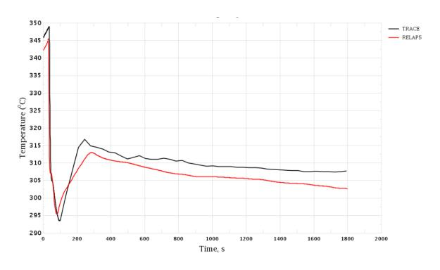
Figure 3-141 Uncontrolled Withdrawal of CR Group. Maximal Cladding Temperature
