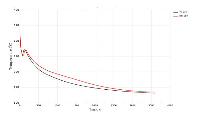
Figure 3-5 MSH Break. Coolant Temperature in Hot Leg, Loop 2
