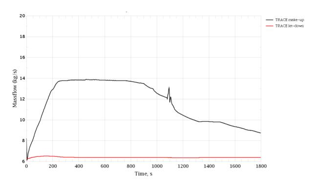
Figure 3-190 Inadvertent Opening of SG SRV in Hot Shutdown. Make-Up and Let-Down Mass Flow
