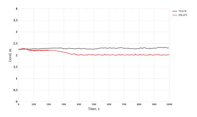
Figure 3-98 Trip of One RCP. SG-2 Level (Wide Range)
