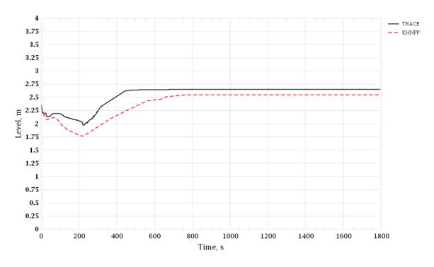
Figure 3-196 Inadvertent Opening of SG SRV in Hot Shutdown. SG-1 Level (Wide Range)
