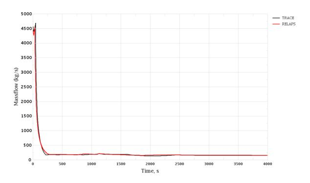
Figure 3-51 Loss of Turbine Condenser Vacuum. RCS Loop 3 Mass Flow Rate
