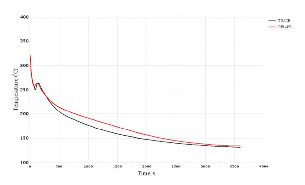
Figure 3-6 MSH Break. Coolant Temperature in Hot Leg, Loop 3
