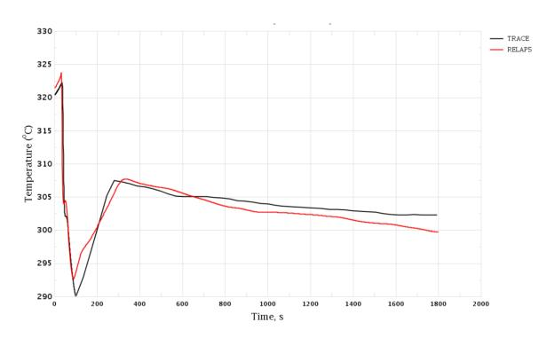
Figure 3-115 Uncontrolled Withdrawal of CR Group. Coolant Temperature in Hot Leg, Loop 3
