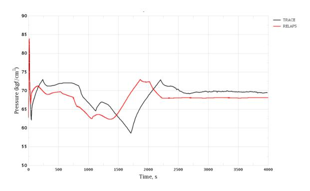
Figure 3-58 Loss of Turbine Condenser Vacuum. SG-2 Pressure
