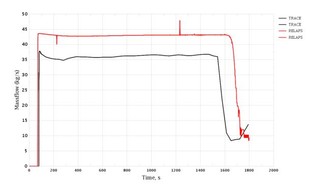
Figure 3-140 Uncontrolled Withdrawal of CR Group. AFW Mass Flow Rate
