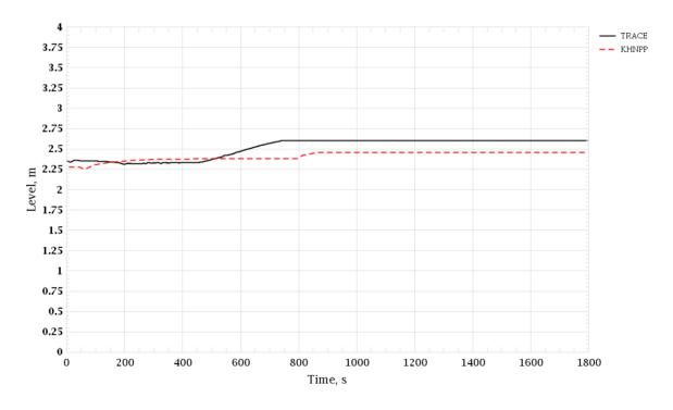
Figure 3-197 Inadvertent Opening of SG SRV in Hot Shutdown. SG-2 Level (Wide Range)
