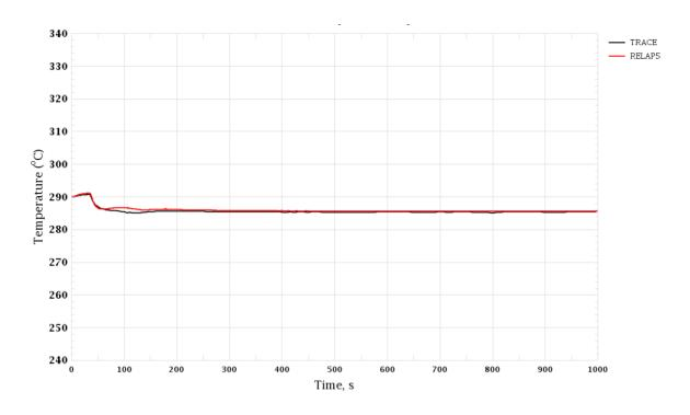
Figure 3-84 Trip of One RCP. Coolant Temperature in Cold Leg, Loop 4
