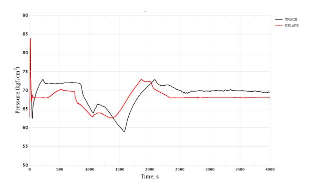
Figure 3-59 Loss of Turbine Condenser Vacuum. SG-3 Pressure
