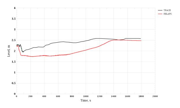
Figure 3-132 Uncontrolled Withdrawal of CR Group. SG-1 Level (Wide Range)
