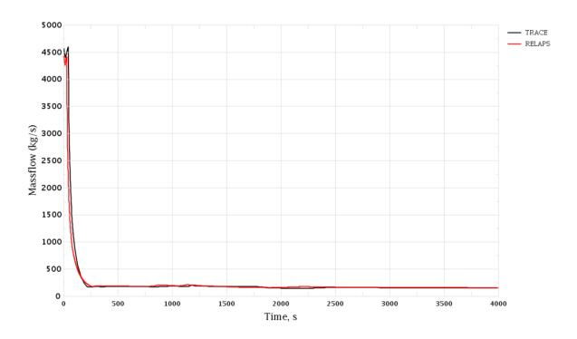
Figure 3-50 Loss of Turbine Condenser Vacuum. RCS Loop 2 Mass Flow Rate
