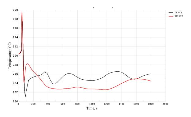
Figure 3-118 Uncontrolled Withdrawal of CR Group. Coolant Temperature in Cold Leg, Loop 2
