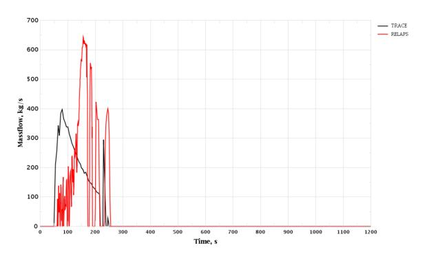
Figure 3-178 PRZ Surge Line Break. HA-2 Mass Flow Rate
