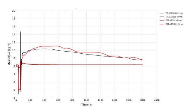
Figure 3-125 Uncontrolled Withdrawal of CR Group. Make-Up and Let-Down Mass Flow
