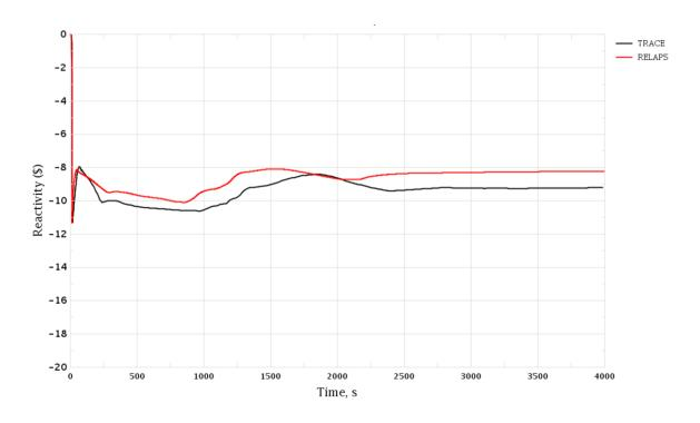
Figure 3-56 Loss of Turbine Condenser Vacuum. Core Reactivity
