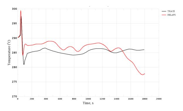
Figure 3-119 Uncontrolled Withdrawal of CR Group. Coolant Temperature in Cold Leg, Loop 3
