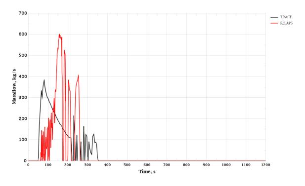
Figure 3-179 PRZ Surge Line Break. HA-3 Mass Flow Rate
