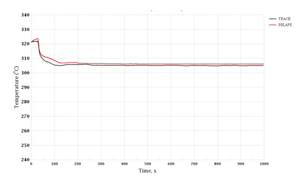
Figure 3-80 Trip of One RCP. Coolant Temperature in Hot Leg, Loop 4
