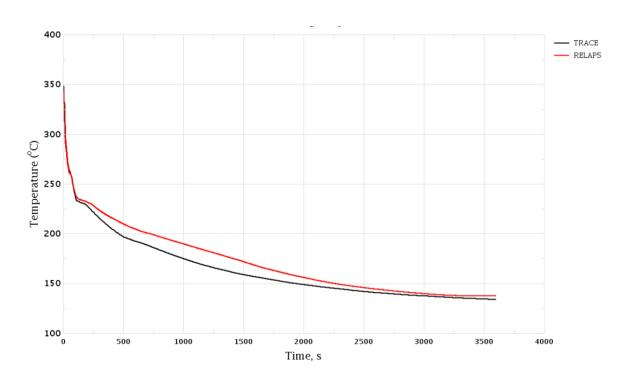
Figure 3-36 MSH Break. Maximal Cladding Temperature
