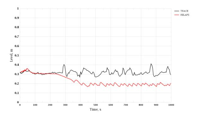
Figure 3-103 Trip of One RCP. SG-3 Level (Narrow Range)
