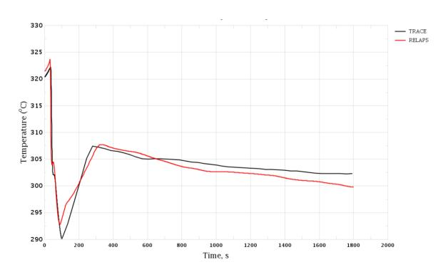
Figure 3-113 Uncontrolled Withdrawal of CR Group. Coolant Temperature in Hot Leg, Loop 1
