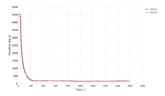
Figure 3-123 Uncontrolled Withdrawal of CR Group. RCS Loop 3 Mass Flow Rate
