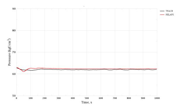
Figure 3-94 Trip of One RCP. SG-2 Pressure
