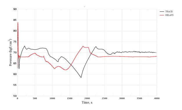
Figure 3-57 Loss of Turbine Condenser Vacuum. SG-1 Pressure
