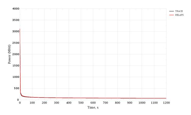
Figure 3-142 PRZ Surge Line Break. Core Thermal Power
