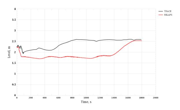
Figure 3-133 Uncontrolled Withdrawal of CR Group. SG-2 Level (Wide Range)
