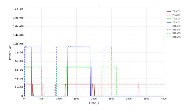
Figure 3-54 Loss of Turbine Condenser Vacuum. PRZ Heaters Power
