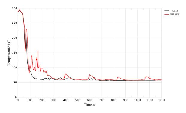
Figure 3-149 PRZ Surge Line Break. Coolant Temperature in Cold Leg, Loop 1
