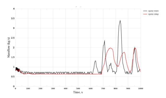
Figure 3-91 Trip of One RCP. PRZ Spray Mass Flow Rate
