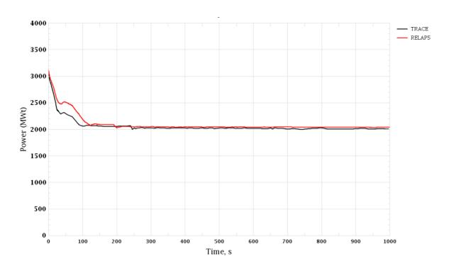
Figure 3-74 Trip of One RCP. Core Thermal Power
