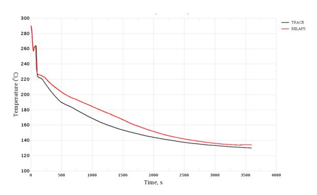
Figure 3-10 MSH Break. Coolant Temperature in Cold Leg, Loop 3
