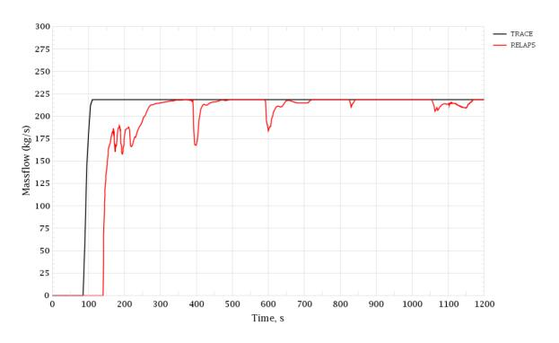
Figure 3-176 PRZ Surge Line Break. LPIS-3 Mass Flow Rate
