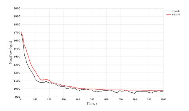
Figure 3-106 Trip of One RCP. Turbine Mass Flow Rate
