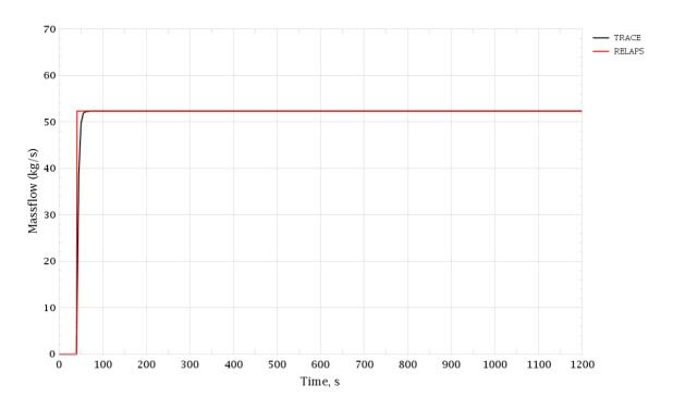
Figure 3-172 PRZ Surge Line Break. HPIS-2 Mass Flow Rate
