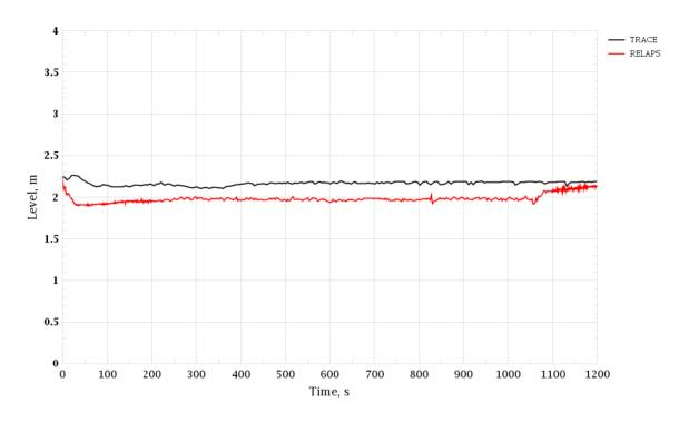
Figure 3-164 PRZ Surge Line Break. SG-1 Level (Wide Range)
