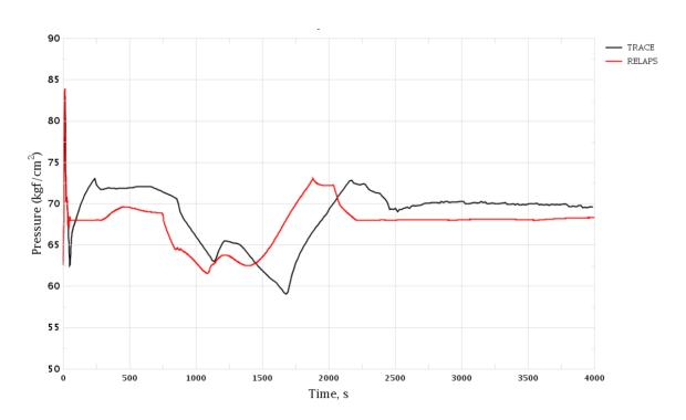
Figure 3-60 Loss of Turbine Condenser Vacuum. SG-4 Pressure
