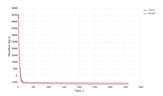
Figure 3-14 MSH Break. RCS Loop 3 Mass Flow Rate
