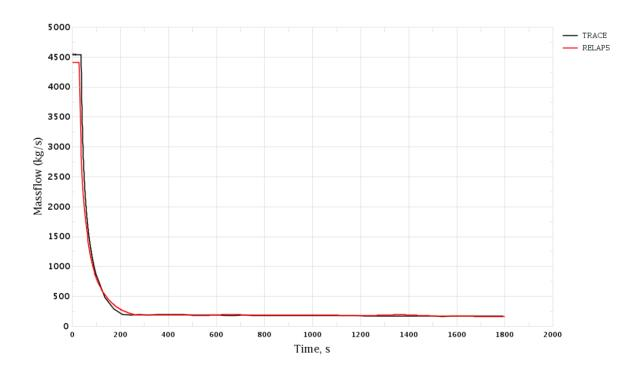
Figure 3-121 Uncontrolled Withdrawal of CR Group. RCS Loop 1 Mass Flow Rate
