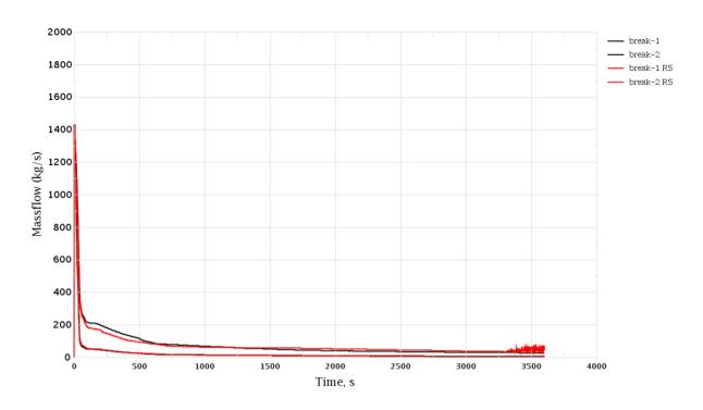
Figure 3-35 MSH Break. Break Mass Flow Rate
