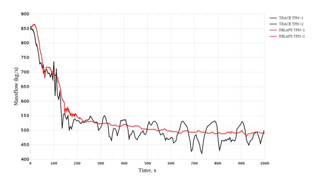
Figure 3-107 Trip of One RCP. MFW Pumps Mass Flow Rate
