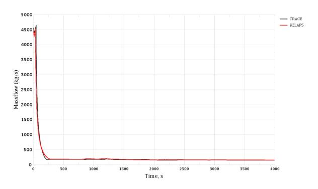
Figure 3-49 Loss of Turbine Condenser Vacuum. RCS Loop 1 Mass Flow Rate
