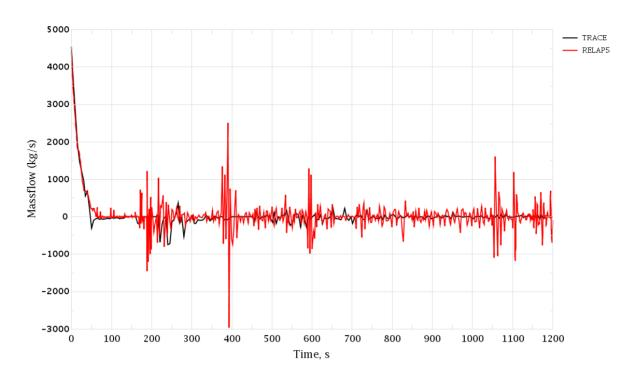
Figure 3-156 PRZ Surge Line Break. RCS Loop 4 Mass Flow Rate
