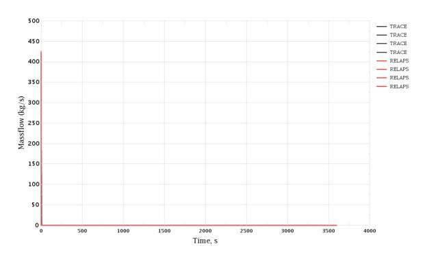
Figure 3-27 MSH Break. Turbine Mass Flow Rate
