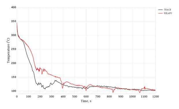
Figure 3-181 PRZ Surge Line Break. Maximal Cladding Temperature
