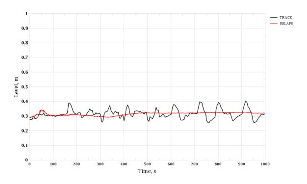
Figure 3-102 Trip of One RCP. SG-2 Level (Narrow Range)
