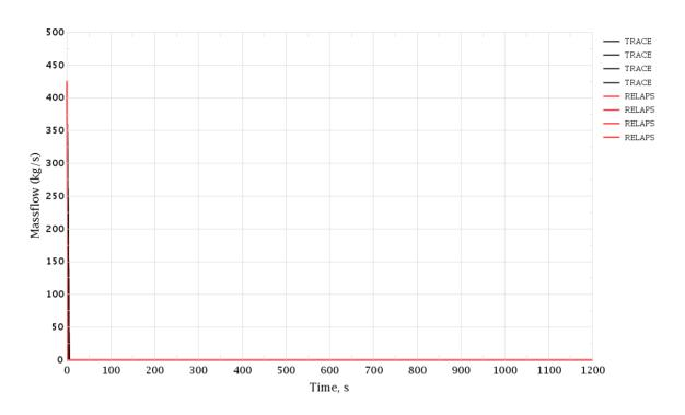
Figure 3-168 PRZ Surge Line Break. Turbines Mass Flow Rate
