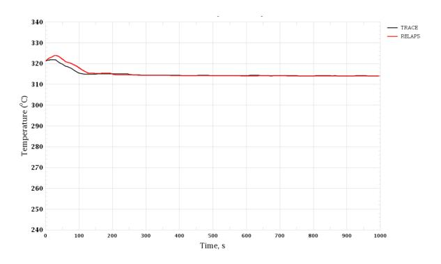
Figure 3-78 Trip of One RCP. Coolant Temperature in Hot Leg, Loop 2
