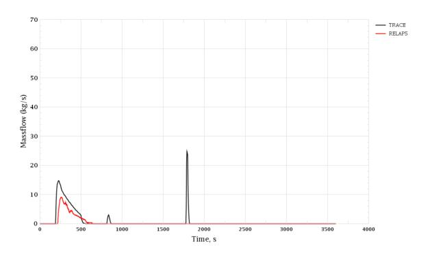
Figure 3-33 MSH Break. HPIS-2 Mass Flow Rate
