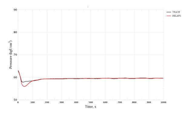
Figure 3-93 Trip of One RCP. SG-1 Pressure
