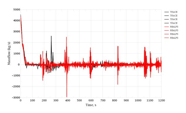
Figure 3-170 PRZ Surge Line Break. MFW Pumps Mass Flow Rate
