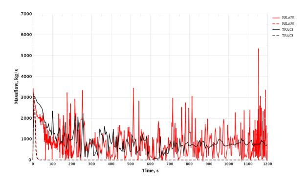
Figure 3-182 PRZ Surge Line Break. Break Mass Flow Rate
