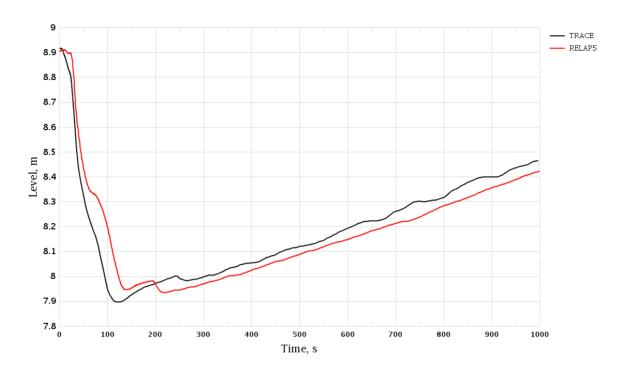
Figure 3-76 Trip of One RCP. Pressurizer Level
