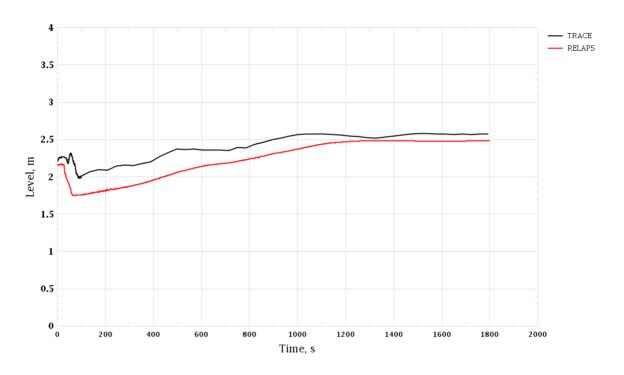
Figure 3-134 Uncontrolled Withdrawal of CR Group. SG-3 Level (Wide Range)
