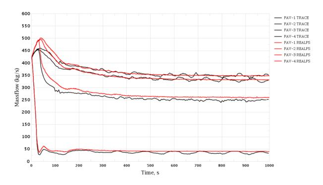
Figure 3-105 Trip of One RCP. Mass Flow through MSIV
