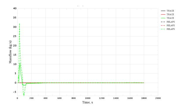
Figure 3-127 Uncontrolled Withdrawal of CR Group. PRZ Spray Mass Flow Rate
