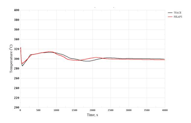
Figure 3-42 Loss of Turbine Condenser Vacuum. Coolant Temperature in Hot Leg, Loop 2
