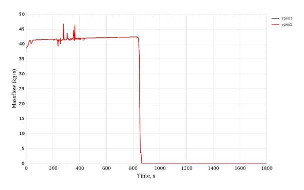
Figure 3-200 Inadvertent Opening of SG SRV in Hot Shutdown. AFW Mass Flow Rate
