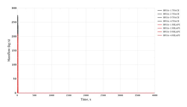
Figure 3-69 Loss of Turbine Condenser Vacuum. SG SRV Steam Mass Flow Rate
