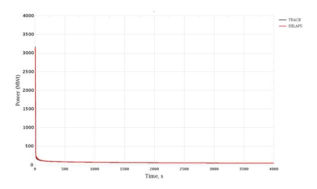
Figure 3-38 Loss of Turbine Condenser Vacuum. Core Thermal Power
