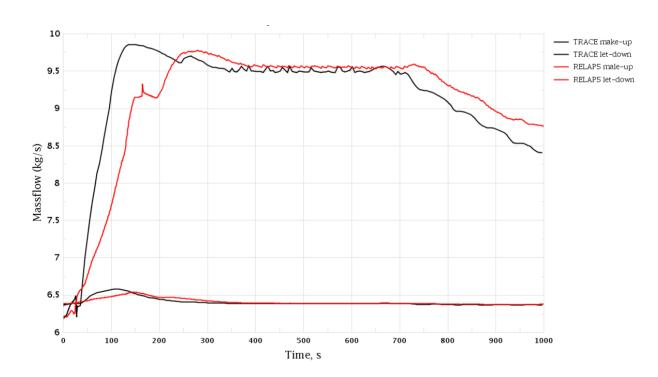
Figure 3-89 Trip of One RCP. Make-Up and Let-Down Mass Flow
