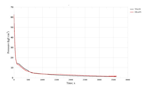
Figure 3-19 MSH Break. SG-1 Pressure
