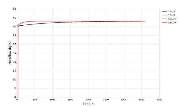
Figure 3-30 MSH Break. AFW Pumps Mass Flow Rate
