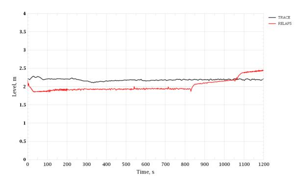
Figure 3-166 PRZ Surge Line Break. SG-3 Level (Wide Range)
