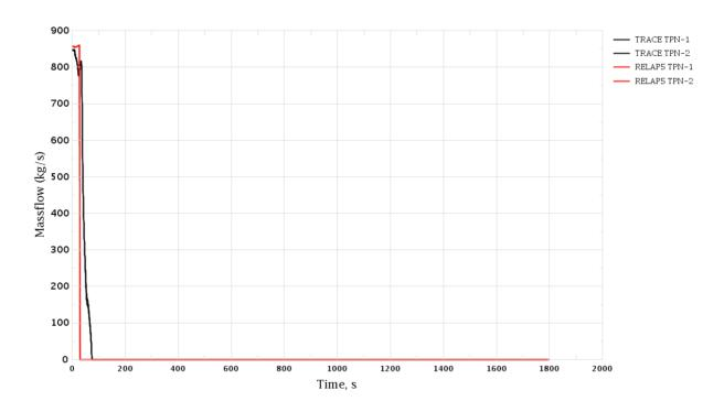
Figure 3-139 Uncontrolled Withdrawal of CR Group. MFW Pumps Mass Flow Rate
