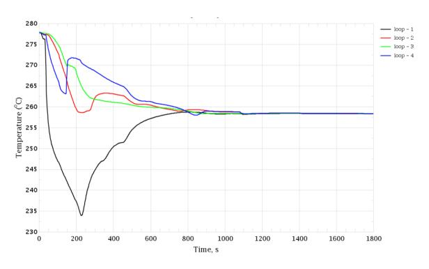
Figure 3-187 Inadvertent Opening of SG SRV in Hot Shutdown. Coolant Temperature in Hot Legs
