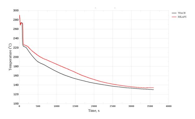
Figure 3-9 MSH Break. Coolant Temperature in Cold Leg, Loop 2
