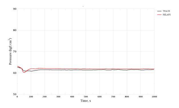
Figure 3-96 Trip of One RCP. SG-4 Pressure
