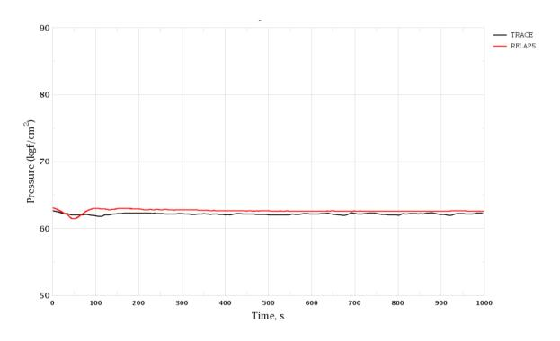
Figure 3-95 Trip of One RCP. SG-3 Pressure
