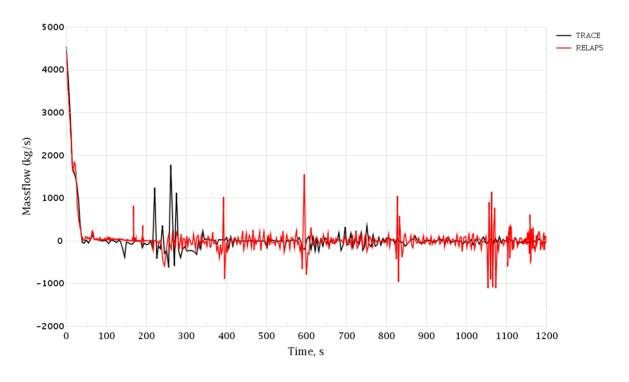
Figure 3-153 PRZ Surge Line Break. RCS Loop 1 Mass Flow Rate
