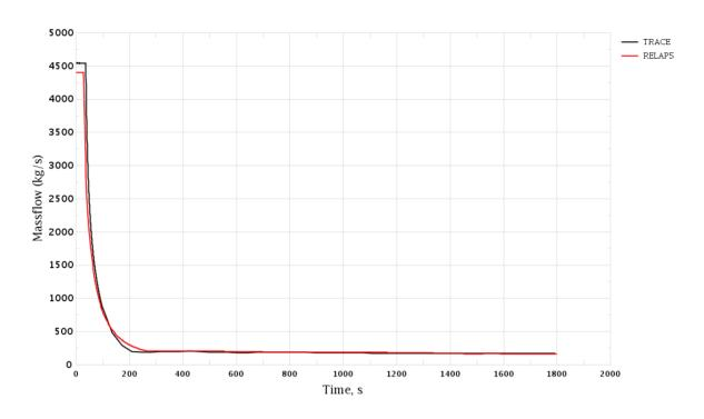
Figure 3-122 Uncontrolled Withdrawal of CR Group. RCS Loop 2 Mass Flow Rate
