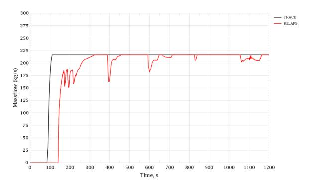
Figure 3-175 PRZ Surge Line Break. LPIS-2 Mass Flow Rate
