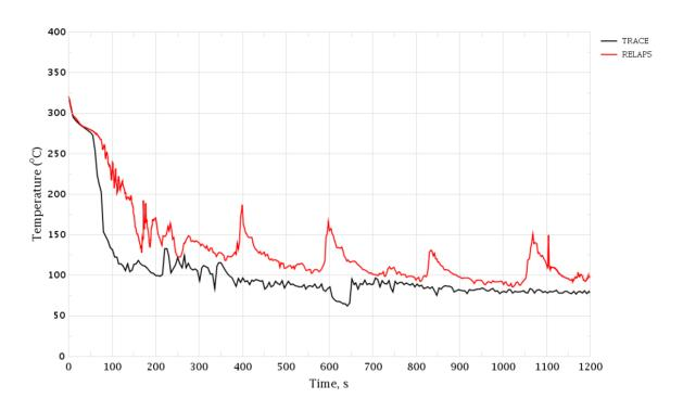
Figure 3-148 PRZ Surge Line Break. Coolant Temperature in Hot Leg, Loop 4
