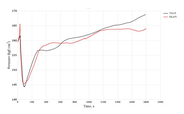
Figure 3-111 Uncontrolled Withdrawal of CR Group. RCS Pressure
