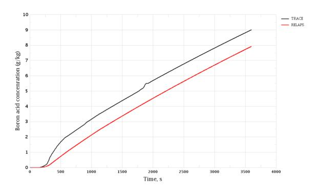
Figure 3-37 MSH Break. Boric Acid Concentration in the Core
