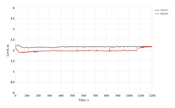
Figure 3-165 PRZ Surge Line Break. SG-2 Level (Wide Range)
