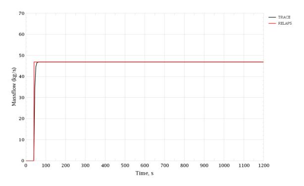
Figure 3-173 PRZ Surge Line Break. HPIS-3 Mass Flow Rate
