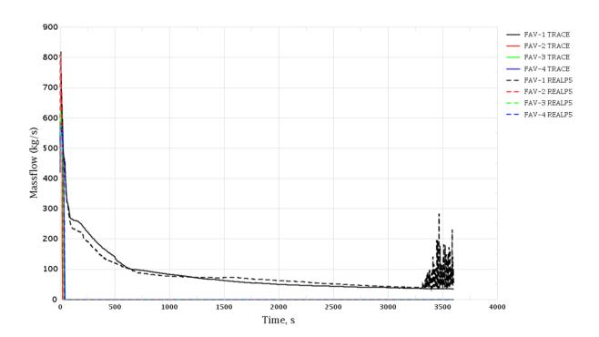
Figure 3-28 MSH Break. Mass Flow through MSIV
