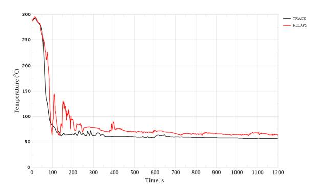
Figure 3-152 PRZ Surge Line Break. Coolant Temperature in Cold Leg, Loop 4
