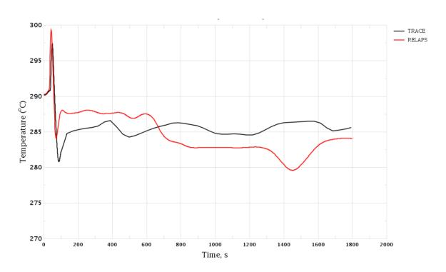
Figure 3-117 Uncontrolled Withdrawal of CR Group. Coolant Temperature in Cold Leg, Loop 1
