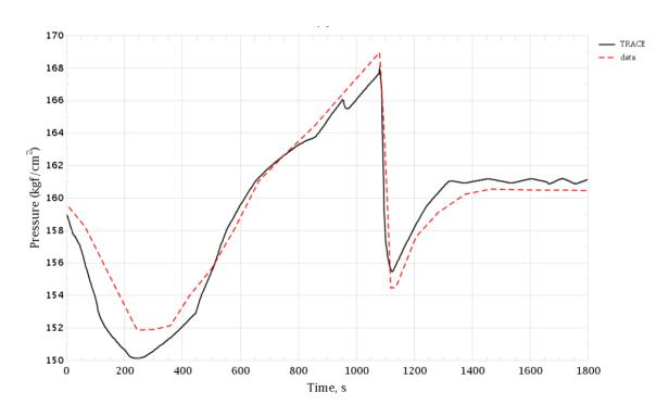
Figure 3-185 Inadvertent Opening of SG SRV in Hot Shutdown. RCS Pressure
