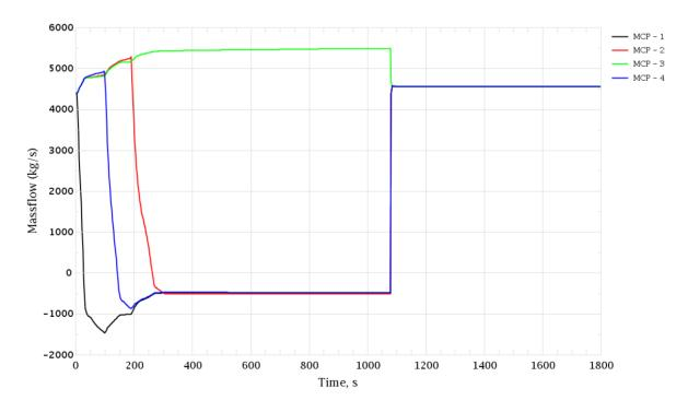
Figure 3-189 Inadvertent Opening of SG SRV in Hot Shutdown. RCS Loops Mass Flow Rate
