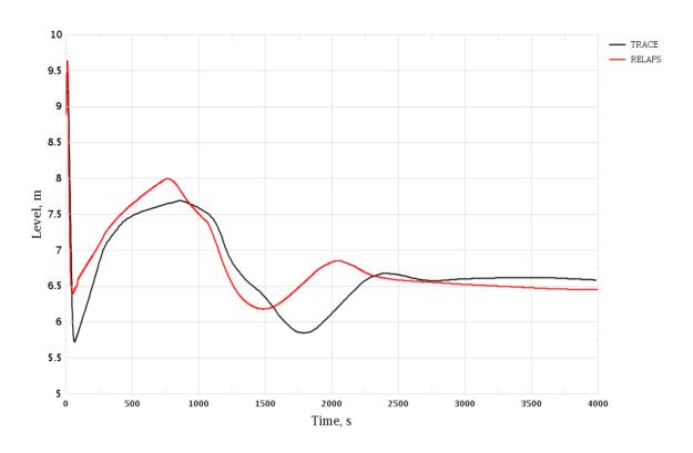
Figure 3-40 Loss of Turbine Condenser Vacuum. Pressurizer Level
