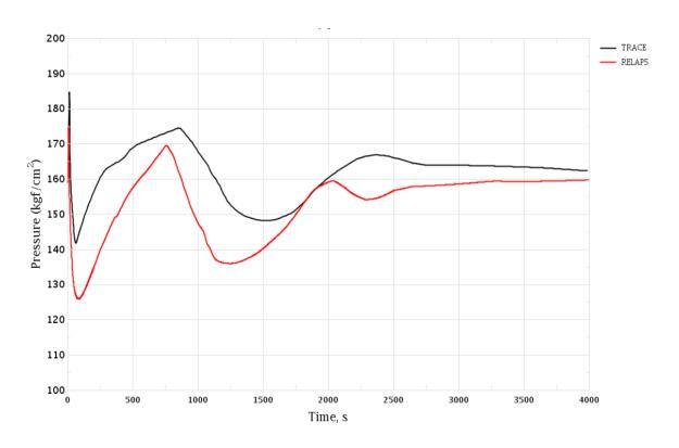
Figure 3-39 Loss of Turbine Condenser Vacuum. RCS Pressure
