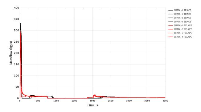
Figure 3-68 Loss of Turbine Condenser Vacuum. BRU-A Steam Mass Flow Rate
