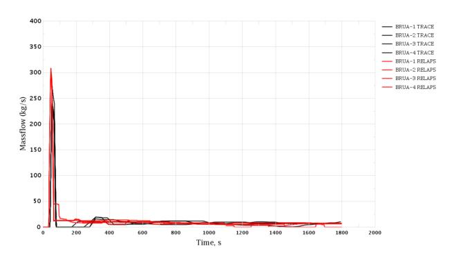
Figure 3-138 Uncontrolled Withdrawal of CR Group. BRU-A Steam Mass Flow Rate
