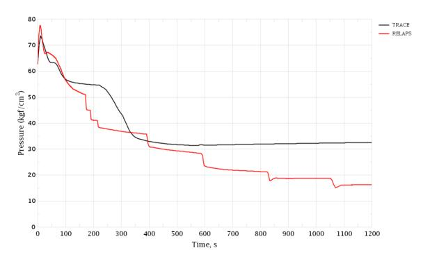
Figure 3-161 PRZ Surge Line Break. SG-2 Pressure
