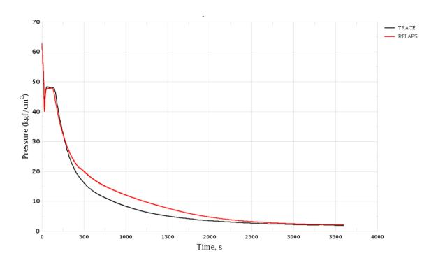
Figure 3-21 MSH Break. SG-3 Pressure
