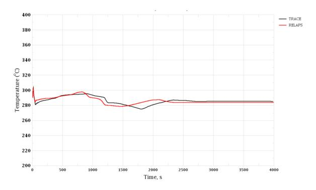
Figure 3-46 Loss of Turbine Condenser Vacuum. Coolant Temperature in Cold Leg, Loop 2
