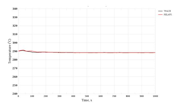
Figure 3-82 Trip of One RCP. Coolant Temperature in Cold Leg, Loop 2
