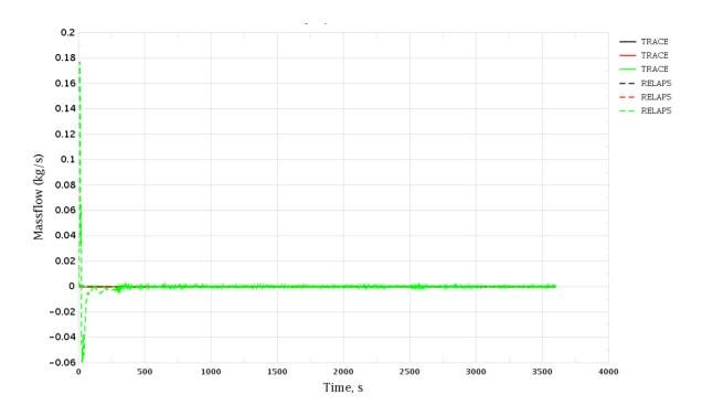
Figure 3-17 MSH Break. PRZ Spray Mass Flow Rate
