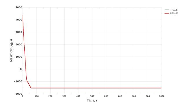
Figure 3-85 Trip of One RCP. RCS Loop 1 Mass Flow Rate
