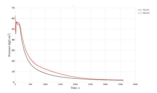
Figure 3-20 MSH Break. SG-2 Pressure
