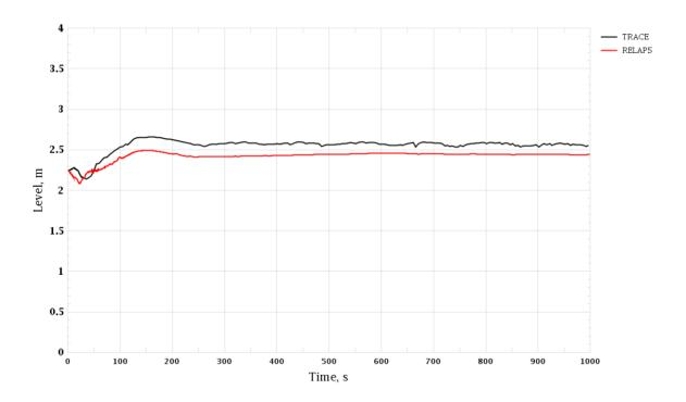
Figure 3-97 Trip of One RCP. SG-1 Level (Wide Range)
