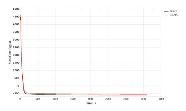
Figure 3-15 MSH Break. RCS Loop 4 Mass Flow Rate
