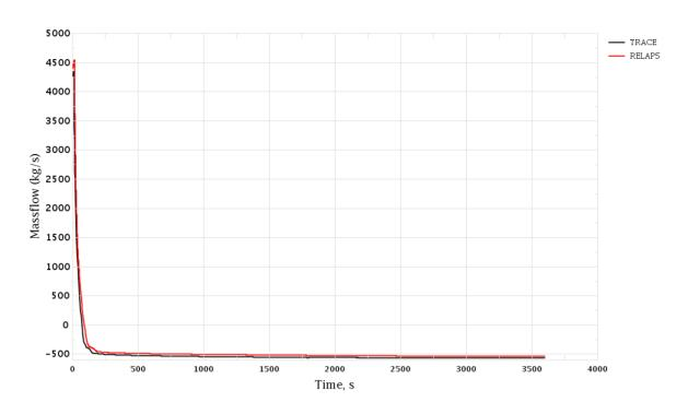
Figure 3-13 MSH Break. RCS Loop 2 Mass Flow Rate
