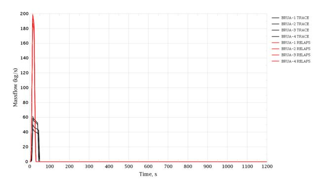
Figure 3-169 PRZ Surge Line Break. BRU-A Steam Mass Flow Rate
