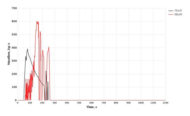
Figure 3-177 PRZ Surge Line Break. HA-1 Mass Flow Rate
