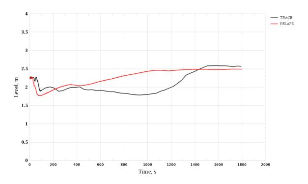
Figure 3-135 Uncontrolled Withdrawal of CR Group. SG-4 Level (Wide Range)
