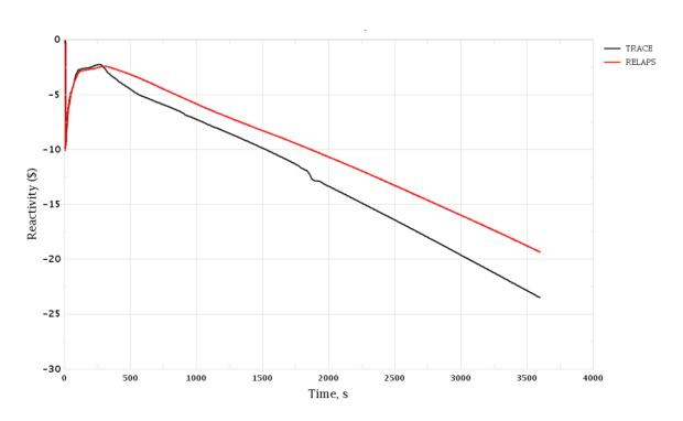
Figure 3-18 MSH Break. Core Reactivity
