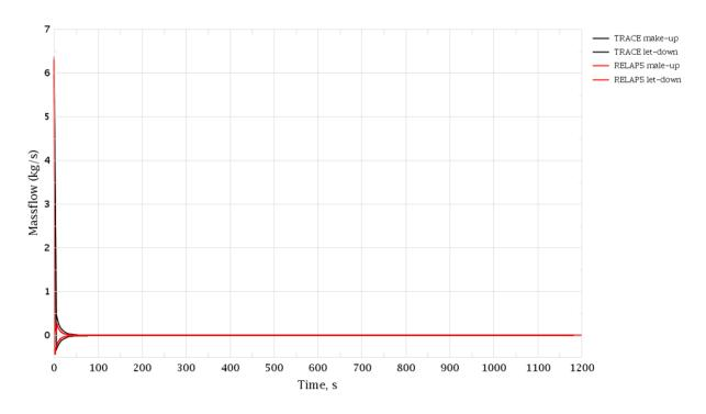
Figure 3-157 PRZ Surge Line Break. Make-Up and Let-Down Mass Flow
