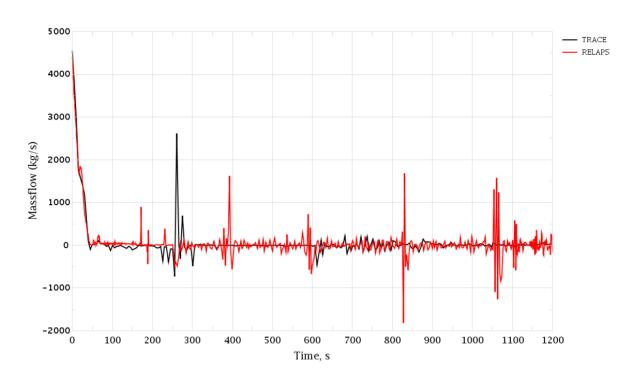
Figure 3-154 PRZ Surge Line Break. RCS Loop 2 Mass Flow Rate
