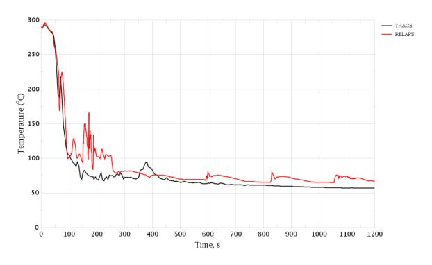
Figure 3-151 PRZ Surge Line Break. Coolant Temperature in Cold Leg, Loop 3
