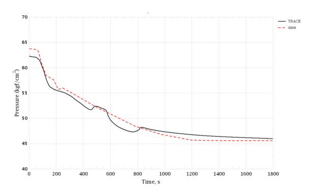
Figure 3-195 Inadvertent Opening of SG SRV in Hot Shutdown. SG-4 Pressure
