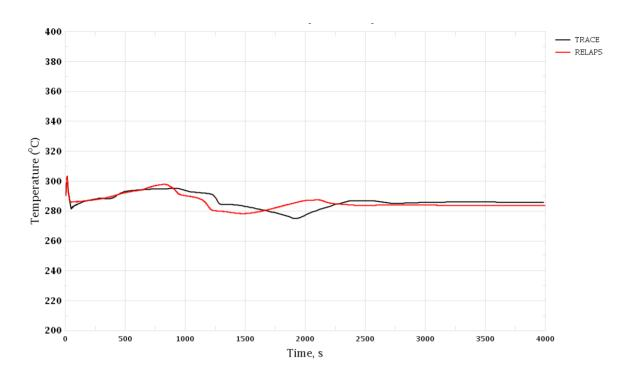
Figure 3-45 Loss of Turbine Condenser Vacuum. Coolant Temperature in Cold Leg, Loop 1
