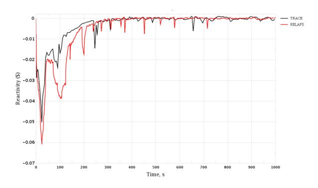
Figure 3-92 Trip of One RCP. Core Reactivity
