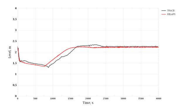
Figure 3-64 Loss of Turbine Condenser Vacuum. SG-4 Level (Wide Range)
