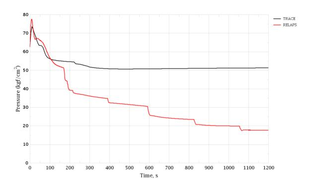
Figure 3-162 PRZ Surge Line Break. SG-3 Pressure
