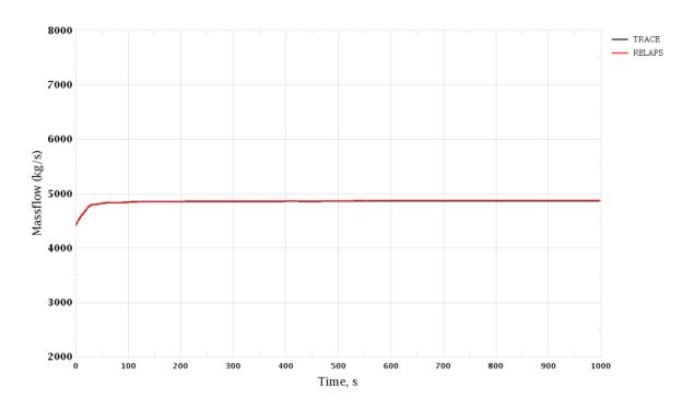
Figure 3-87 Trip of One RCP. RCS Loop 3 Mass Flow Rate
