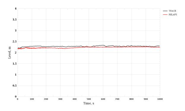
Figure 3-99 Trip of One RCP. SG-3 Level (Wide Range)
