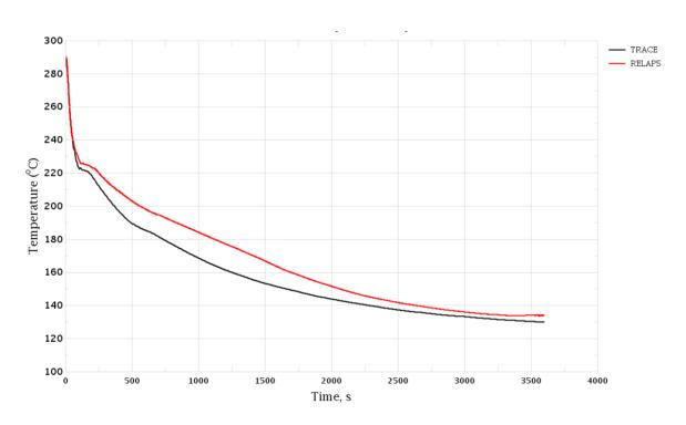
Figure 3-8 MSH Break. Coolant Temperature in Cold Leg, Loop 1
