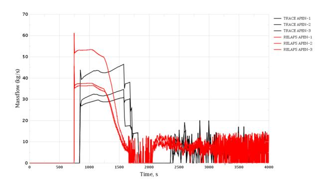
Figure 3-72 Loss of Turbine Condenser Vacuum. EFW Pumps Mass Flow Rate
