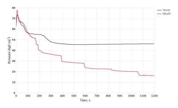
Figure 3-160 PRZ Surge Line Break. SG-1 Pressure
