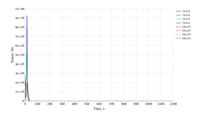
Figure 3-158 PRZ Surge Line Break. PRZ Heaters Power
