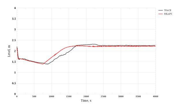
Figure 3-63 Loss of Turbine Condenser Vacuum. SG-3 Level (Wide Range)
