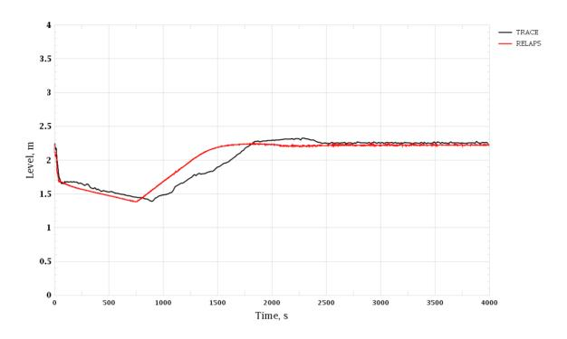
Figure 3-61 Loss of Turbine Condenser Vacuum. SG-1 Level (Wide Range)
