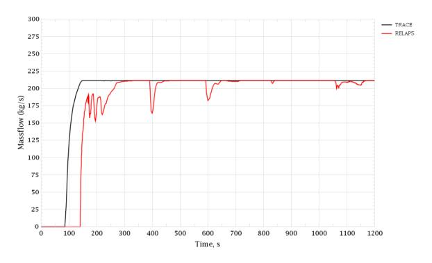
Figure 3-174 PRZ Surge Line Break. LPIS-1 Mass Flow Rate
