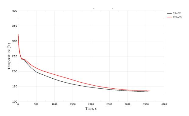
Figure 3-4 MSH Break. Coolant Temperature in Hot Leg, Loop 1
