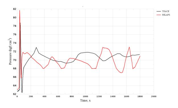
Figure 3-130 Uncontrolled Withdrawal of CR Group. SG-3 Pressure
