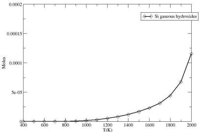
Regarding the hydroxide production, the calculation shows that the related gases begin to be released at rather high temperature. They are expected to modify the chemistry in the primary circuit, in particular the Cs one by potentially forming silicates.
