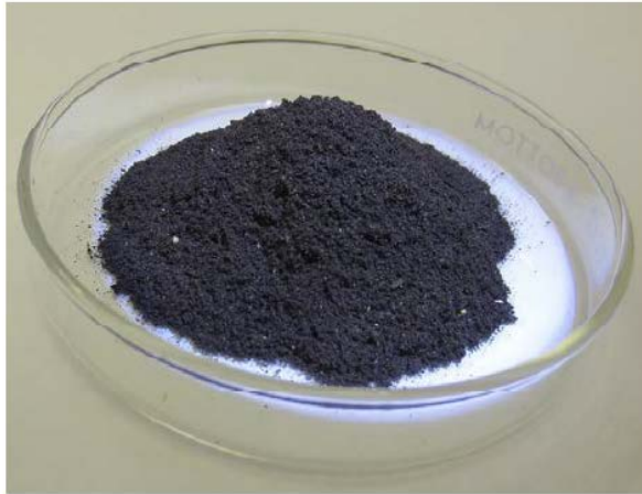
Figure 92: Rust collected from bottom of scaled air-based RCCS test facility over 100-day period [58]
