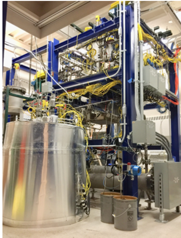
Figure 33. The experimental flow loop at the University of Michigan will be used to demonstrate the SAFARI digital twin model on a molten-salt demonstration loop [7].
