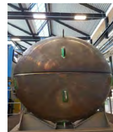
Mockup EB weld of lower head
