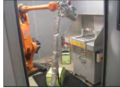
Robot for pre-programmed movement of spray gun
