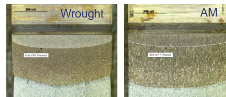
Heat tint more difficult to see in AM material
