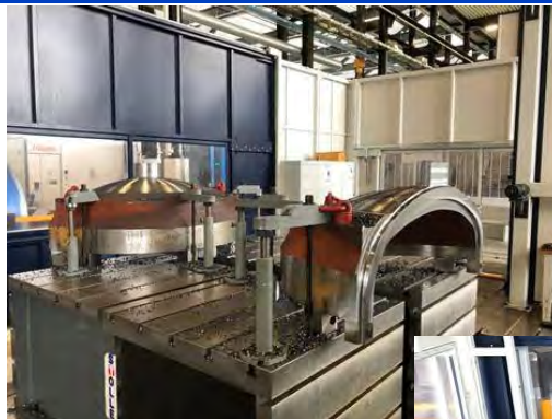
Each One-half Lower Reactor Head ~6500lbs (2950 kg) x 70 inches @ 2/3rds scale
