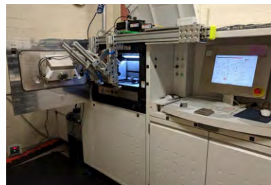
EOSM270 LPBF Thermography System www.nist.gov/el/lpbf-thermography
