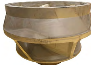
NNS Reactor Coolant Pump Impeller (courtesy Framatome and Albert & Duval)
