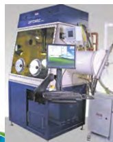
Optomec LENS MR-7 w/ melt pool monitoring (Stratronics)
