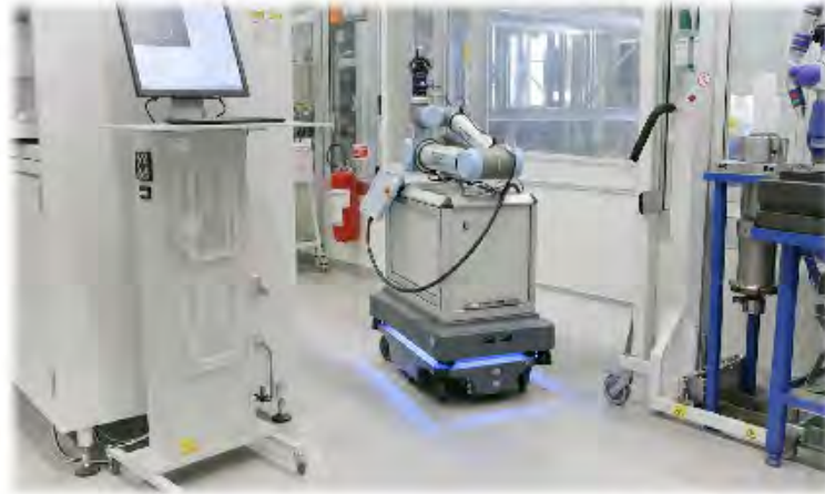
Collaborative robots for cleaning of machines chamber
