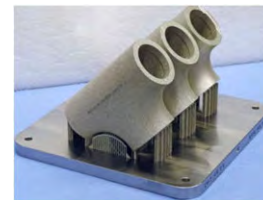
Sacrificial Supports Courtesy of Rolls-Royce
