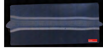
110mm (thick) EB Weld
