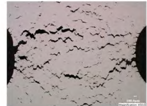
Creep cavitation (INL)
