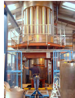
40" diameter HIP Vessel Courtesy: Isostatic Forge International
