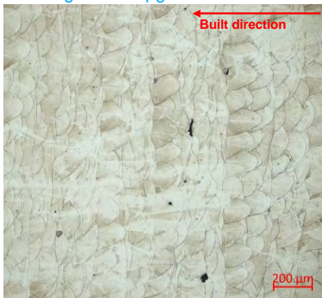
Before gas flow upgrade
