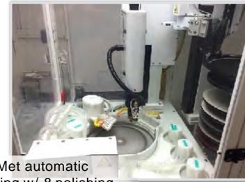
Controlled material removal from 0.2 - 10 micron using well developed material preparation techniques.
