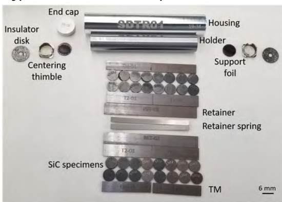
Typical HFIR irradiation capsule for ceramics
