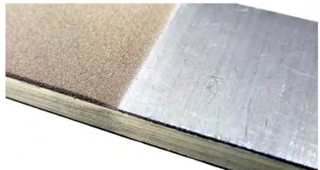
High-pressure cold spray coating of commercially pure nickel sprayed (left side) at PNNL
