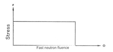
Figure A-12 Stress under irradiation as step-function loading (Shibata et al., 2010, Explanatory Figure 2.3.2(b))
