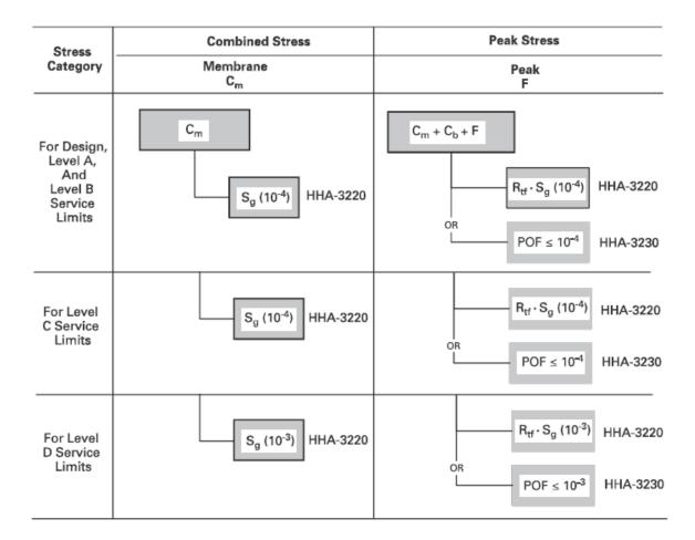
Figure A-9 Design-allowable stresses for SRC-1 GCCs (HHA-3221-1)
