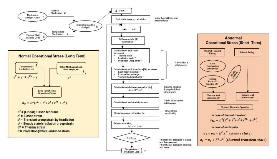
Figure A-14 General flowchart for stress calculation in a graphite component in a graphite-moderated reactor (Shibata et al., 2010, Explanatory Figure 2.2.3(a))
