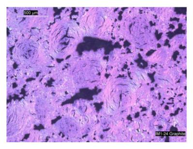
Figure A-20 Microstructure of IM1-24 graphite (Burchell, 2010, p. 21)
