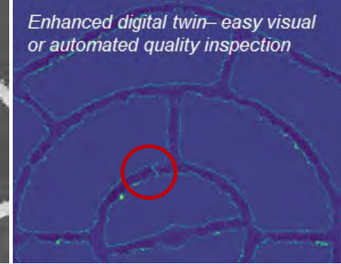
Build 26: based on improved AM technique, no pores in junctions
