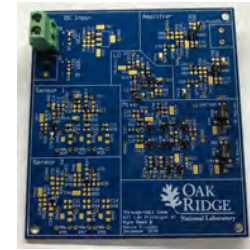
>2Mrad JFET-based Sensor Interface Electronics (DOE NEET)
