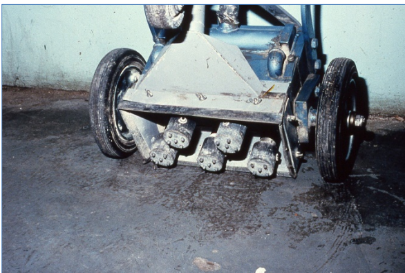
Underside of a typical hand-pushed scabbling machine with vacuum used to roughen concrete surfaces and remove contamination in the surface coatings or embedded deep into the concrete surface.
