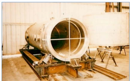
Left: Model 125-B rail shipping cask under fabrication showing internal structure without inner containment shell. Right: Outer containment shell. (481.14)
