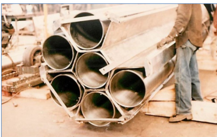
Left: Model 125-B rail shipping cask under fabrication showing internal structure without inner containment shell. Right: Outer containment shell. (481.14)
