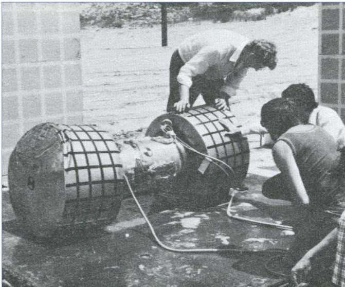
Model 125-B rail shipping cask 1/4-scale model following a drop test. (481.14)
