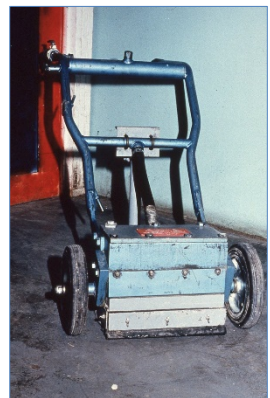
Underside of a typical hand-pushed scabbling machine with vacuum used to roughen concrete surfaces and remove contamination in the surface coatings or embedded deep into the concrete surface.
