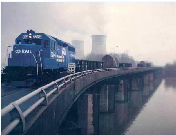
Rail shipment of three Model 125 B shipping casks containing defueling canisters. (481.14)
