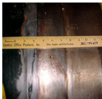
V.C. Summer (Fall 2000): Cracking in a hot leg nozzle pipe weld
