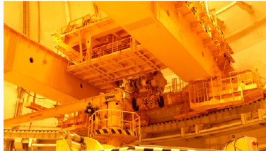
Polar crane in reactor hall as tool for measurement of core shroud dimension
