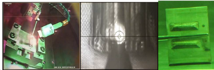
Laser welding of irradiated 304L
