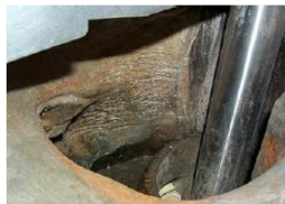
V.C. Summer (Fall 2000): Cracking in a hot leg nozzle pipe weld
