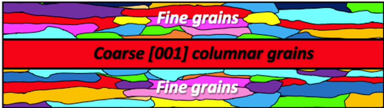
Figure 2.4. Schematic of functionally fabricated SLM Inconel 718 using variable processing parameters.
