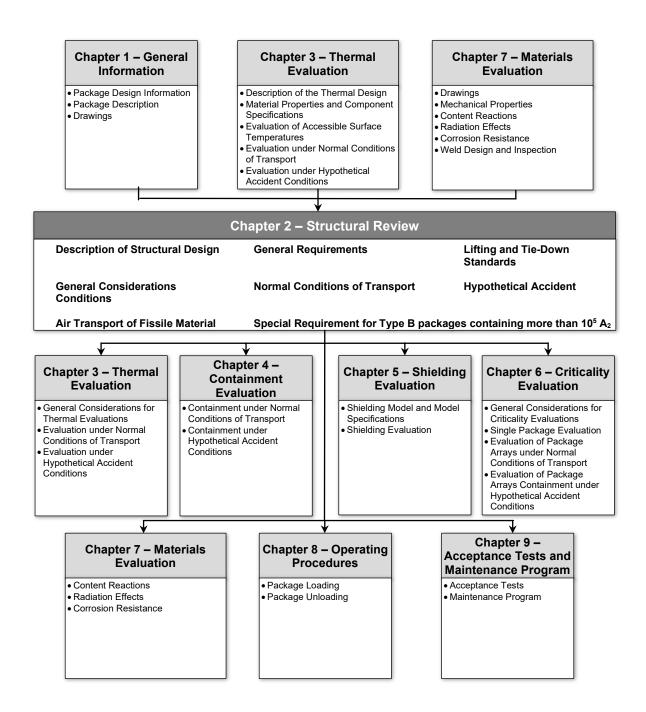
Figure 2-1 Information Flow for the Structural Evaluation
