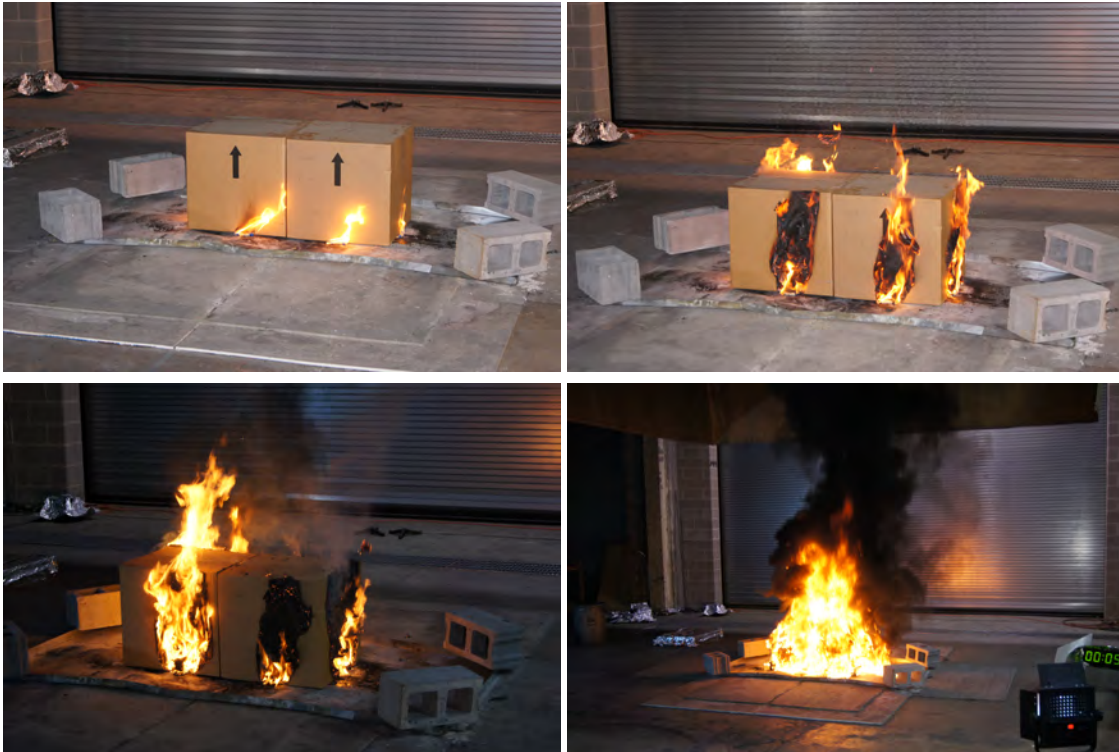
Figure 28: Heat release rate and photographs of Test 26.
