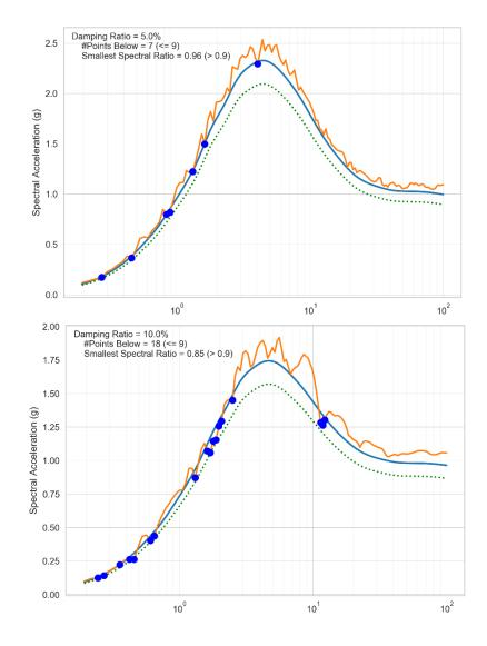
Figure 5-8 Multiple DRS governing at different frequencies (Approach 1 criteria with a log-power frequency series) (smooth curves showing the criteria)
