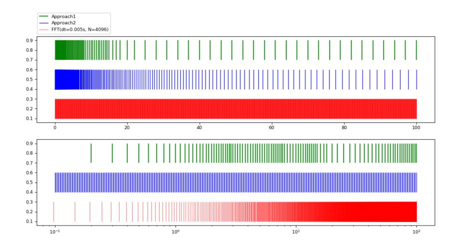
Figure 5-1 A comparison of frequencies for Approach 1, Approach 2, and the FFT for a typical time history
