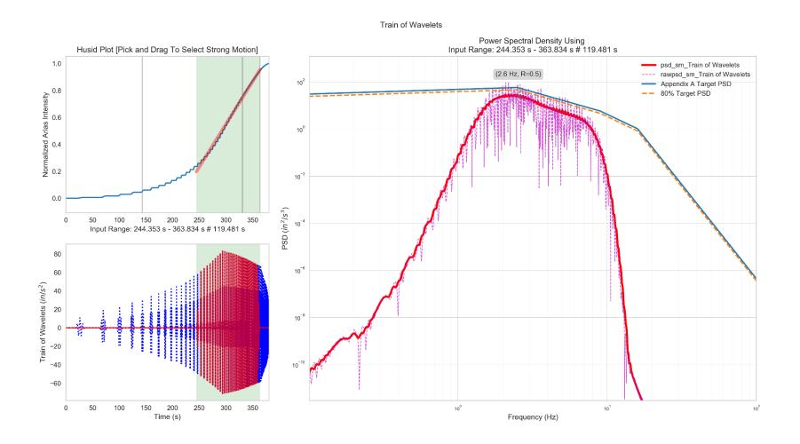
Figure 2-2 PSD check of the train of wavelets (±5 percent window)
