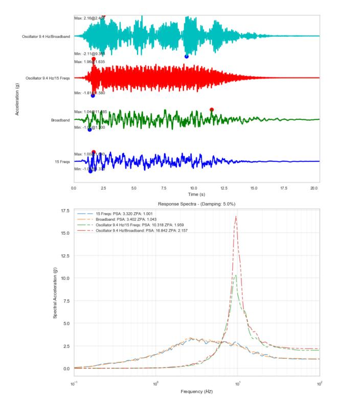
Figure 2-29 Relative responses of the 9.4-Hz SDOF structure
