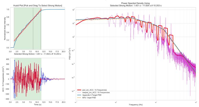
Figure 2-9 PSD check of the accelerogram with 15 major frequencies (±10-percent window)
