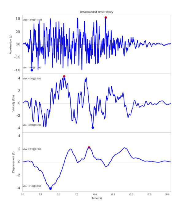
Figure 2-26 The acceleration, velocity, and displacement of the broadband accelerogram
