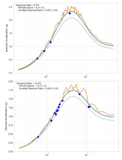
Figure 5-6 Multiple DRS governing at different frequencies (Approach 1 criteria) (smooth curves showing the criteria)
