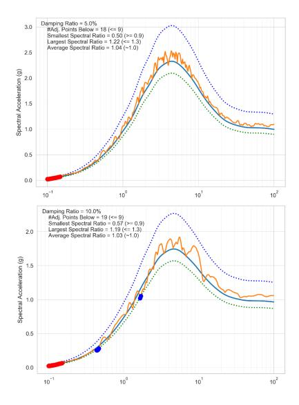
Figure 5-7 Multiple DRS governing at different frequencies (Approach 2 criteria) (smooth curves showing the criteria)
