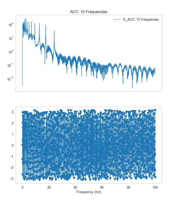
Figure 2-6 Fourier spectra with the frequency in linear scale
