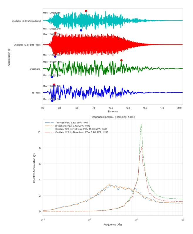
Figure 2-30 Relative responses of the 12.8-Hz SDOF structure
