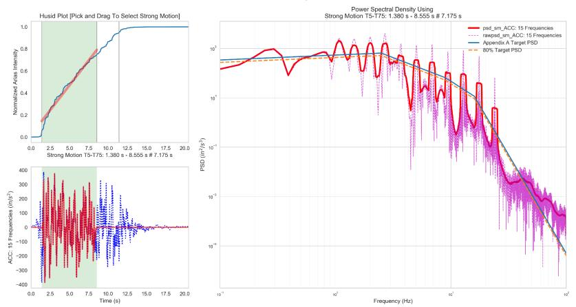
Figure 2-10 PSD check of the accelerogram with 15 major frequencies (±5-percent window)
