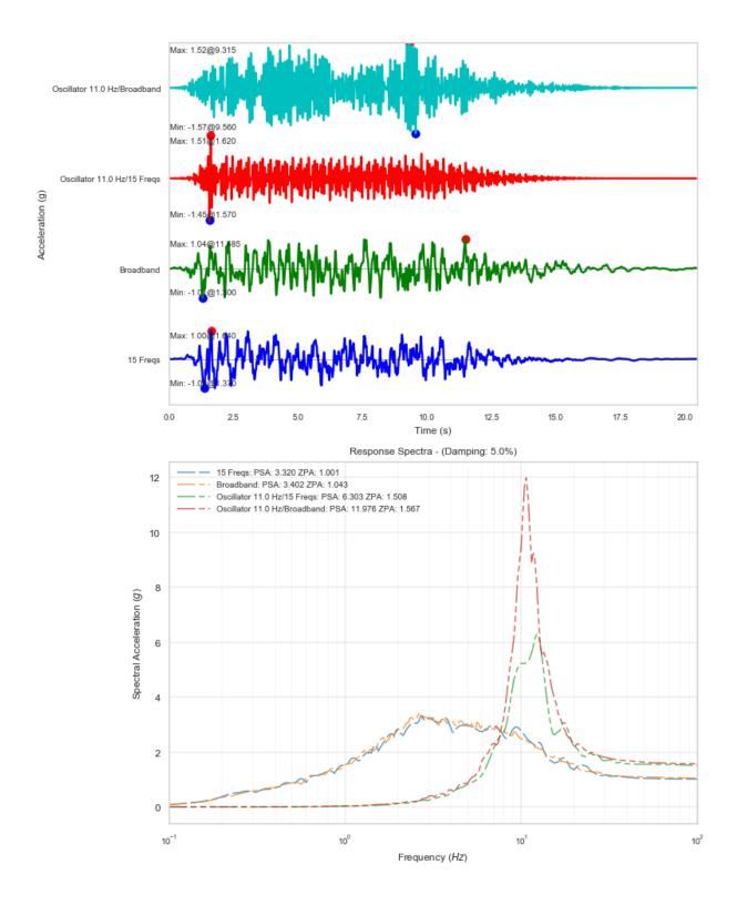
Figure 2-28 Relative responses of the 11.0-Hz SDOF structure
