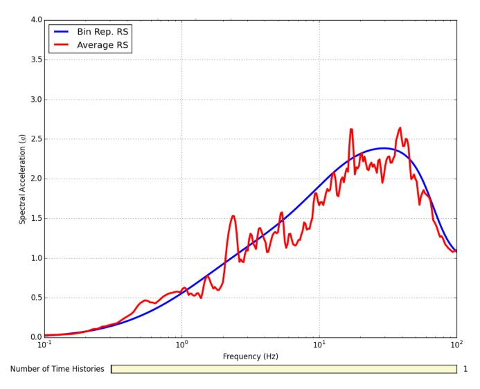
Figure 2-15 The RS of a time history generated from the target PSD function
