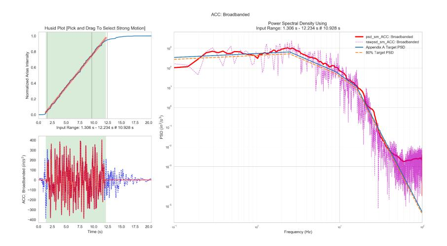
Figure 2-27 A PSD check of the broadband accelerogram
