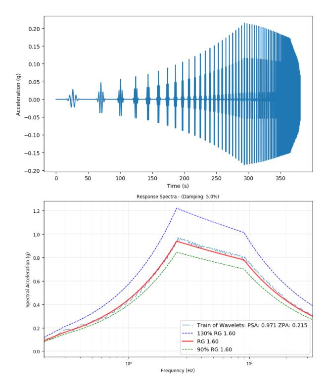
Figure 2-1 Illustration of a train of wavelets that matches well with the RG 1.60 DRS
