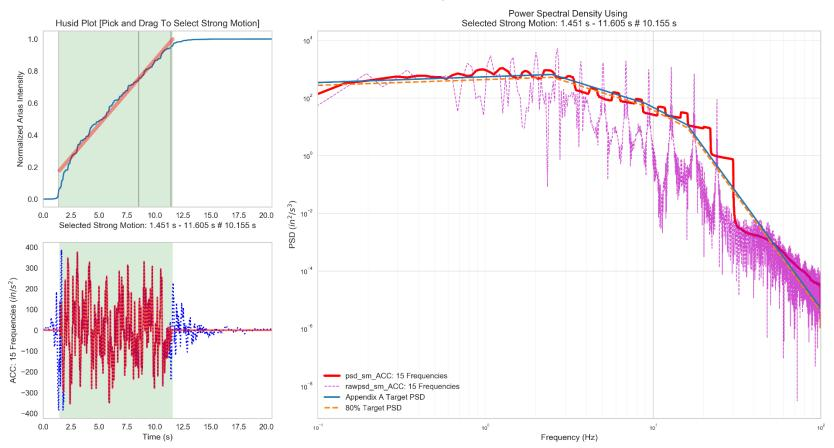
Figure 2-8 PSD check of the accelerogram with 15 major frequencies (±20-percent window)
