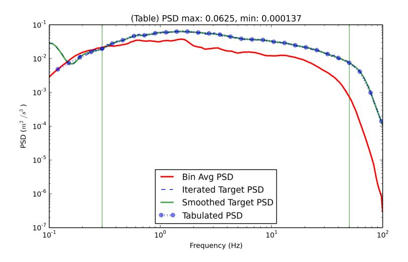
Figure 2-14 A target PSD function (dotted)
