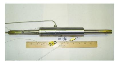
Figure 7-27 Specimen 01-3/4 in the As-received Condition
