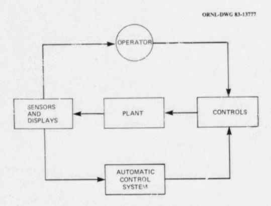
Fig. 2.8. A symmetrical man/machine model.
