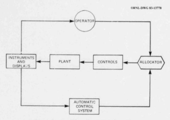
Fig. 2.9. An "allocated" man/machine model.
