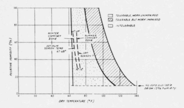
Fig. A-4. Temperature-humidity tolerability (with conventional clothing) (from Woodson, 1981).
