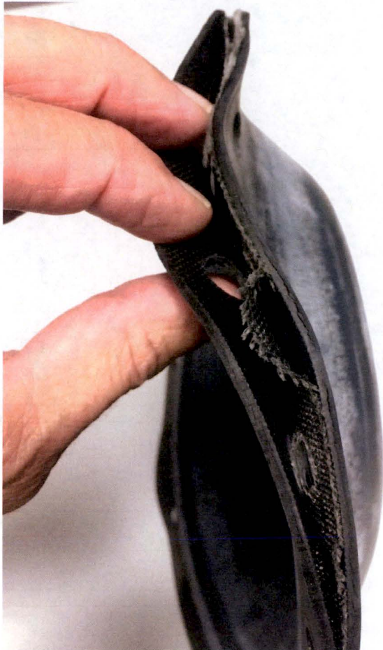
Figure 2: Delamination of fabric from elastomer
