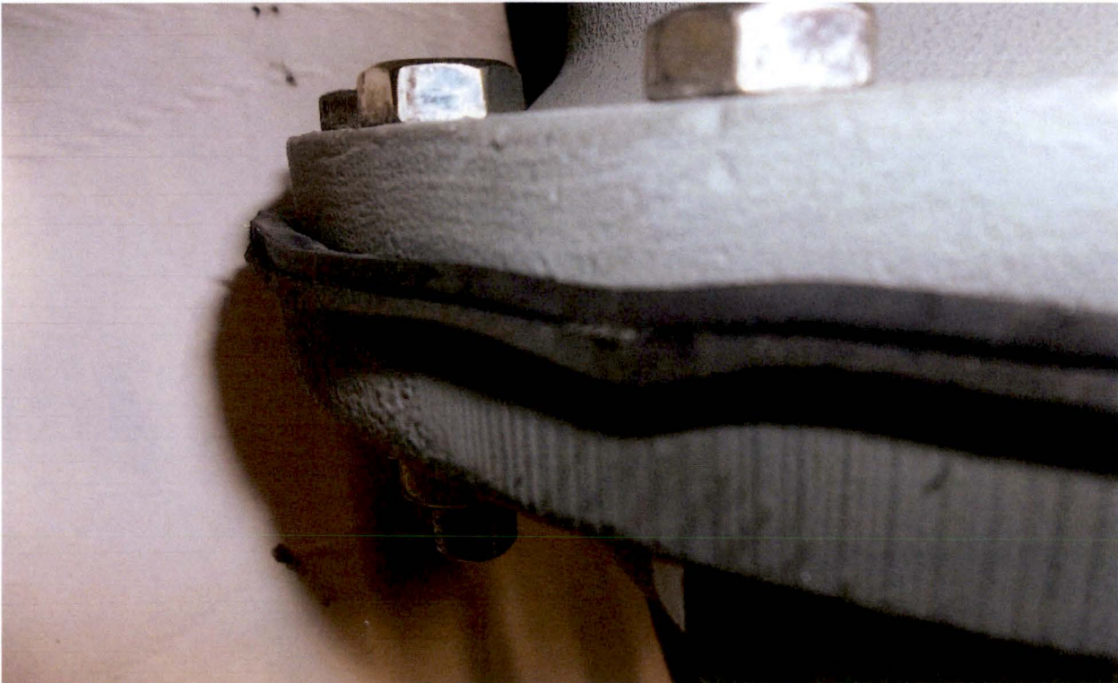
Figure 10: Diaphragm with 300 in-lb applied torque – Distorted, edge not square
