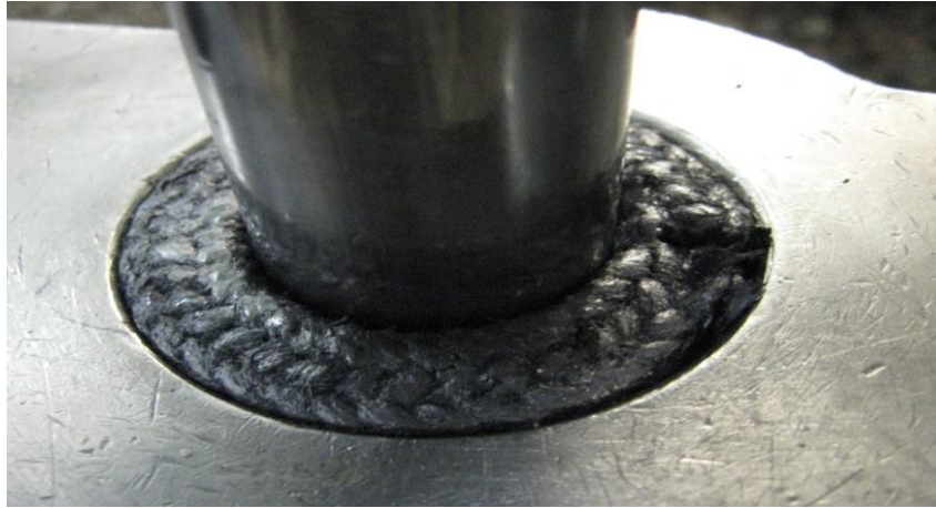
Figure 7. Braided Carbon/Graphite Ring in the Test Fixture Packing Box (Source: Author)
