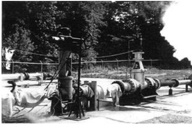
Figure 1: An extensive matrix of flow-loop tests, including multiple blowdowns and thermal-binding scenarios, was performed to qualify the innovative gate valve design.
