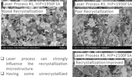
grains is unavoidable in AM parts even after high temperature annealing.
