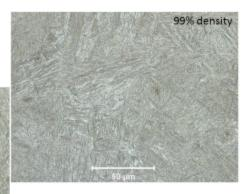
Pores represent residual gases trapped in the powder during manufacture
