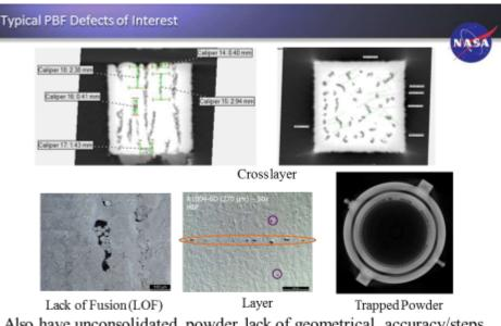
Also have unconsolidated powder, lack of geometrical accuracy/steps in the part, reduced mechanical properties, inclusions, gas porosity, voids, and poor or rough surface finish 20
