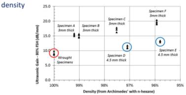
A clear upward trend of increasing gain with decrease in density for similarly-sized specimens
