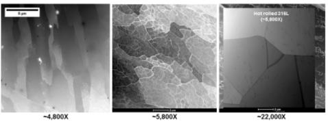
HAADF STEM of columnar grains containing subgrains ADF STEM of dislocation networks within grains
