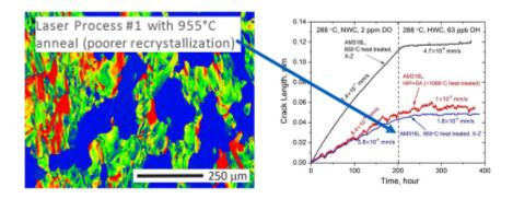
After high temperature annealing (above stress relief), retained unrecrystallized grains in the material may not significantly affect SCC behavior.
