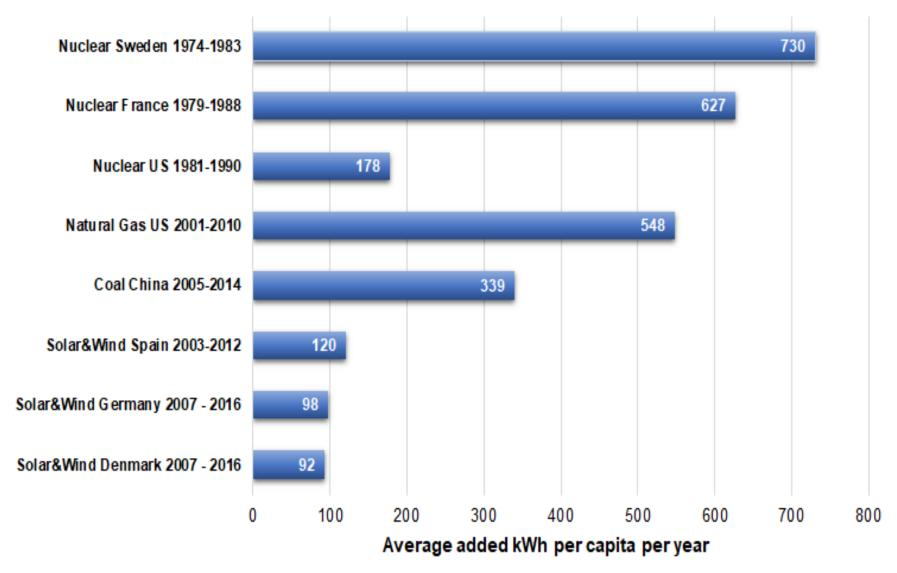
Nuclear electricity can be deployed as quickly as coal or gas at a time of need
