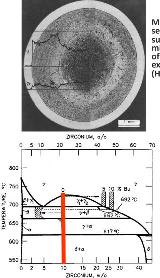
Metallographic cross section with superimposed radial microprobe scans at top of U-10Zr pin DP-81, experiment X447 (Hofman, et al., 1995)
