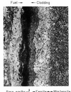
Rare earths — Ferrite — Martensite Optical, Etched, 500× Fuel — Cladding
