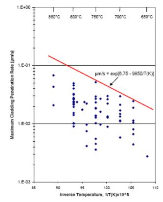
Effective cladding penetration rates from FBTA tests for speciments tested for 1.0 hour (Tsai, et al., 2007)
