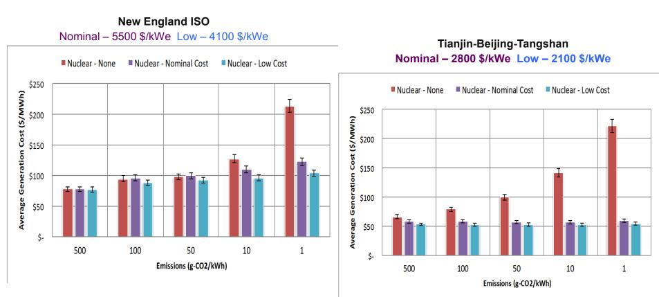
Simulation of optimal generation mix in power markets MIT tool: hourly electricity demand + hourly weather patterns + capital, O&M and fuel costs of power plants, backup and storage + ramp up rates
