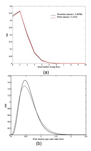
Figure C-11 Prior and posterior flaw density (a) and intensity (b) for large size flaw
