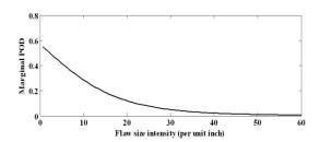
Figure C-10 Marginal POD independent of small flaw depth
