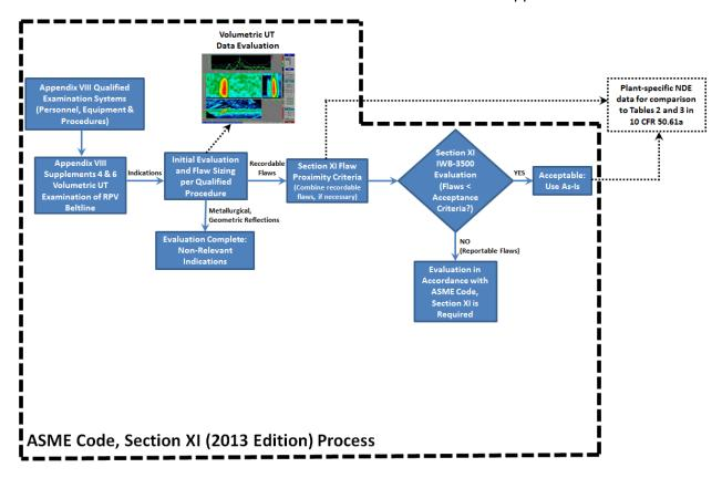
Figure 6-2 ASME Code, Section XI, examination and flaw evaluation process and identification of flaws for comparison to the Alternate PTS Rule
