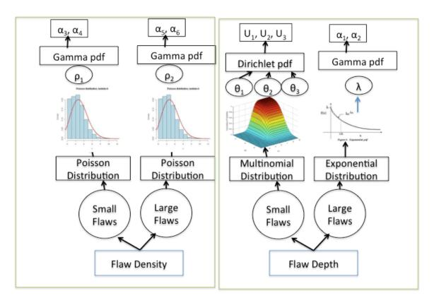
Figure D-2 Flaw-Depth and Flaw-Density Distributions Used in VFLAW and Their Corresponding Parameter Hyper-PDFs
