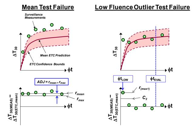
Figure 5-3 Specific procedures to account for failure of the mean test (left) or low-fluence outlier statistical test (right)
