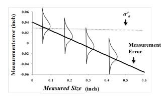
Figure C-6 Measurement error vs. flaw depth
