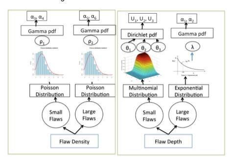
Figure C-4 Flaw depth and flaw density distributions used in VFLAW and their corresponding parameter hyper PDFs
