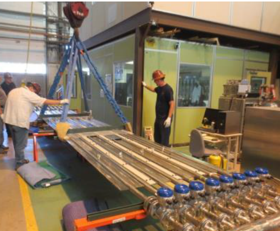
Assembled panel staged for 180° flip
