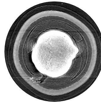
X-ray tomogram of irradiated AGR-1 particle showing fission product attack of the SiC layer
