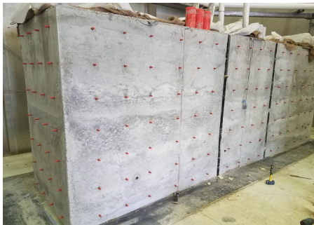
Figure 12.4 ASR concrete block sample.
