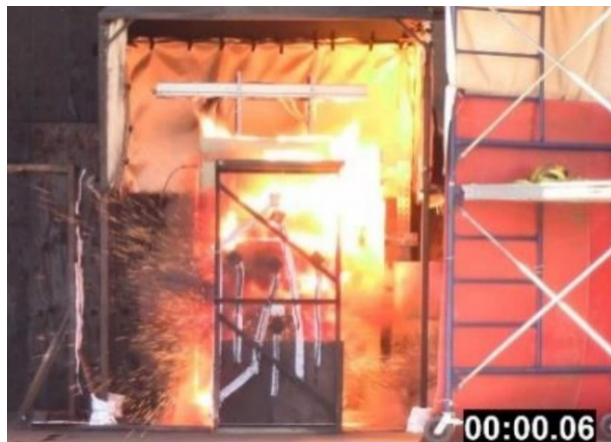
Figure 9.6 High Energy Arc Fault Testing of Electrical Components.
