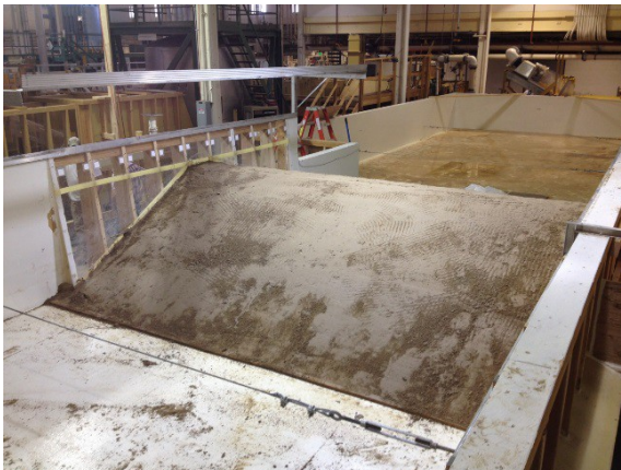
Figure 10.10 Dam breach test facility at Reclamation.
