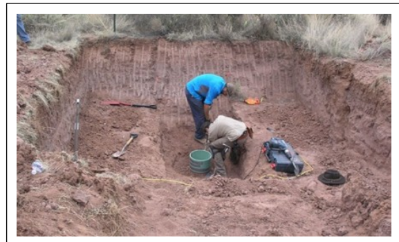
Figure 5.15 Test Pit at the Bluewater Site.
