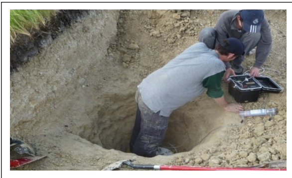
Figure 5.14 Radon flux measurement at Falls City.
