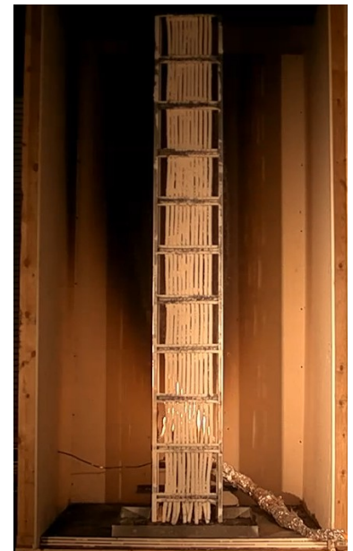
Figure 9.7 IEEE-383/1202 modified test with single cable layer tray coated with fire retardant coating.
