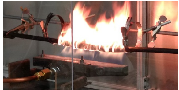
Figure 9.4 Horizontal electrical cable circuit integrity test.
