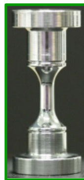
Figure 11.6 PWSCC initiation testing rig and 1.2-inch-tall specimen developed by PNNL.
