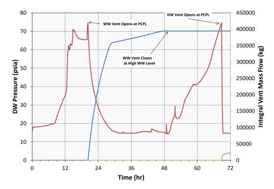
Figure 3-54 Mark II containment pressure and vent flow for Case 11
