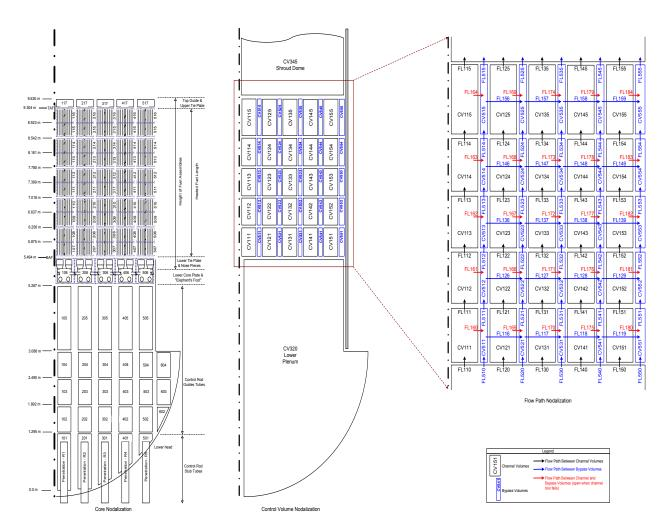
Figure 3-3 MELCOR core nodalization for Mark I analysis
