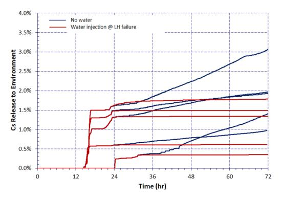
Figure 3-37 Effect of water injection on selected cesium releases for selected cases
