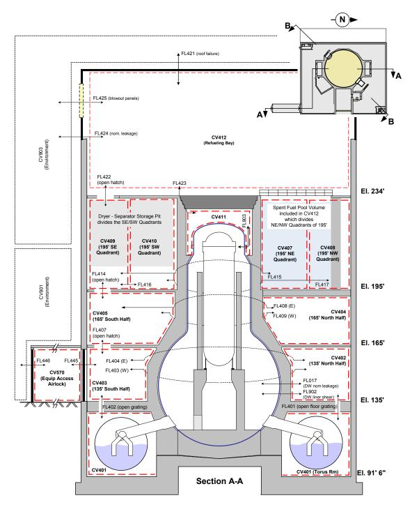
A sectional view of the reactor building is shown in Figure 3-6. It is modeled on a level-by-level basis, beginning in the basement (i.e., torus room) and sequentially rising up through the main floors to the refueling bay.
