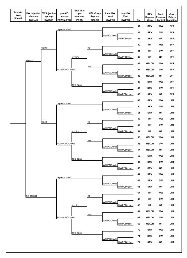
Figure C-4 APET for DW Injection and WWF Venting Strategies (APET 3), Sheet 2, Sequences 37 to 72
