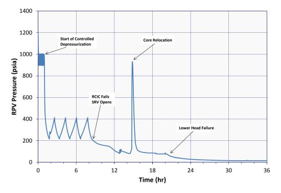
Figure 3-48 Mark II RPV pressure for Case 11
