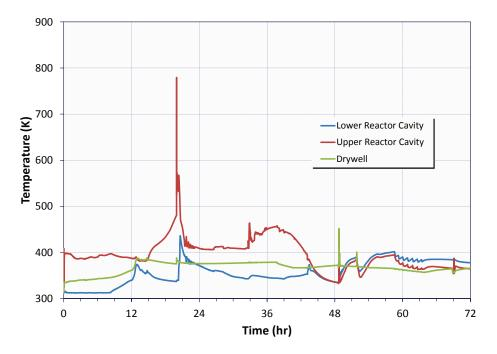
Figure 3-57 Mark II containment atmosphere temperatures for Case 11
