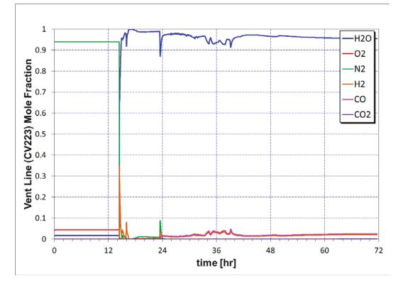
Figure 3-43 Mark I wetwell vent line gas distribution for Case 9
