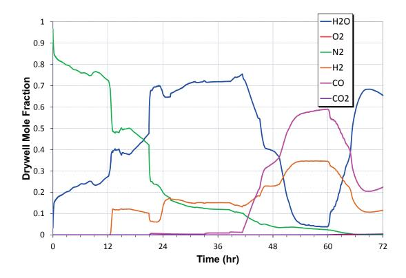
Figure 3-73 Mark II drywell gas distribution for Case 11p1
