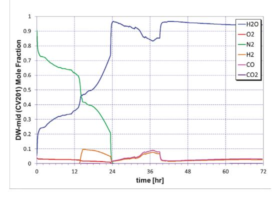
Figure 3-41 Mark I drywell gas distribution for Case 9
