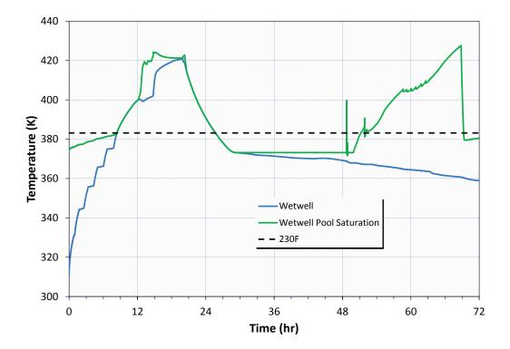
Figure 3-55 Mark II suppression pool temperature for Case 11
