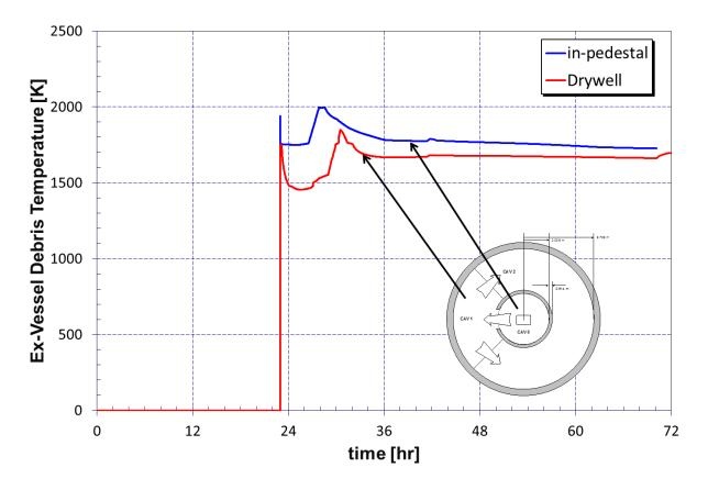
Figure 3-30 Mark I ex-vessel debris temperature for Case 1
