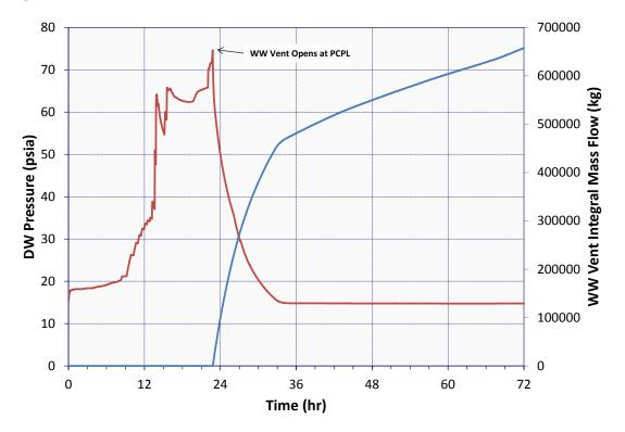
Figure 3-65 Mark II containment pressure and vent flow for Case 1
