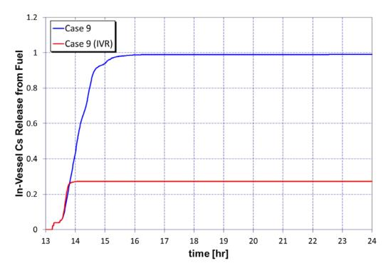
Figure 3-46 Mark I cesium release fraction from fuel for Case 9 (IVR)
