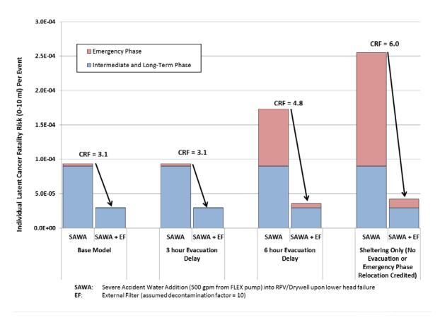
Figure 4-20 CRF for conditional ILCF risk (0-10 mi) for evacuation sensitivity calculations for BWR Mark I MELCOR Case 49
