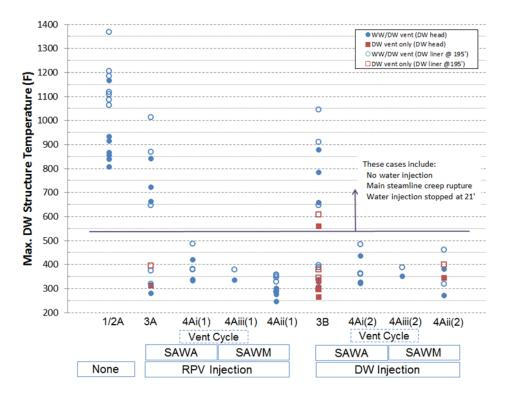
Figure 3-38 Mark I containment gas and structure temperatures
