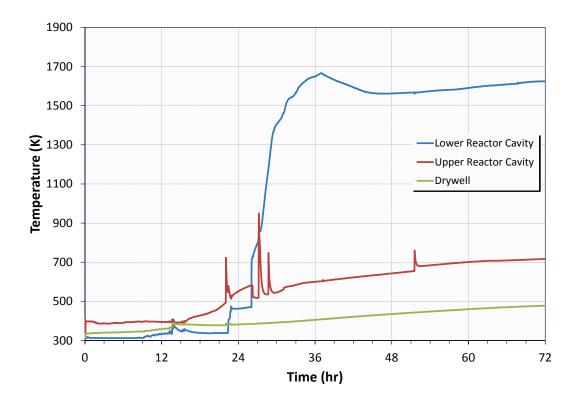
Figure 3-66 Mark II containment atmosphere temperatures for Case 1
