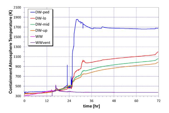
Figure 3-33 Mark I containment atmosphere temperature for Case 1
