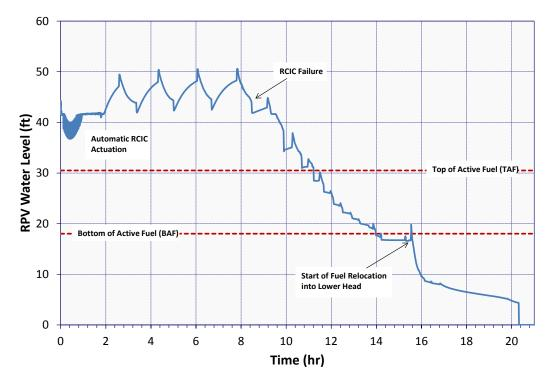
Figure 3-61 Mark II RPV water level for Case 1
