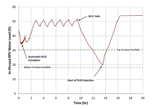
Figure 3-45 Mark I RPV water level for Case 9 (IVR)
