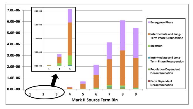
Figure 4-11 Mark II source terms – population dose per event (person-rem) with breakdown by accident phase and exposure pathway (0-50 miles)
