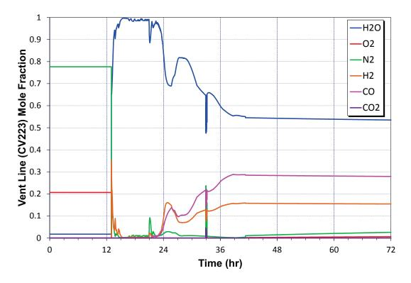
Figure 3-75 Mark II wetwell vent gas distribution for Case 11p1
