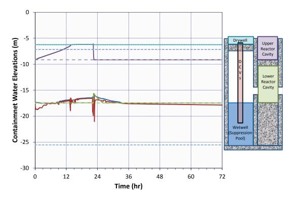
Figure 3-67 Mark II containment water levels for Case 1
