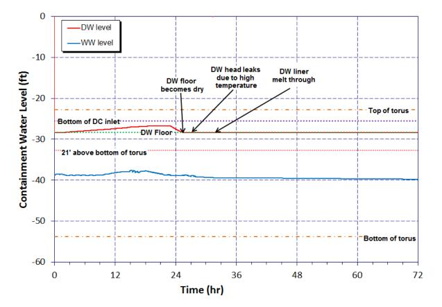
Figure 3-29 Mark I containment water level for Case 1
