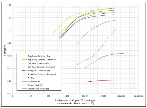
Figure 1 Spherical, Homogeneous Mixtures of <sup>235</sup>U and Various Nonfissile Materials (30-cm Thick Water Reflection)
