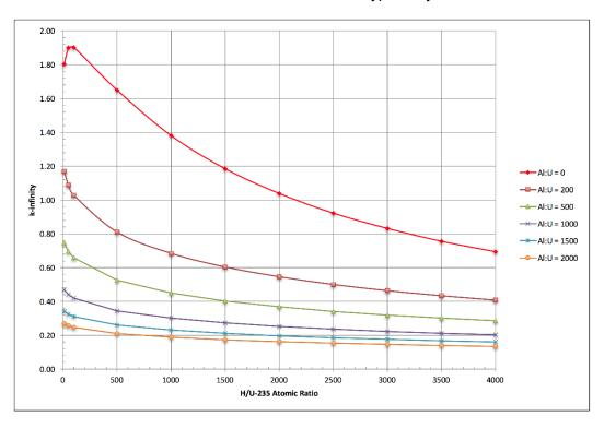
Figure 2 Infinite Homogeneous Mixture of <sup>235</sup>U Metal and Water with Aluminum Present as a Diluent
