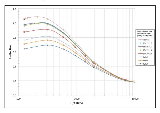
Figure 5 Arrays of U(0.995)-Metal Units Immersed in Water
