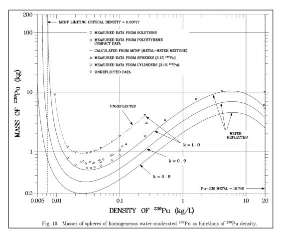
Figure 8 Masses of Spheres of Homogeneous Water-Moderated <sup>239</sup>Pu as Functions of <sup>239</sup>Pu Density (Ref. 22, Fig. 10)
