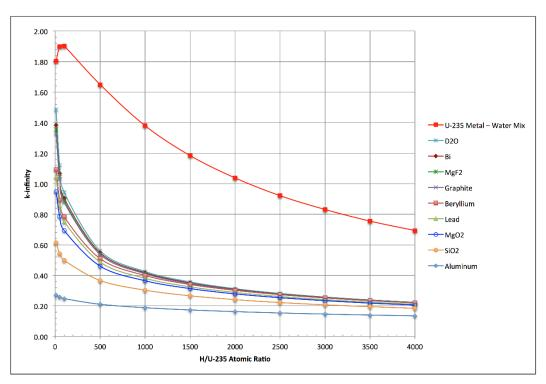
Figure 3 Infinite Homogeneous Mixture of <sup>235</sup>U Metal and Water with a Diluent-to-<sup>235</sup>U Ratio of 2000
