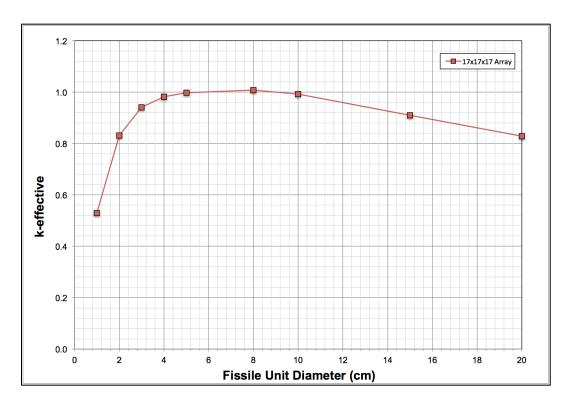
Figure 6 17 × 17 × 17 Array of U(0.995)-Metal Units Immersed in Water
