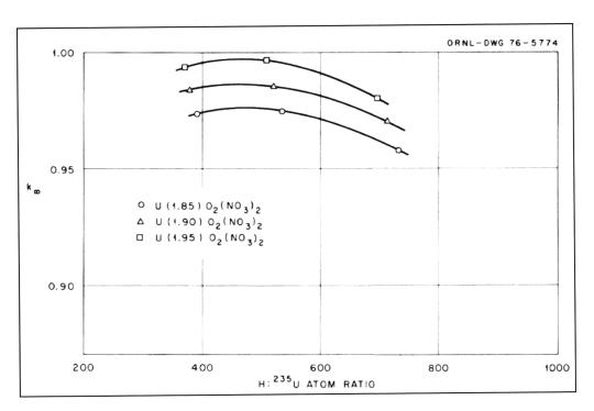
Figure 7  $k_{inf}$  Calculated for  $UO_2(NO_3)_2$ - $H_2O$  Mixtures (Ref. 24, Fig. 2)
