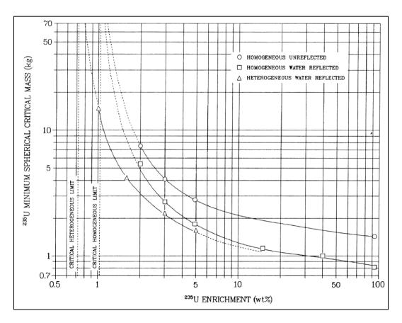
Figure 4 Minimum Spherical Critical Masses as Functions of <sup>235</sup>U Enrichment in Homogeneous and Heterogeneous Hydrogen-Moderated Systems (Ref. 21, Fig. 22)
